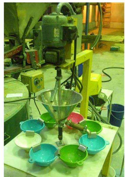
**Figure 4.1: Rotary pulp splitter.**
