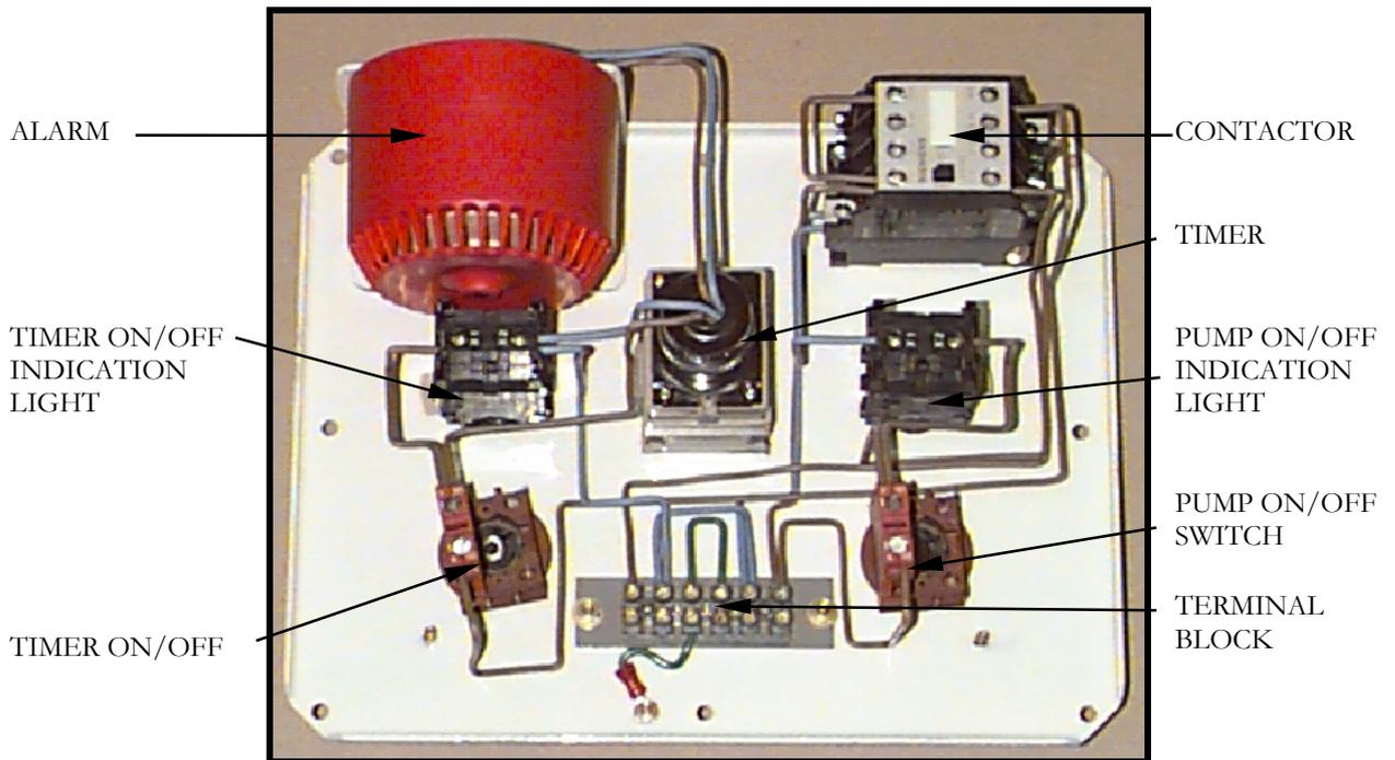
**Figure 15 - Control Panel, Wiring Diagram (Model M12)**
