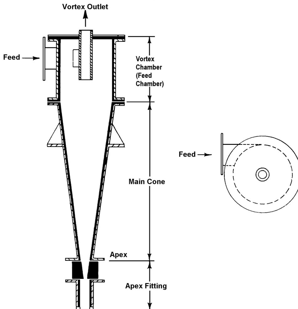
For operation, a suspension of solid particles in a liquid is introduced under pressure through the feed opening. The tangential entry induces the liquid to spin within the cyclone and the design of the apparatus results in a portion of the liquid, together with the faster-settling particles, being discharged through the apex opening. The remainder of the liquid, together with the slower settling particles, is discharged through the vortex outlet.
