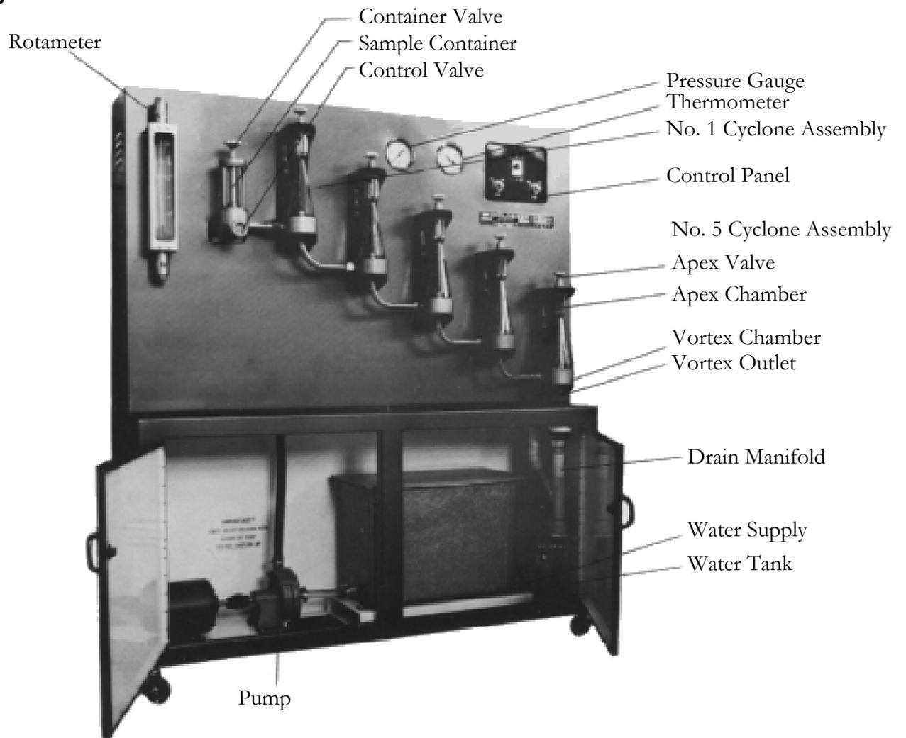
**Figure 6 - Diagrammatic Arrangement**
