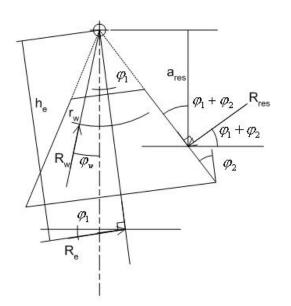
Mechanical model of spiderless cone crusher
