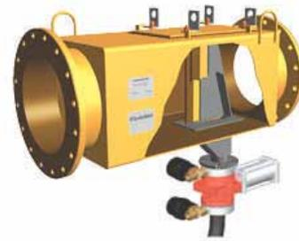
A LSA vertical cutter sampler with an optional VSA automatic flushing valve set for process flows at ambient pressure. A cyclone overflow is a typical LSA sampling point.
