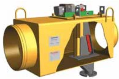
NLA non plug vertical cutter sampler with automatic mechanical cutter cleaner for ambient pressure process flow containing trash. Victaulic process pipe connections.
