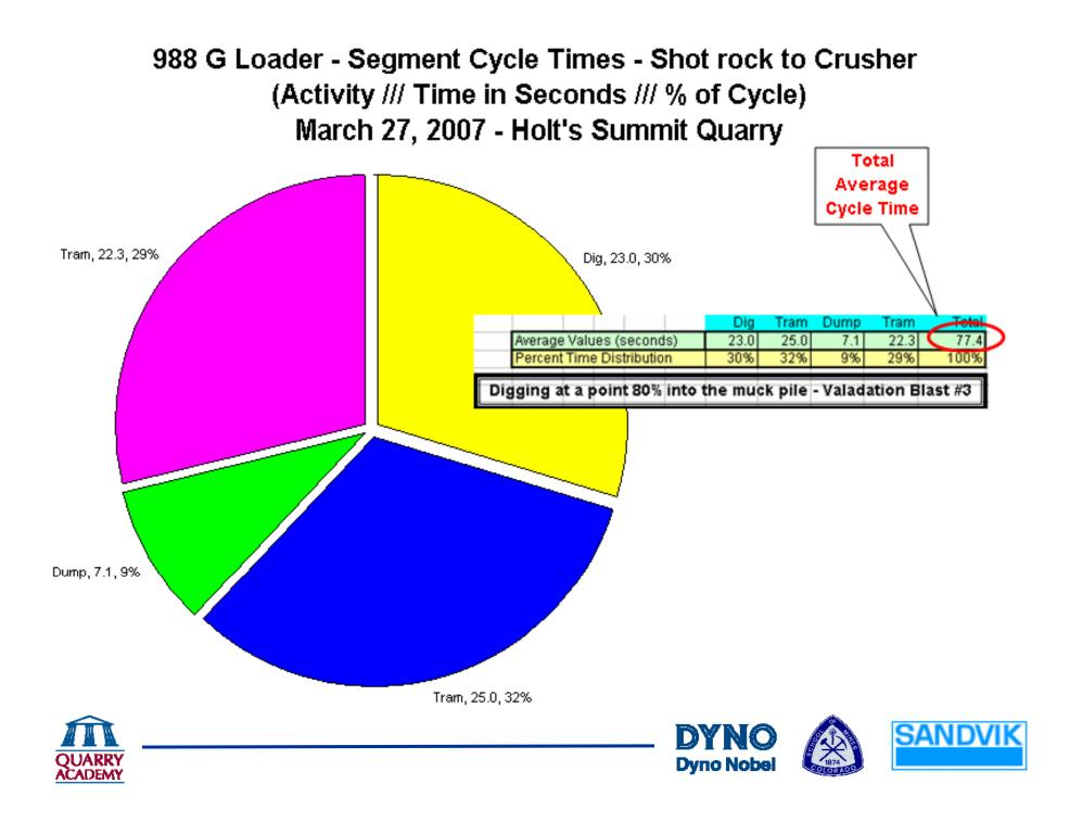
988 G Loader - Segment Cycle Times - Shot rock to Crusher (Activity /// Time in Seconds /// % of Cycle) March 28, 2007 - Holt's Summit Quarry
