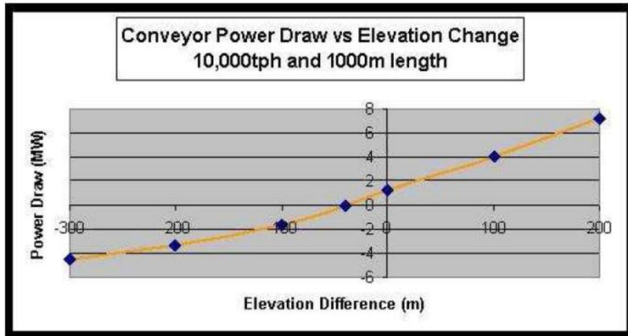
This shows that if we have downhill hauls, then **regardless of scale** a conveyor can generate power and offset the operating cost of the system
