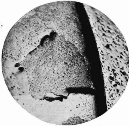
FIG. 55.—CRACKS AT GRAIN BOUNDARIES
