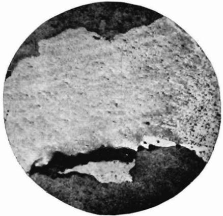
FIG. 56.—CRACK PARTLY THROUGH GRAIN
