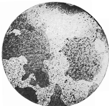
FIG. 29a.—TUNGSTEN INGOT CONTAINING 0.75 PER CENT.  $\text{ThO}_2$ , HEATED 20 MIN. AT  $2600^\circ\text{C}$ . AND THEN HEATED 10 MIN. AT  $3200^\circ\text{C}$ .  $\times 74$ .
