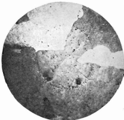
FIG. 31.—COARSE-GRAINED TUNGSTEN INGOT WITH FUSED CENTER.  $\times 17$ .
