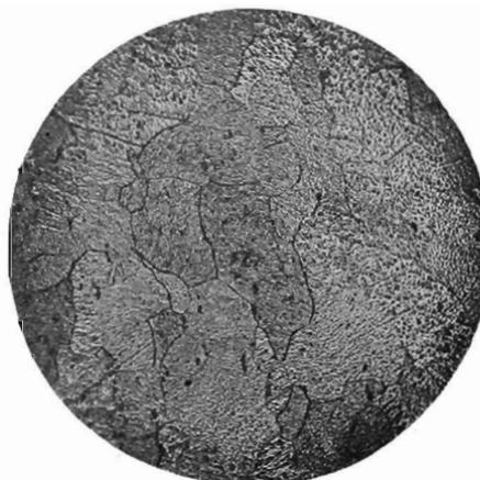
FIG. 39.—SWAGED TUNGSTEN ROD CONTAINING 0.75 PER CENT. ThO<sub>2</sub>, 0.080 IN. DIAM. RECRYSTALLIZED BY HEATING 3 MIN. AT 3100° C.  $\times 240$ .
