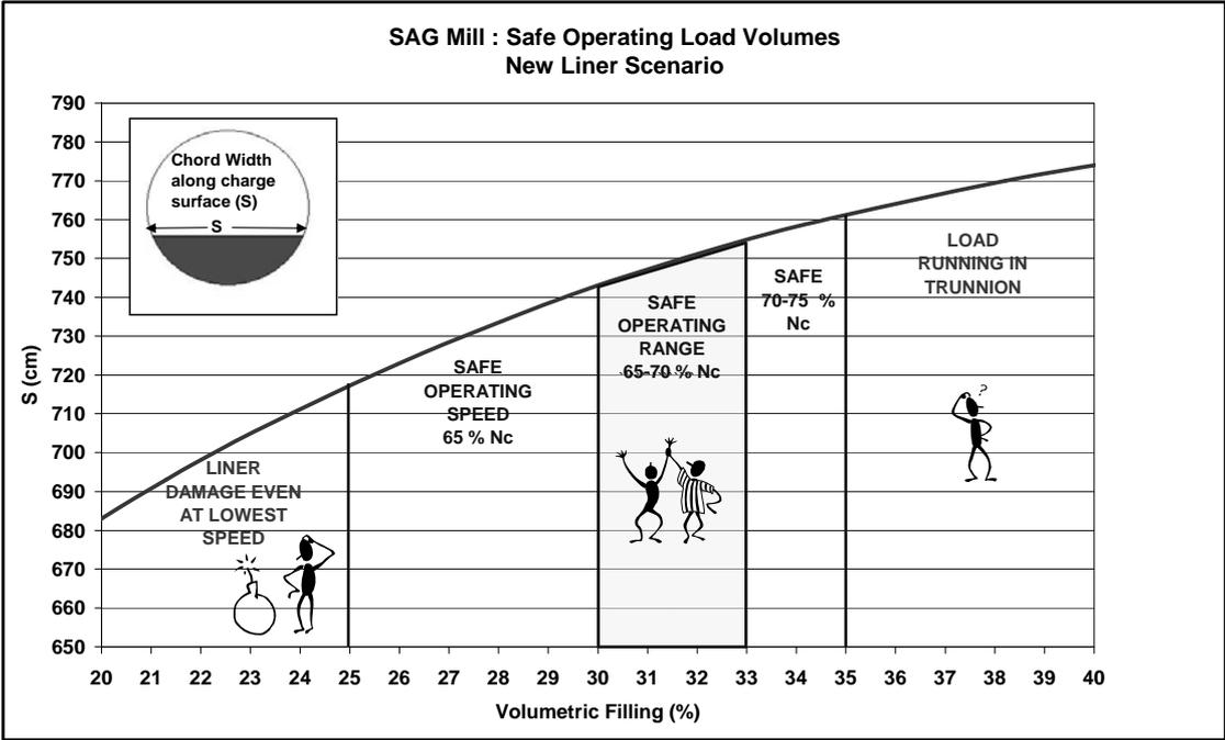
Figure 36. Example of defined safe operating window for a 6m SAG mill with new liners
