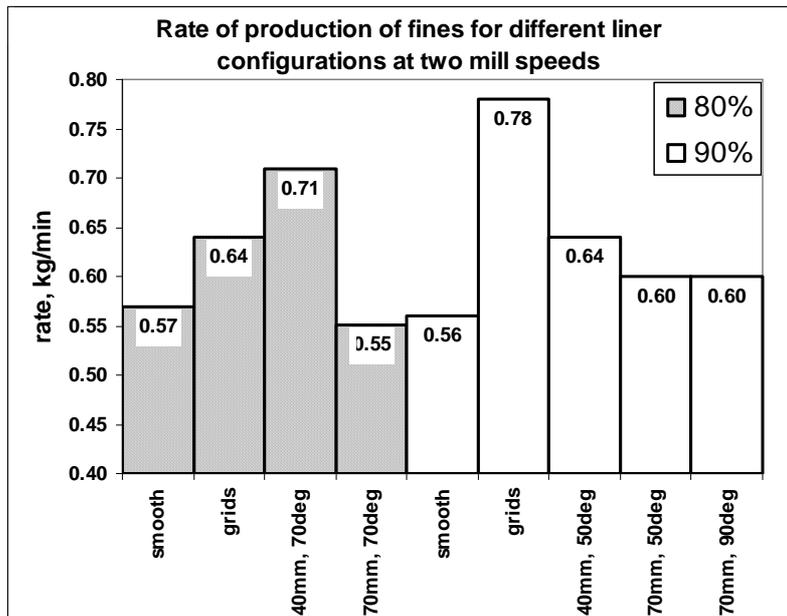
**Figure 13. Influence of liner profile on mill performance**
