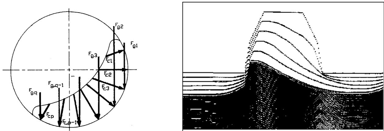
**Figure 15. a) Ball charge forces acting on mill liner b) Bevelled liner profile wear simulation**
