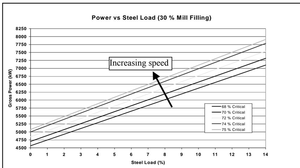
**Figure 39. Mill power versus steel loading for a 30ft mill at 30% total volumetric filling**
