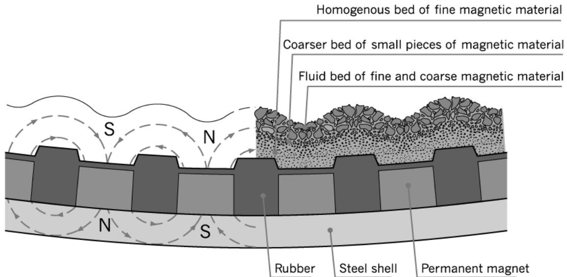
**Figure 9. Magnetic liner (Metso Orebed)**
