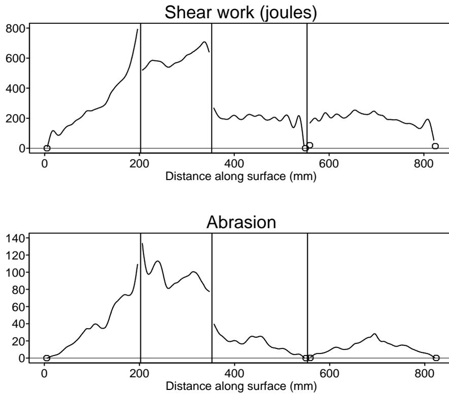
**Figure 31. Abrasive wear rate along the lifter and liner plate as given by the shear work and an angular dependent abrasion measure.**
