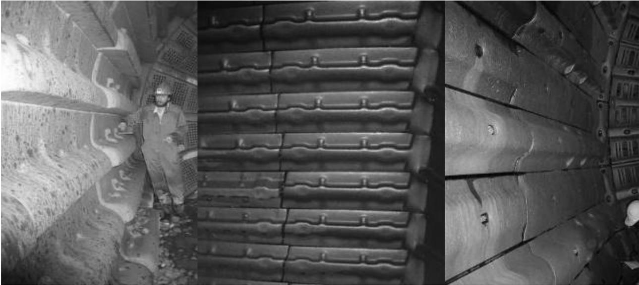
**Figure 1. Solid steel liners with integral lifter bars**
