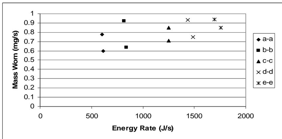
**Figure 18. Mass worn differences for similar energy rates (1045 steel, Ottawa foundry sand).**
