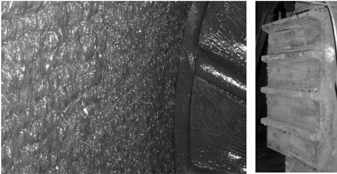
**Figure 10. Orebed liner in secondary ball mill, and a single panel**
