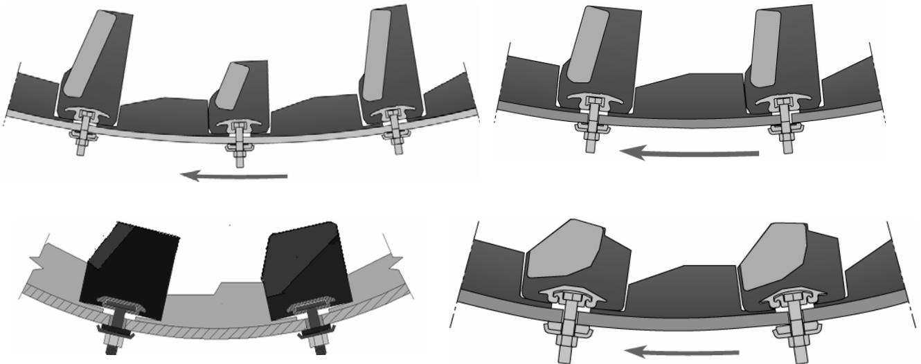
**Figure 7. configurations of Metal-capped rubber liners**
