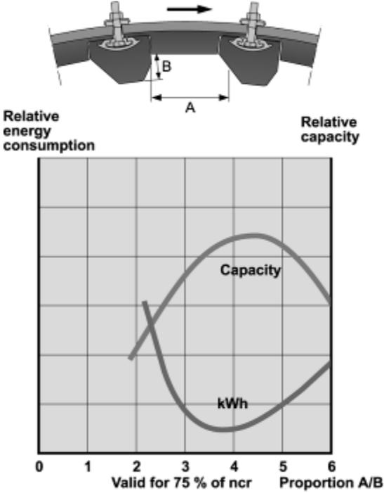
**Figure 20. The Skega A/B ratio related to mill capacity and throughput**
