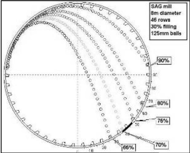
**Figure 22 Influence of mill speed on ball trajectory**
