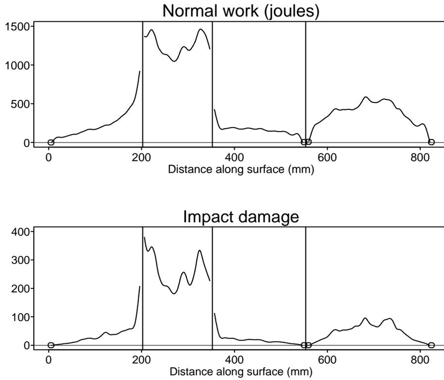
**Figure 30. Impact wear rate along the lifter and liner plate as given by the normal work and an impact damage measure.**
