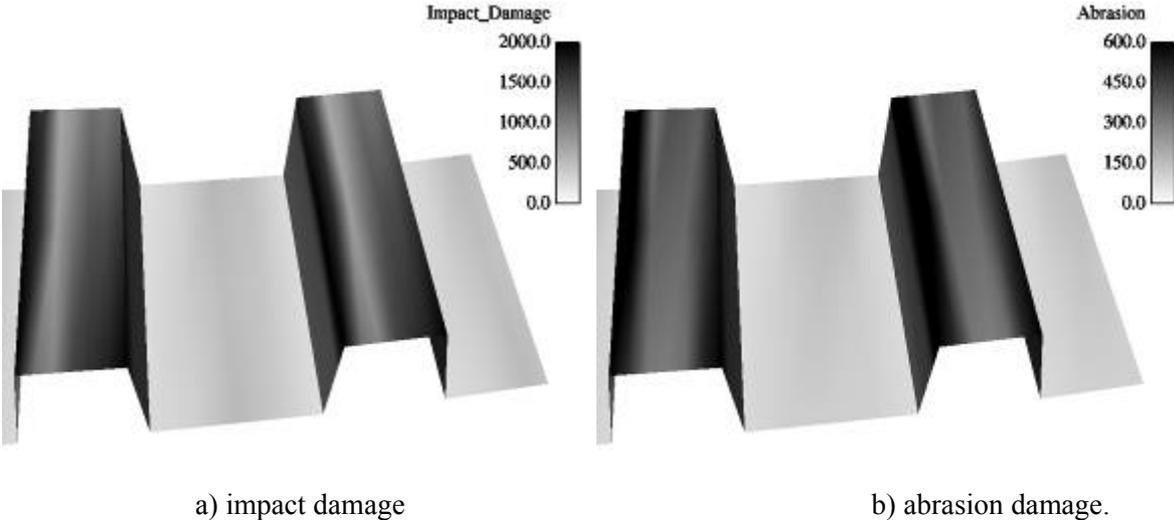
**Figure 29. Wear distributions on the SAG liner. Dark = high magnitudes, light = low.**
