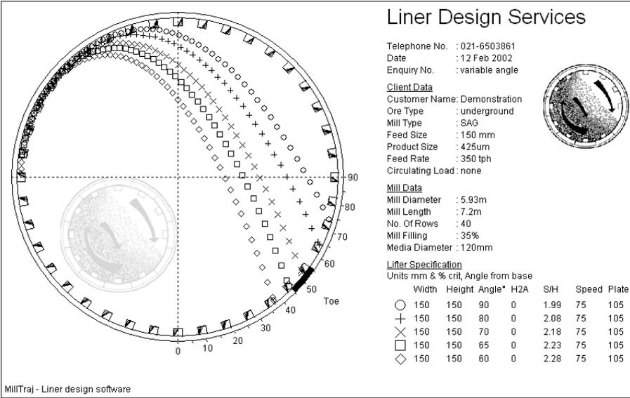
**Figure 21. Trajectories for different angled lifter bars**
