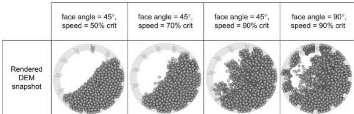
**Figure 25. Example of DEM charge motion predictions**
