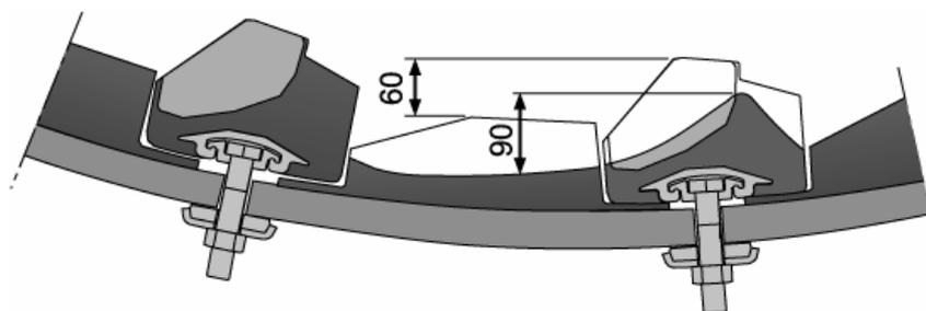
**Figure 8. Designing steel-capped liners for even wear**
