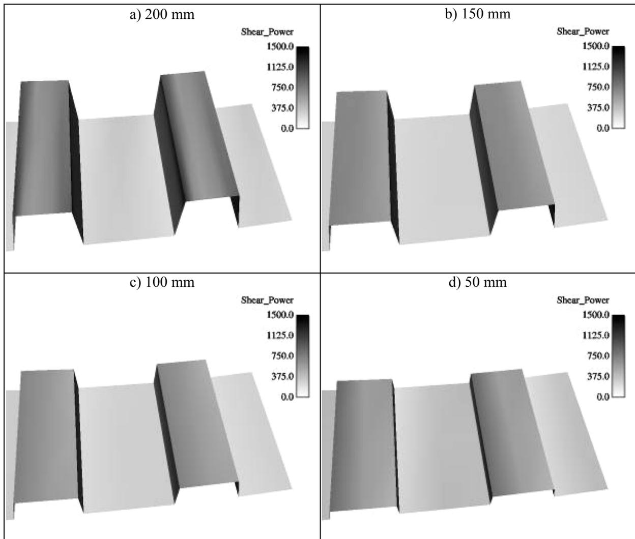
**Figure 32. Rate of shear energy (abrasive wear) on the liner as the lifter height is decreased in 50 mm increments.**
