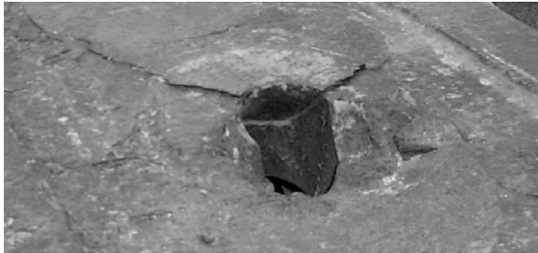
**Figure 11. bolt hole cracking**
