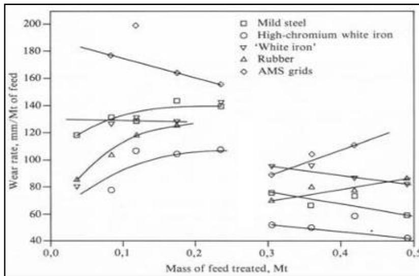
Figure 19. liner wear rate after lifter bar renewal, (Powell 1991b)
