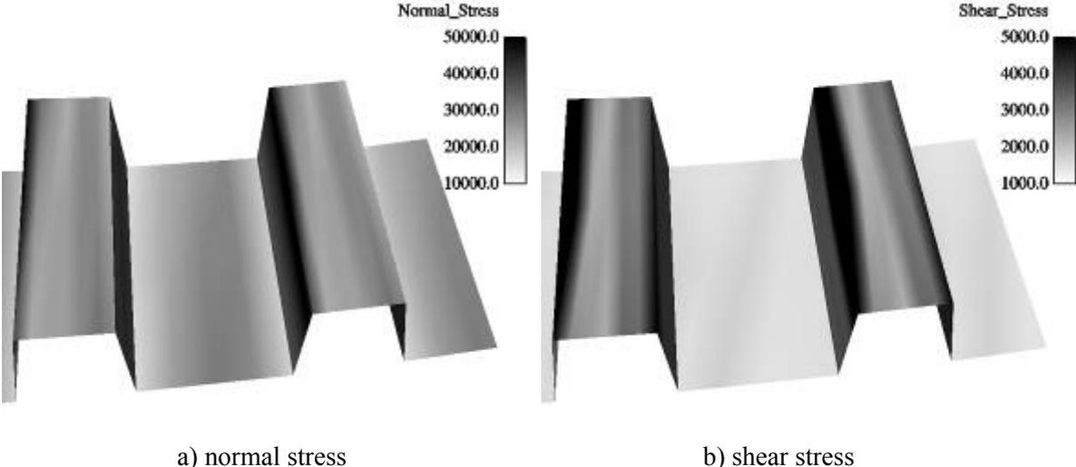
**Figure 27. Stress distributions on the SAG liner. Dark = high magnitudes, light = low.**
