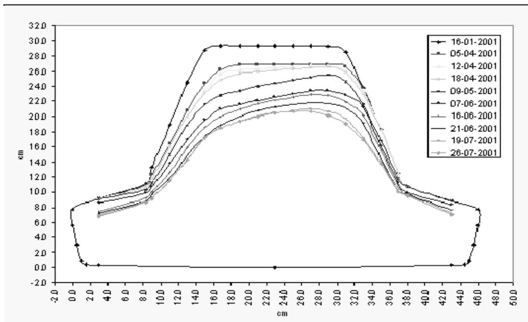
**Figure 34. The changing profile of a lifter bar in a 24ft diameter SAG mill**
