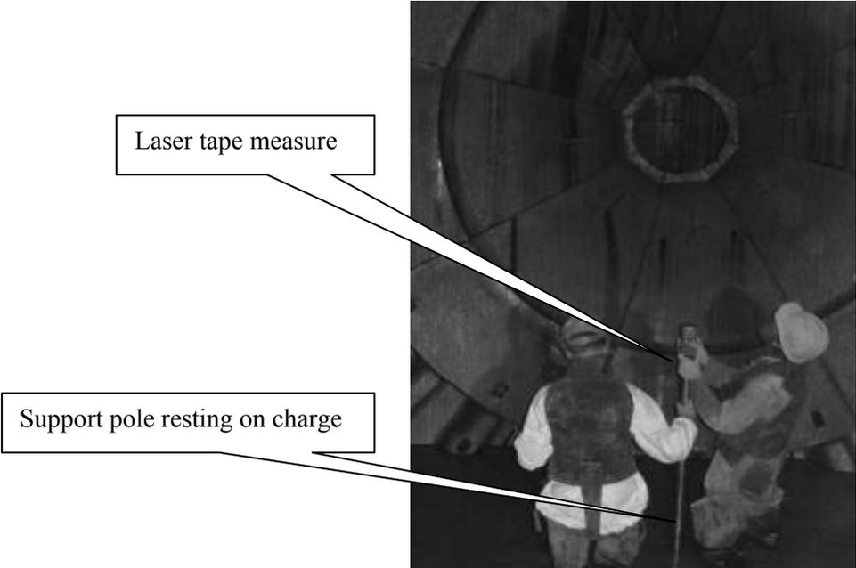
**Figure 37. Measuring the mill filling with a laser tape measure**
