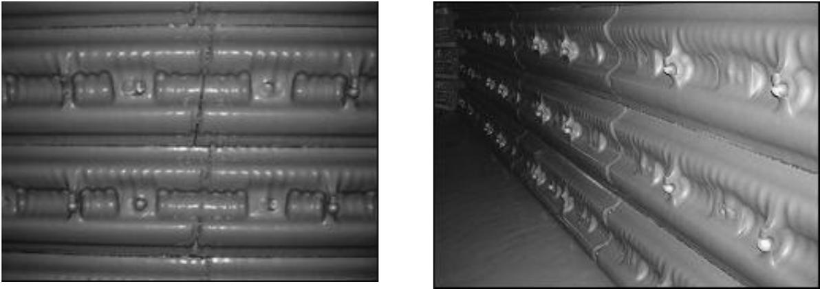
**Figure 35. Raceways and accelerated ‘pocketing’ resulting from the operation of a ball mill with too dilute a slurry charge**
