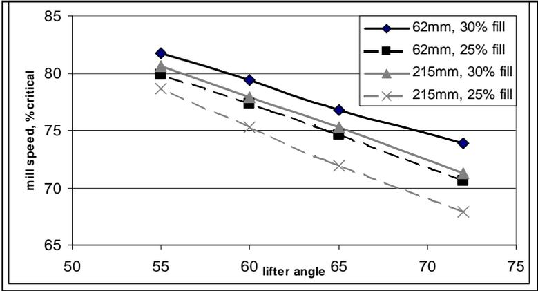
**Figure 23. Safe Operating Window of a mill as a function of speed, lifter angle, lifter height and mill filling**
