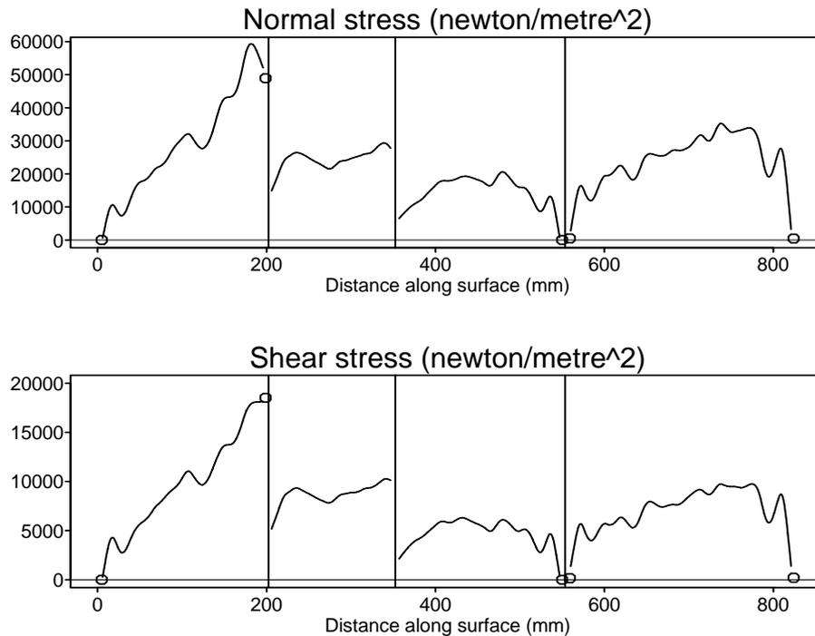
**Figure 28. Normal and shear stresses along the lifter and liner plate. The distance is measured from the base of the lifter front. Each region (lifter front, top and rear and finally the liner plate) is separated by a vertical line.**
