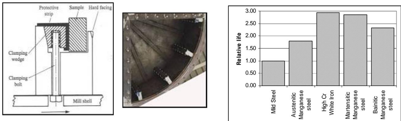
Figure 14. Wear testing mill and relative wear rates results
