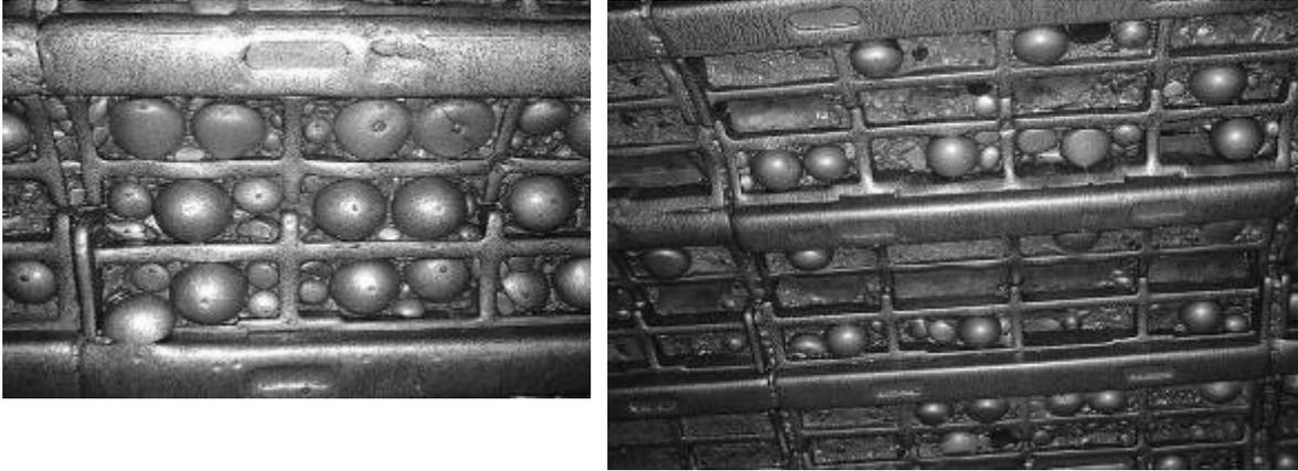
**Figure 3. Austenitic Manganese steel grid liners**
