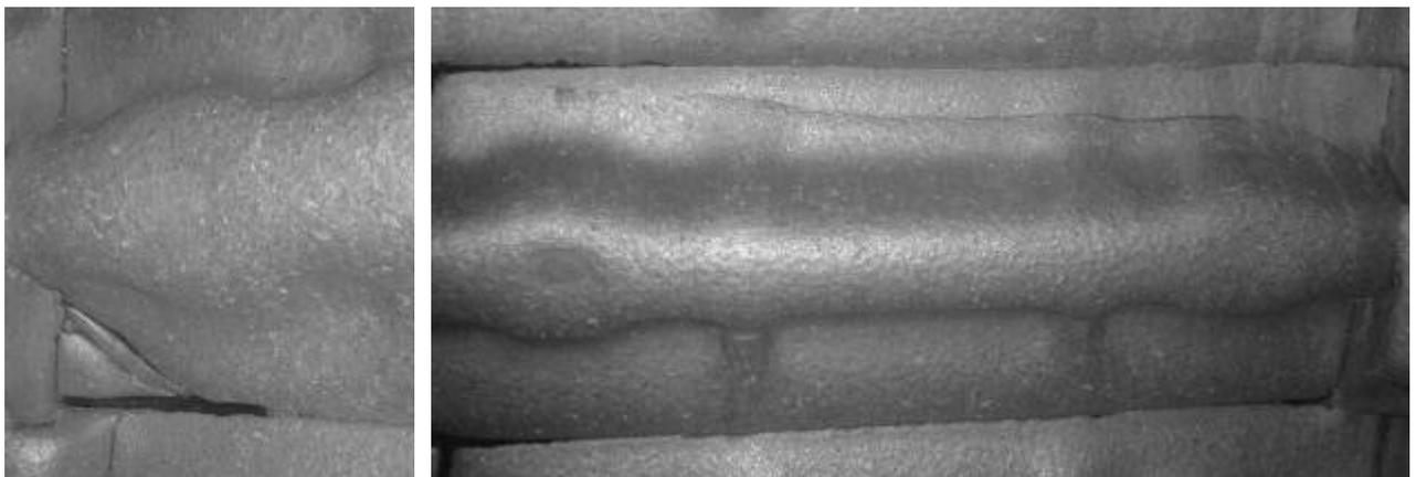
**Figure 12. Heavily dimpled, peened, and cracked liners**
