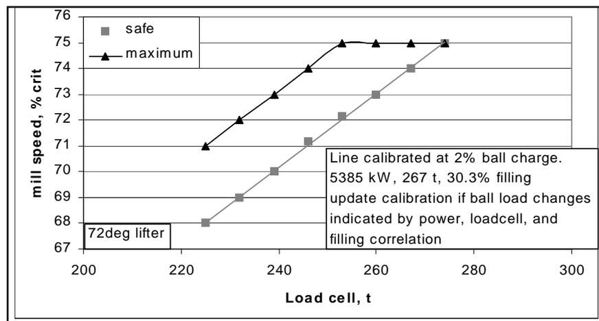
**Figure 24. Safe operating range as a function of mill speed and filling for an example mill with new high lifters with an aggressive face angle**
