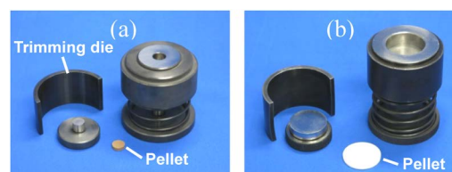
Fig. 5. Sample preparation with cylinder type dies.
