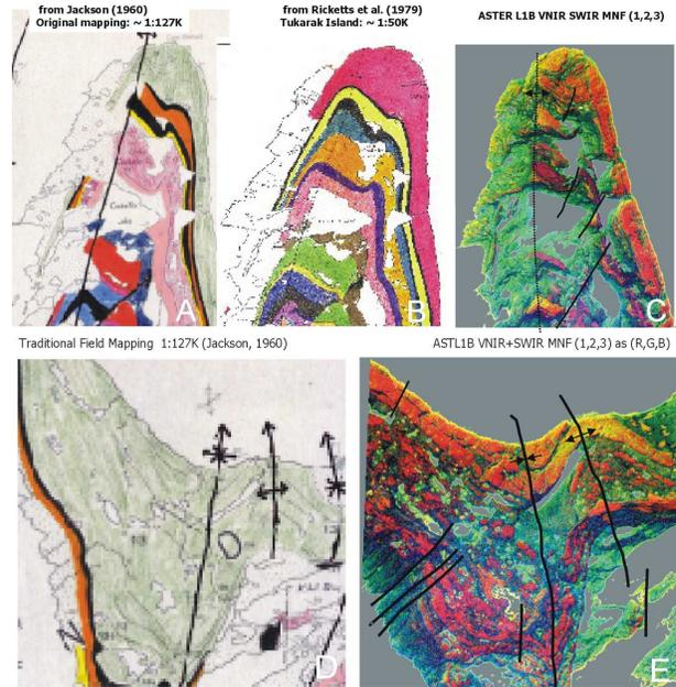
**Figure 3:** Two examples comparing field geological maps and RGB images based on MNF “endmembers” 1, 2, 3 computed from ASTER data. Geological maps are interpretive, since they do not specifically address the distribution of any overburden. Both examples show increased detail provided by the ASTER imagery. A) Jackson (1960), B) Ricketts et al. (1982), C) ASTER, D) Jackson (1960), E) ASTER.
