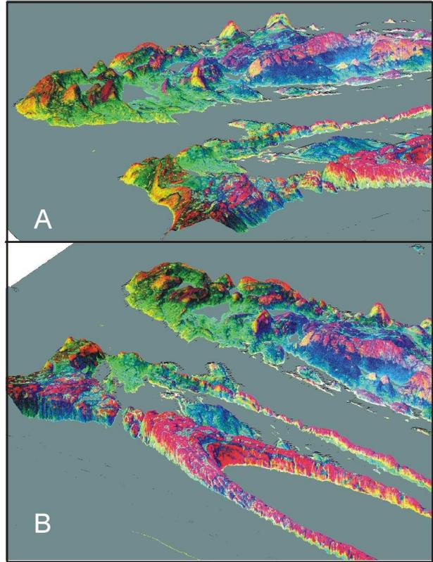
**Figure 5:** A) and B): Southeasterly and northeasterly views of the MNF 1, 2, 3 image orthorectified to the SRTM topographic surface. Note the relationship between cap rock units and topographic ridges, co-incident of topography variations with lithological variations at fold noses.
