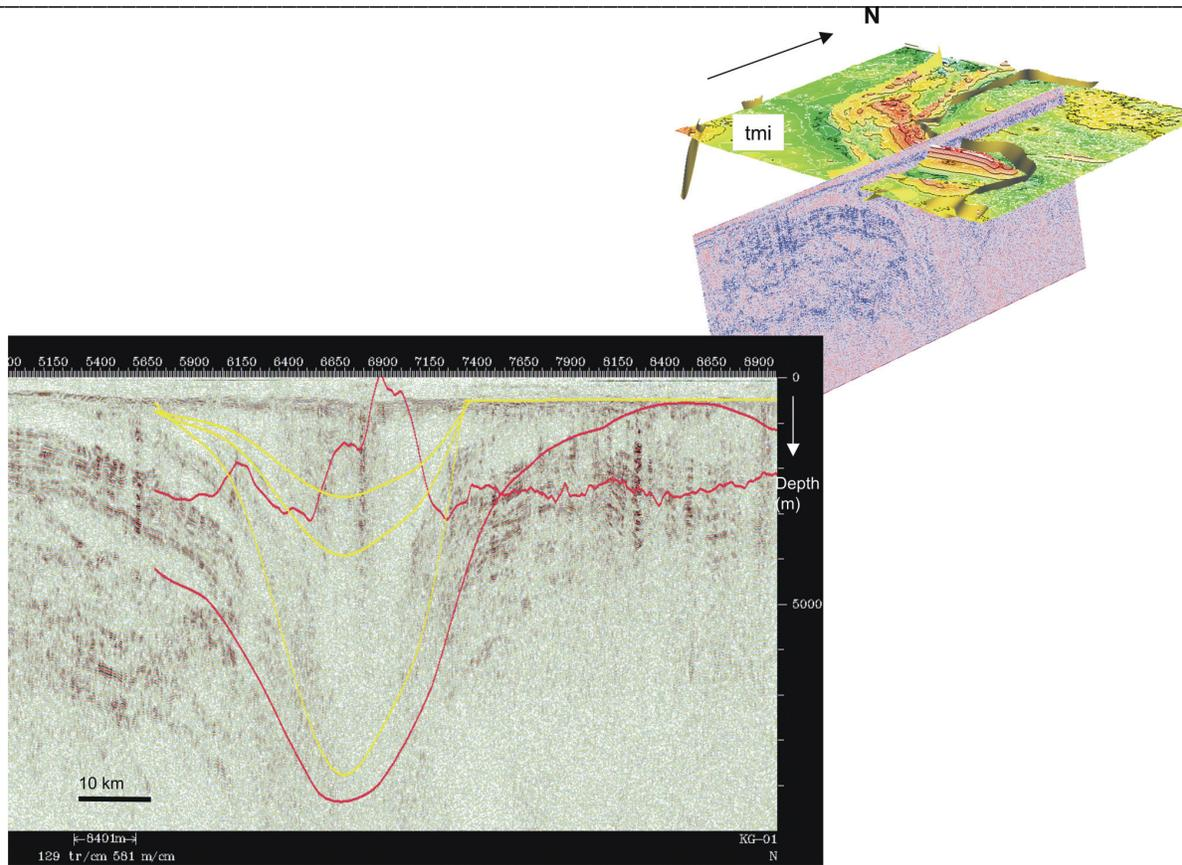
**Figure 4:** Syncline shape from Bouguer anomaly structural inversion (in yellow). Increasing depths are obtained for decreasing density contrast (respectively for 0.3, 0.2 and 0.1 gcm-3 from top to bottom). The TMI and Bouguer anomaly (inverted in the figure) have been overlaid in red. Top right corner: location plot of the KG-01 section below the magnetic anomaly.
