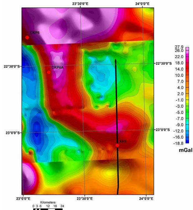
Figure 2. Bouguer gravity anomaly (Left; mGal). The contours of the anomaly are displayed only in the area used for the inversion.
