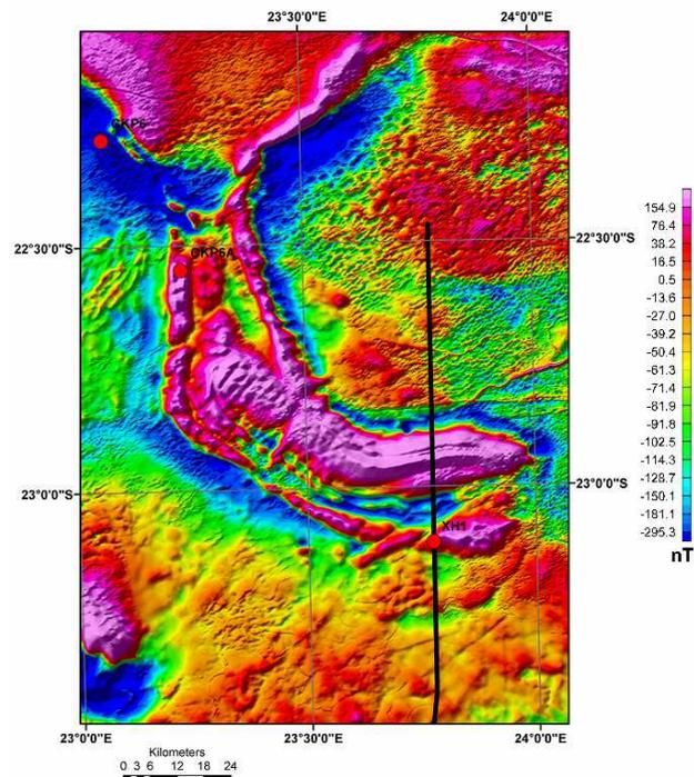
**Figure 1:** Total Magnetic Intensity over the Xade complex. Seismic line boreholes referred in the text are indicated.
