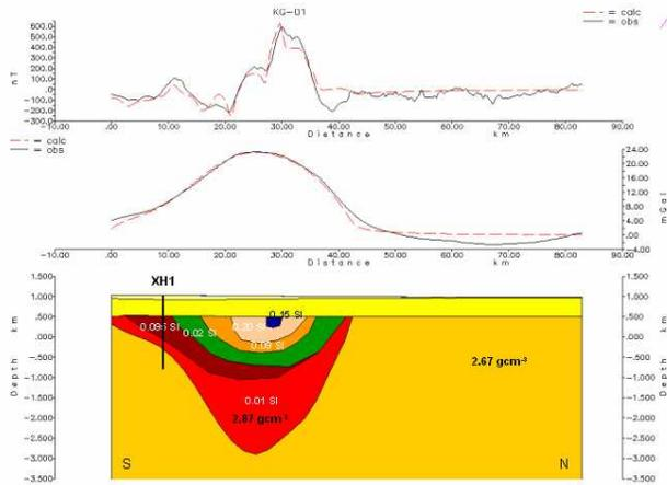
Figure 3: 2D gravity and magnetic modelling across the Xade complex (along line KG-01).
