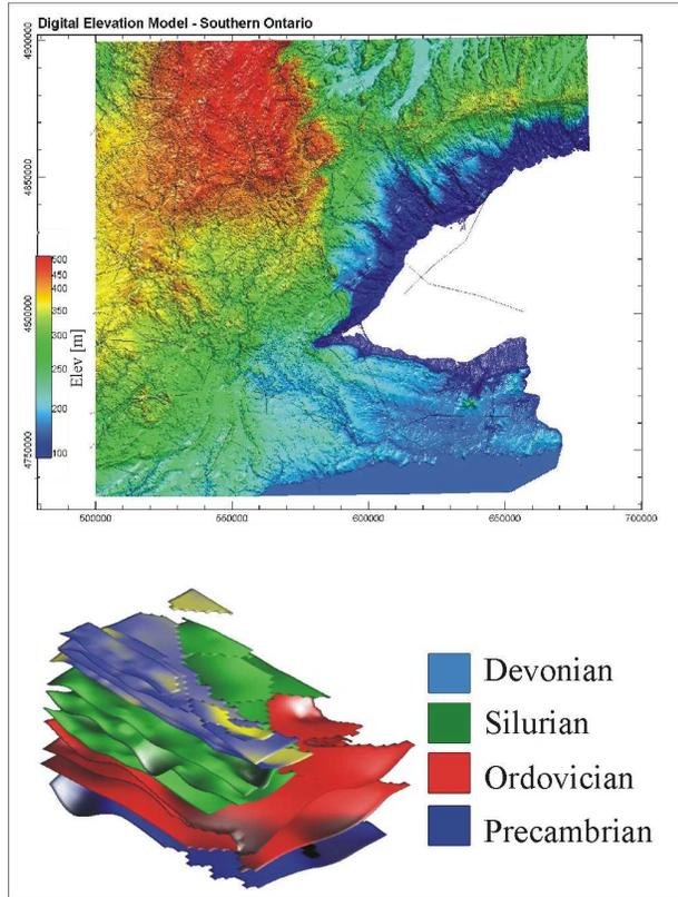
**Figure 3:** Top, digital elevation model of the area of study, with linear features extracted from the different stratigraphic levels. Bottom, 3D model of the different stratigraphic levels, as mapped from borehole lithological logs. Each 3D surface represents the top of the corresponding geological unit.
