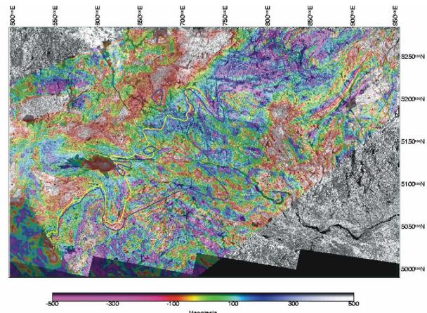
**Figure 5:** OGS 800m grid cell aeromagnetic data overlain on Landsat panchromatic Band 8. Ottawa – Bonnechere graben complex is identified by black lines. Thrust boundaries as presented in Figure 4.
