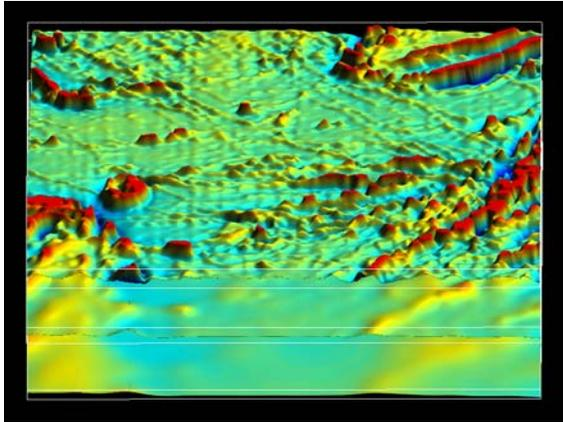
**Figure 4:** Pseudo-topographic representation of variation of total magnetic field variation over study area. Image based on Ontario Provincial data set after micro-levelling and band-pass filtering to accentuate near – surface sources.
