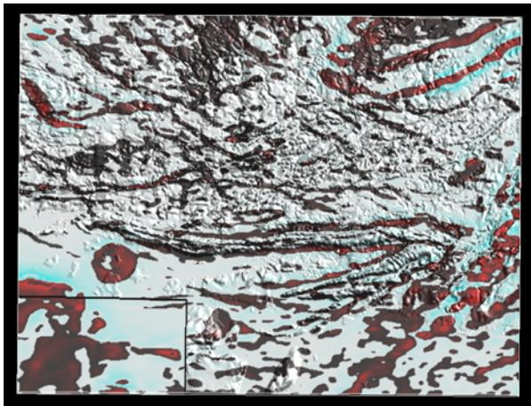
**Figure 5:** Aeromagnetic data draped over topographic surface. Histogram distribution of magnetic data set is modified to accentuate magnetic highs (red) and lows (blue).
