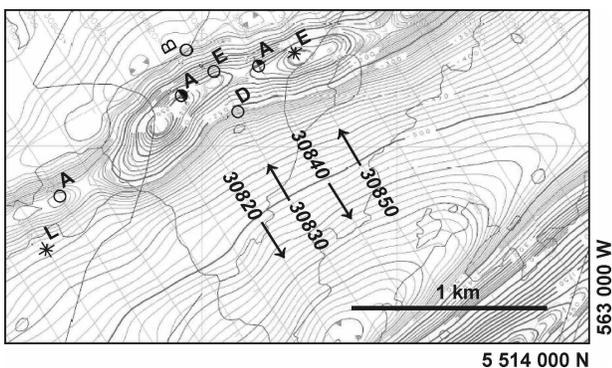
**Figure 5:** EM anomalies plotted on a contour map of the residual total magnetic field. Anomaly D from line 30830 is a dip effect, the conductor axis is located under anomaly E. Coordinates are UTM, Zone 18.
