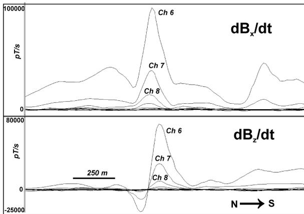
**Figure 2:** MEGATEM II response over the Scott deposit. Channel 6 is the first off-time channel of the system.
