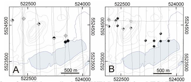
**Figure 3:** (A) EM anomalies from INPUT Mk VI, (B) from MEGATEM II survey. Coordinates are UTM, Zone 18.
