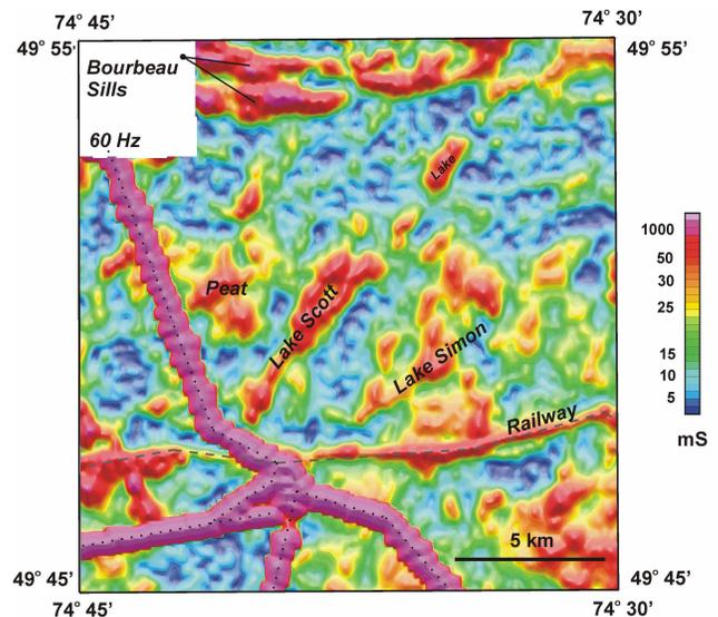
**Figure 6:** Apparent conductance over a portion of Block A. Note the effect of power lines and the railway. Glacial direction is north east and geological strike east west.
