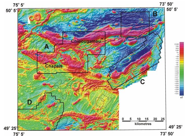
**Figure 1:** Location of the 4 survey blocks superimposed on the residual total magnetic field from 200 m line spacing INPUT surveys flown at a height of 120 m.
