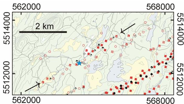
**Figure 4:** New anomalies along the Lemoine mine horizon. Arrows point to the horizon. The blue star locates the mine. MEGATEM II anomalies are black, INPUT anomalies red. Coordinates are UTM, Zone 18.
