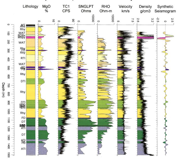
**Figure 2:** Logview presentation of lithology (from chemistry and mineralogy), whole rock chemistry - magnesium, total count natural gamma (TC1, cps), single point electrical resistance (SNGLPT, Ohms), electrical resistivity (RHO, Ohm-m), acoustic velocity in kilometres per second, density (or specific gravity) in grams per cubic centimetre, and a synthetic seismogram derived from the velocity and density.
