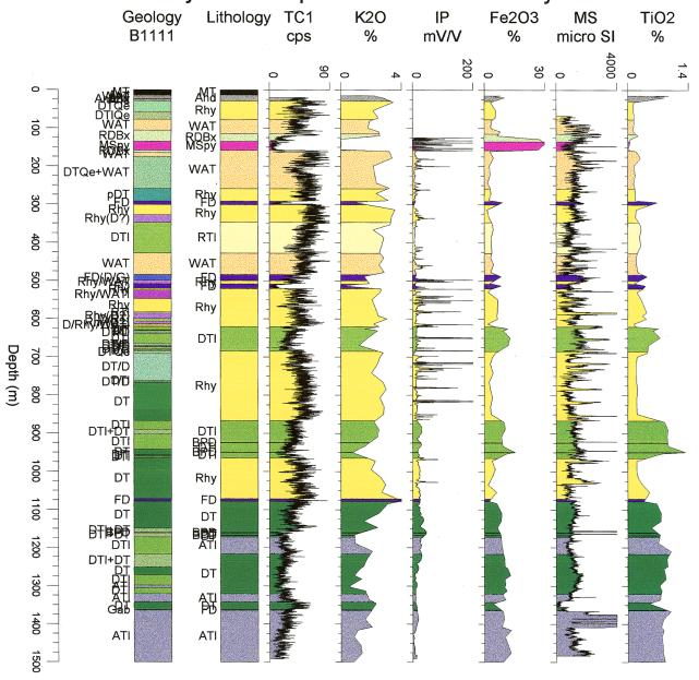
Figure 1: Logview presentation of geology (macroscopic visual), lithology (revision of geology from chemistry and mineralogy), total count natural gamma (TC1, cps), whole rock chemistry - potassium (K2O%), induced polarization (IP, mV/V), whole rock chemistry - iron (Fe2O3%), magnetic susceptibility (MS, micro SI), and whole rock chemistry - titanium (TiO2%).
