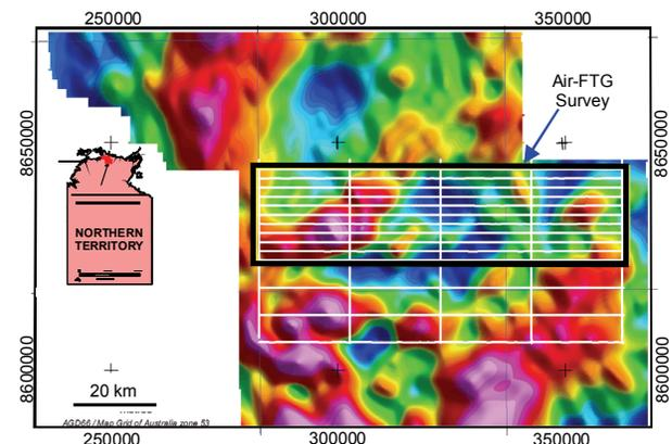
**Figure 1:** The location map of a test survey at West Arnhem Land, Australia and the free Air Gravity data from the 2003 GTIA survey. The Air-FTG<sup>®</sup> survey location is shown in black rectangle. The GTIA data is obtained from Australian Geoscience's website.
