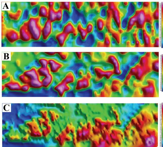
**Figure 2:** (A) First vertical derivative of airborne gravity ( $T_{zz\_GT1A\_1VD}$ ), (B) Free air full tensor processed vertical gradient data as measured by the Air-FTG<sup>®</sup>, (C) Digital Elevation Model.
