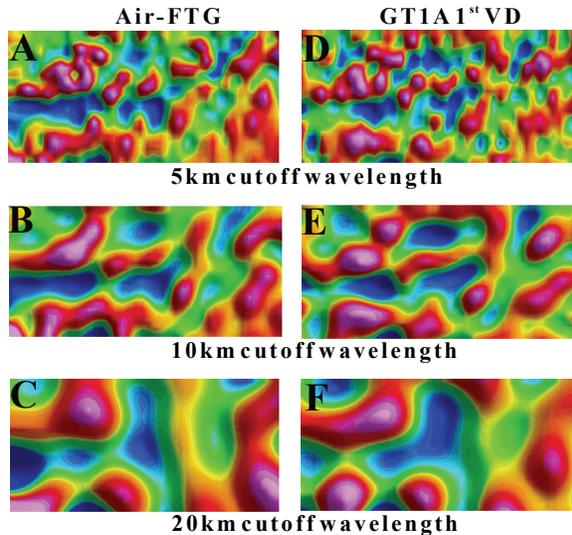
**Figure 3:** Frequency filtering analysis slices between Air-FTG and GT1A at short (A and D), intermediate (B and E) and long wavelengths (C and F).
