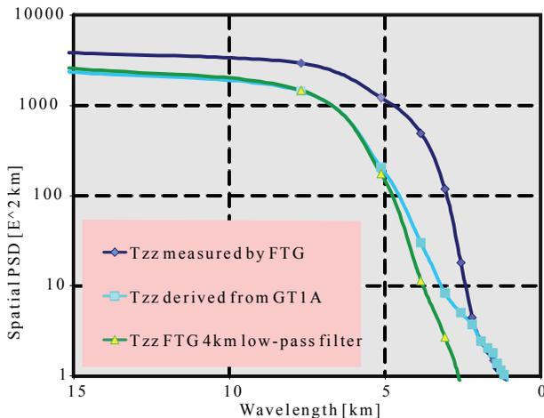
**Figure 4:** Spectral comparison of Tzz measured by the FTG and derived from GT1A airborne gravimetry. The FTG spectrum is shown with and without application of a 4 km low-pass filter. Note that the horizontal is reversed.
