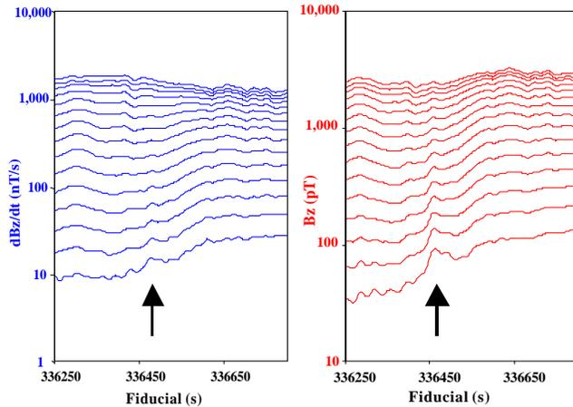
**Figure 12:** Comparison of a dB/dT and a B-field response. The black arrows indicate the position of a massive sulphide conductor. The dB/dT (response on left) and B-field (response on right) data were gathered concurrently. The enhanced late time (lower channels) of the B-field is (are) clearly evident.. After Wolfgram and Thomson, 1998.
