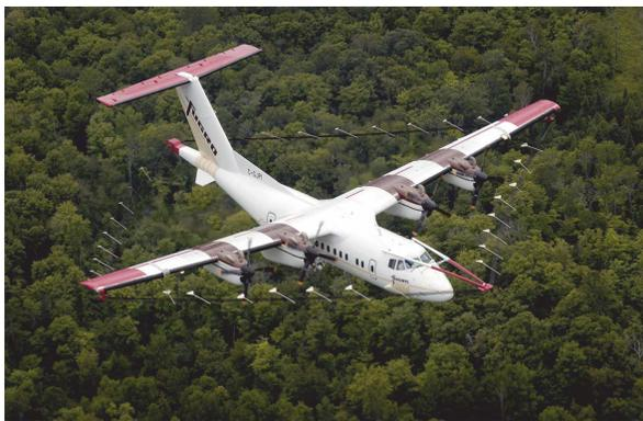
**Figure 13:** The MEGATEM™ system was developed for high altitude applications, but also enabled the development of higher power systems as measured by peak dipole moment. Courtesy of Fugro Airborne Surveys
