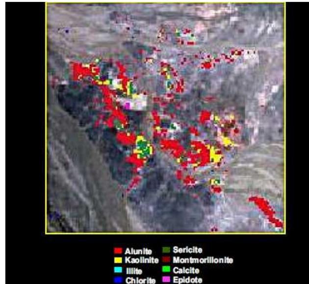
**Figure 21:** Cutout from Figure 17. The resolution of hyperspectral technology can create a detailed suite map of related minerals. After Stevens and Zamudio, undated web publication.
