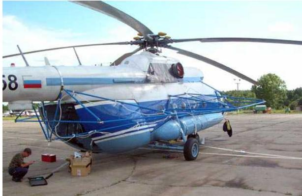
Figure 10: The EM-4H conductivity mapping system which uses a transmitter loop attached to the helicopter and a towed body receiver. Courtesy Andrey Volkovitskiy.
