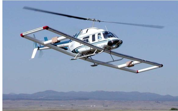
**Figure 16:** The ORAGS-TEM system developed for unexploded ordnance detection where high near-surface spatial resolution and reliability of detection is required. Courtesy of the Oakridge National Laboratory
