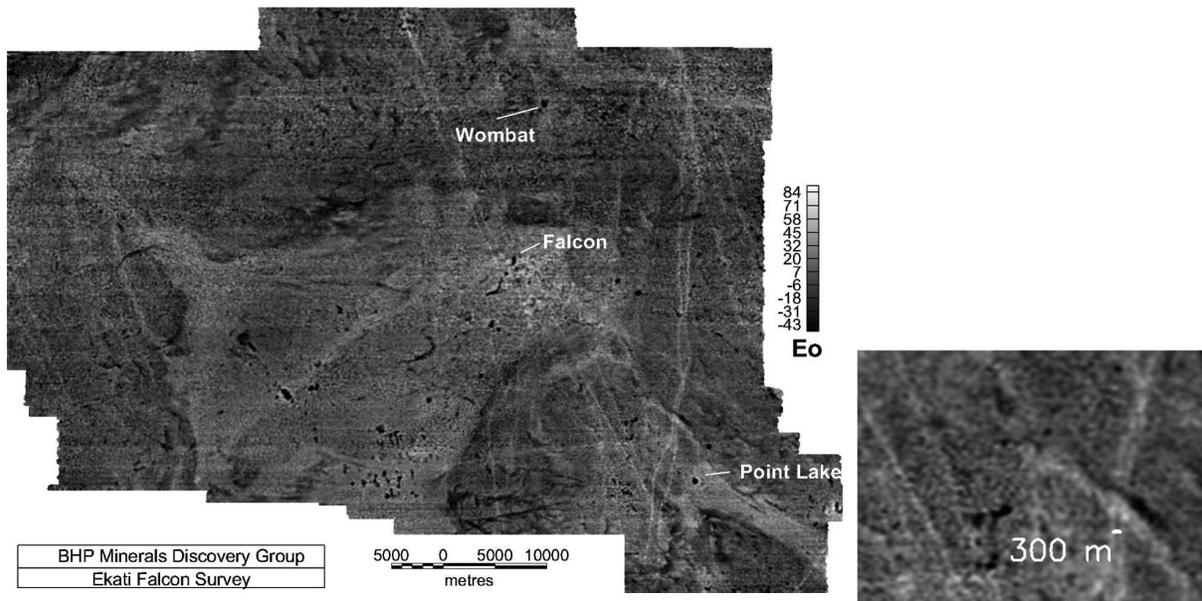
Figure 6: The vertical gravity gradient from a survey near the Ekati mine, Canada. The image on the right shows an enlargement of a section in the lower right of the main image. Two narrow dykes separated by about 300 m (as indicated by the white bar) are resolved by the gravity gradient measurements. After Liu et al, 2001.
