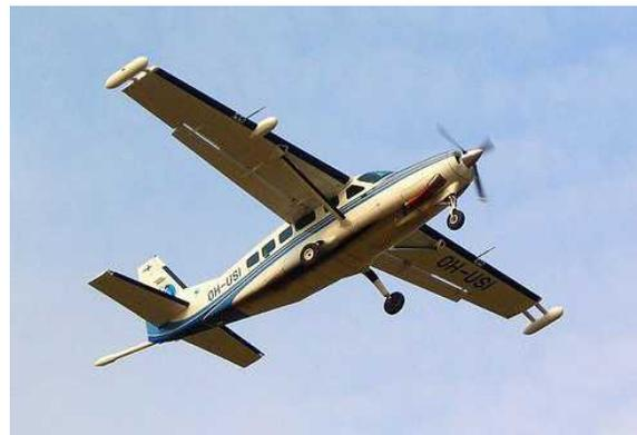
**Figure 9:** A typical fixed wing frequency domain electromagnetic system with wingtip mounted transmitter and receiver pods clearly visible. The tail stinger is not a component of the EM system; it contains a magnetometer. Courtesy of GTK
