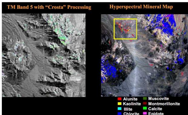
**Figure 20:** Comparative mineral maps from Landsat and airborne hyperspectral over an area of Chile. The area delineated by the yellow box is shown below. After Stevens and Zamudio, undated web publication.
