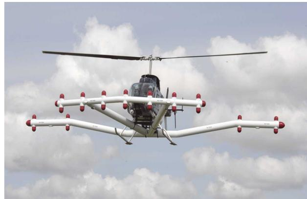
**Figure 2:** The ORAGS VG-22 system with 11 boom mounted vertical gradiometers (22 total field magnetometers) for UXO detection. Courtesy of Oak Ridge National Laboratory
