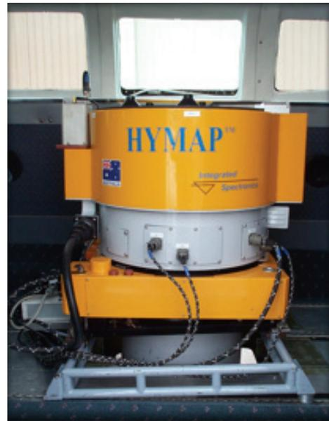
**Figure 3:** The HyMap instrument mounted in a survey aircraft. The lower part of the system is a stabilized platform.
