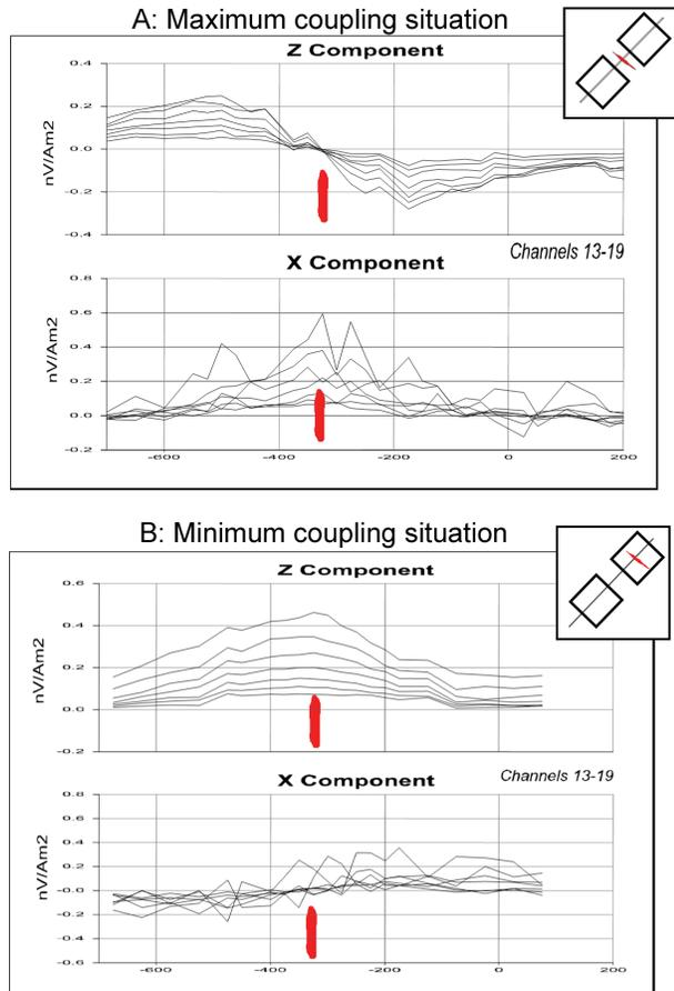
**Figure 3:** InfiniTEM® survey results over Caber-North deposit (in red) using a loop design of 400 x 400 m half-loops 200 m apart. A: The deposit is located in the area of horizontal primary field yielding in a maximum coupling situation. B: The deposit is located in the area of vertical primary field yielding in a minimal coupling situation. For both cases, the 350 m deep conductor is detected. A Protem 67D and a TEM57 and TEM67 transmitting combo were used to energize the ground with 8 amps.
