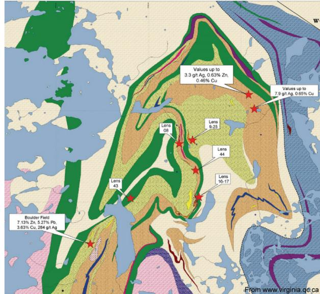
**Figure 4:** Geological plan map of the Coulon Property, Quebec James Bay low lands (Virginia Mines Inc.). Lens 43 is located within the green volcanic belt.
