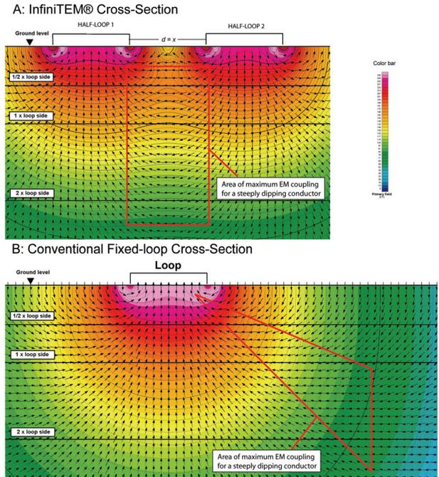
**Figure 2:** Comparison of primary field cross-section for both InfiniTEM® and conventional rectangular loop configurations in the case of steeply dipping conductor exploration. For a vertical conductor buried at a depth equivalent to  $2x$ , the InfiniTEM® survey provides a more intense horizontal primary field (cyan zone) than the conventional loop design (light blue zone).
