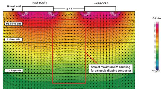
B: Conventional Fixed-loop Cross-Section
