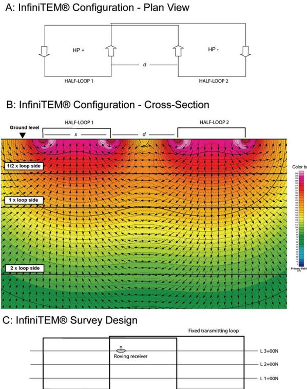
**Figure 1:** InfiniTEM® configuration setup. A: plan view, B: associated primary field cross-section showing field orientation (arrows) and intensity (color) computed with Biot-Savard equation, C: plan view of a typical survey design.
