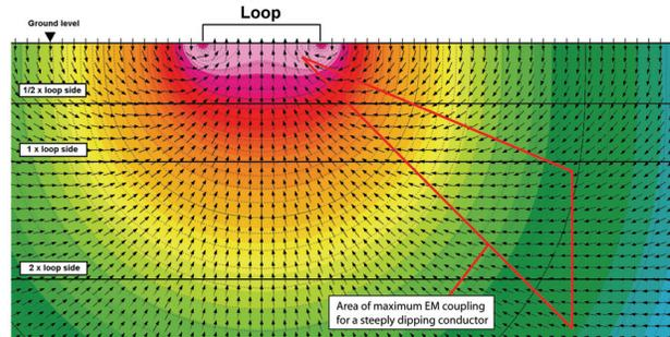
**Figure 2:** Comparison of primary field cross-section for both InfiniTEM® and conventional rectangular loop configurations in the case of steeply dipping conductor exploration. For a vertical conductor buried at a depth equivalent to  $2x$ , the InfiniTEM® survey provides a more intense horizontal primary field (cyan zone) than the conventional loop design (light blue zone).
