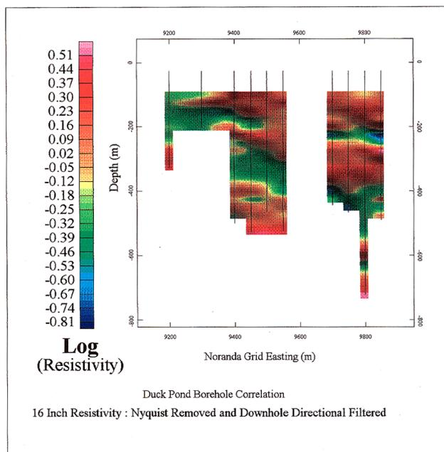
Figure 4: Gridded 16" resistivity section.
