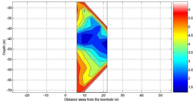
**Figure 3:** VRP apparent resistivity pseudo-section for a borehole which intersects massive sulfides at the depth of 40 – 50 m.
