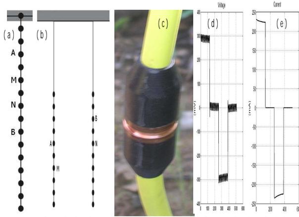
**Figure 1:** (a) borehole electrode cable deployment for vertical resistivity profiling; (b) cross borehole tomography; (c) copper-ring electrode; (d) measured voltage waveform; and (e) injected current waveform for 130 m electrode separation between boreholes.
