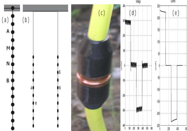
**Figure 1:** (a) borehole electrode cable deployment for vertical resistivity profiling; (b) cross borehole tomography; (c) copper-ring electrode; (d) measured voltage waveform; and (e) injected current waveform for 130 m electrode separation between boreholes.
