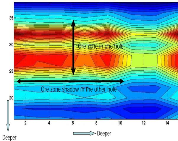
**Figure 6:** Electric current flowing between electrodes in two boreholes with constant voltage excitation. One borehole intersects an ore zone, while the other borehole passing this zone at a distance.
