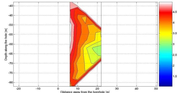
**Figure 4:** VRP apparent resistivity pseudo-section for a borehole which passes a massive sulfide ore body at a distance. From this pseudo-section, we can see that a massive sulfide zone is about 15 m away from the borehole at the depth of 60-70 m. Note the decreasing apparent resistivity with large offset.
