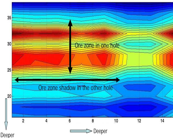
**Figure 6:** Electric current flowing between electrodes in two boreholes with constant voltage excitation. One borehole intersects an ore zone, while the other borehole passing this zone at a distance.
