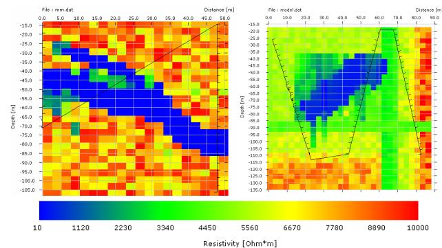
**Figure 7:** Two examples of BRT models derived from 2D tomographic inversions from the Sudbury area. The borehole traces are projected onto the 2D plane, where the resistivity structure is inverted. We assume the resistivity structure will not change in the direction perpendicular to the 2D plane.
