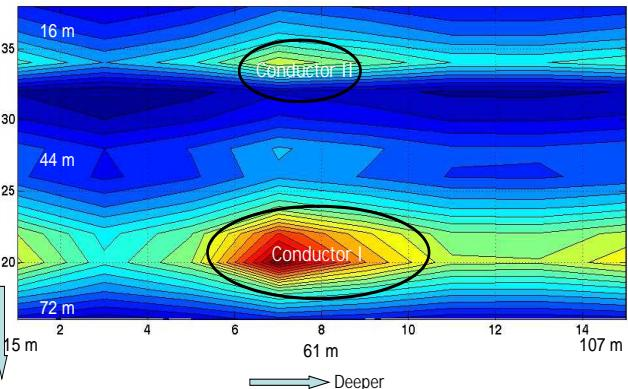
**Figure 5:** Quality control of electric current flowing between electrodes in two boreholes with constant voltage excitation. Note the data shows characteristics of two conductive zones between the pair of boreholes.
