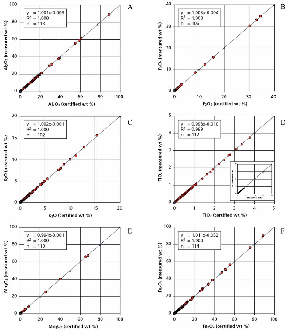
Figure 2: Accuracy verification: comparison of certified and measured values for the WROXI standards and a large number (n) of RMs. The regression values y, x and R2 are for the RMs only.
