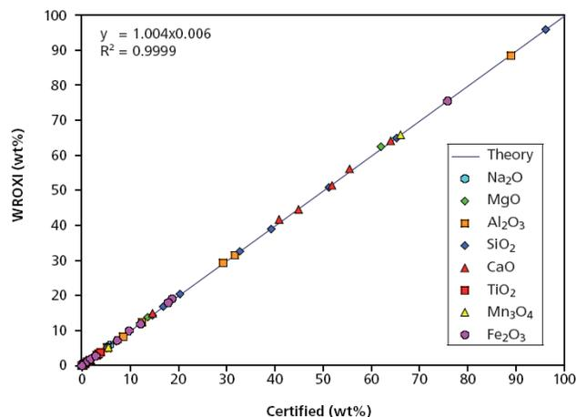
**Figure 1:** Accuracy overview: comparison of certified and measured values for 8 oxides in the wide variety of RMs listed in Table 2.
