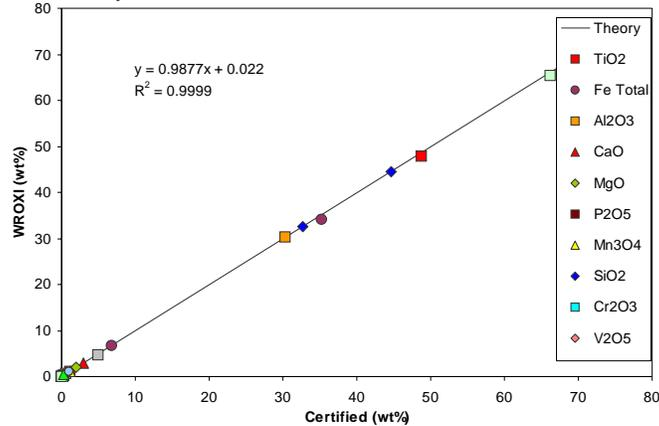
Figure 3: Courtesy Rio Tinto Fer & Titane. Validation of synthetic standards by external standards (Brammer 3701 (coke ashes) SARM 59 (ilmenite), BCS 388 (zircon) in the analysis of the titanium oxide process.
