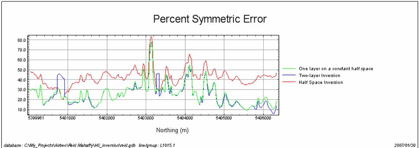
Figure 6: Plot of the percent symmetric error for one-layer and two-layer inversions on line 15 with AIRBEO.
