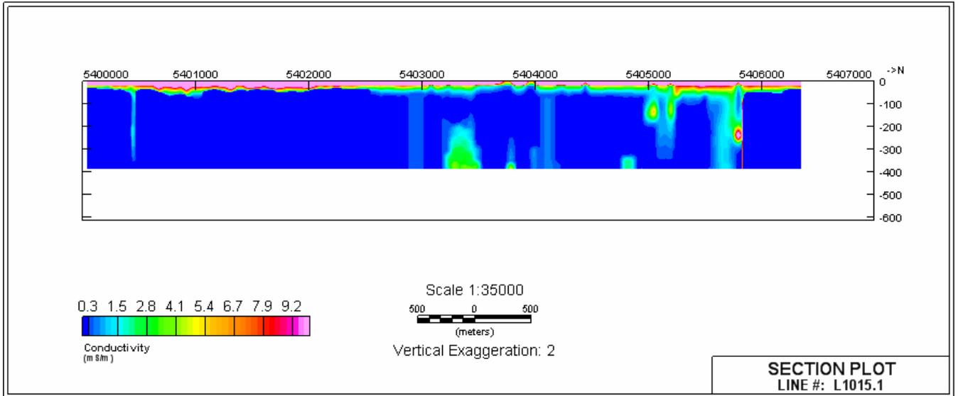
Figure 1: Conductivity-depth transform of B-field GEOTEM data for Reid-Mahaffy line 15.
