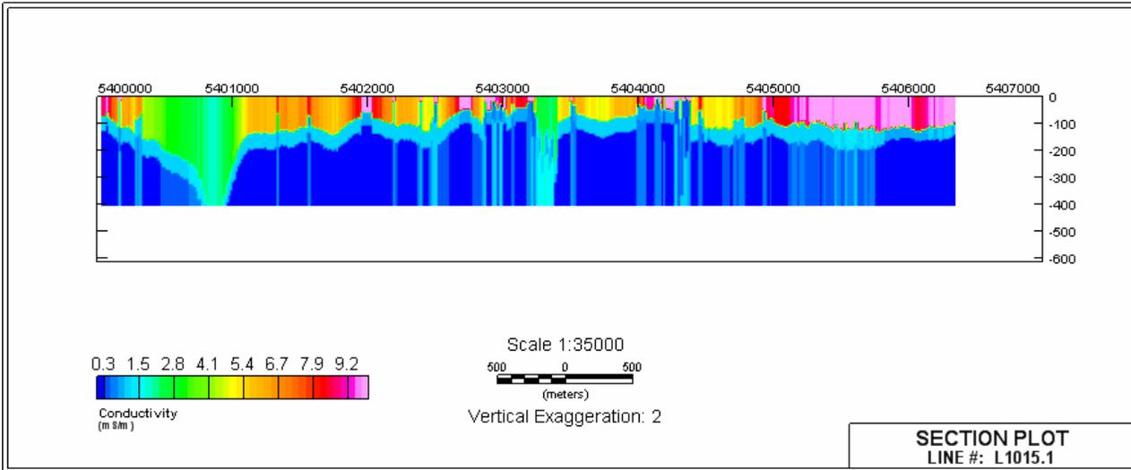
Figure 7: Three-layer inversion of line 15 with an initial model of 10 mS/m, 50 m, over 1 mS/m, 50 m, and a half-space of 0.1 mS/m.
