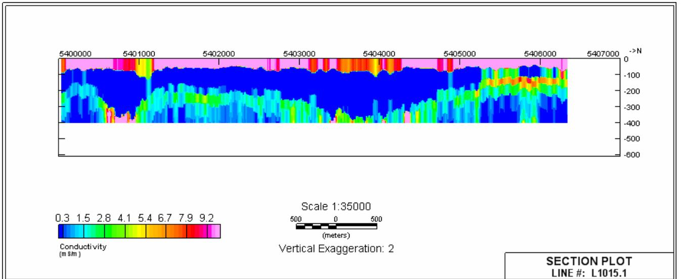
Figure 2: Conductivity image along Reid-Mahaffy line 15 using Zohdy's method.
