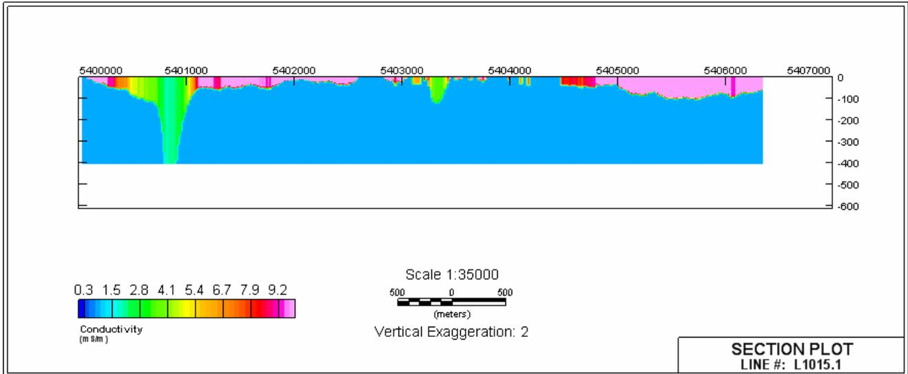
Figure 5: Two-layer inversion with a fixed basement of 1 mS/m on line 15 at Reid Mahaffy with AIRBEO.
