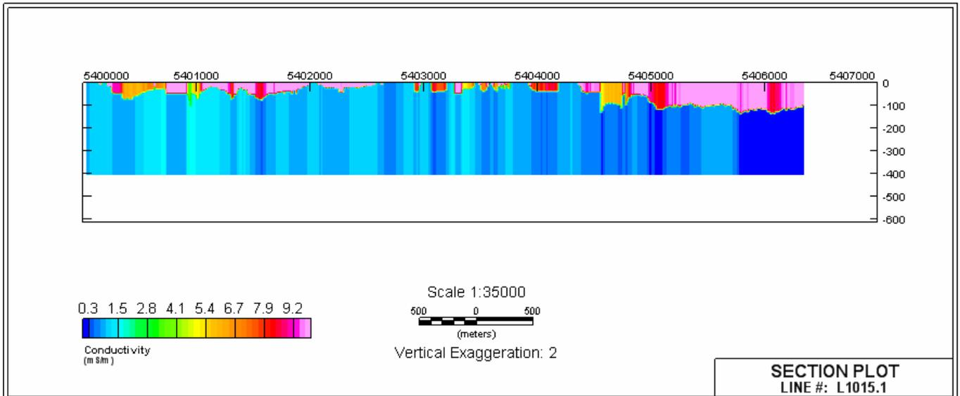
Figure 4: Two-layer inversion over line 15 at Reid Mahaffy with AIRBEO.
