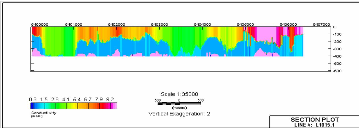
Figure 8: Three-layer inversion of line 15 with an initial model of 10 mS/m, 50 m, over 1 mS/m, 50 m, and a half-space of 1 S/m.
