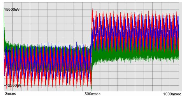
Figure 3: Raw signal from Atlantis fluxgate probe from A (red), U(blue) and V(green) component data.
