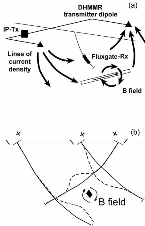
Figure 2: Sign conventions for DHMMR surveys.
