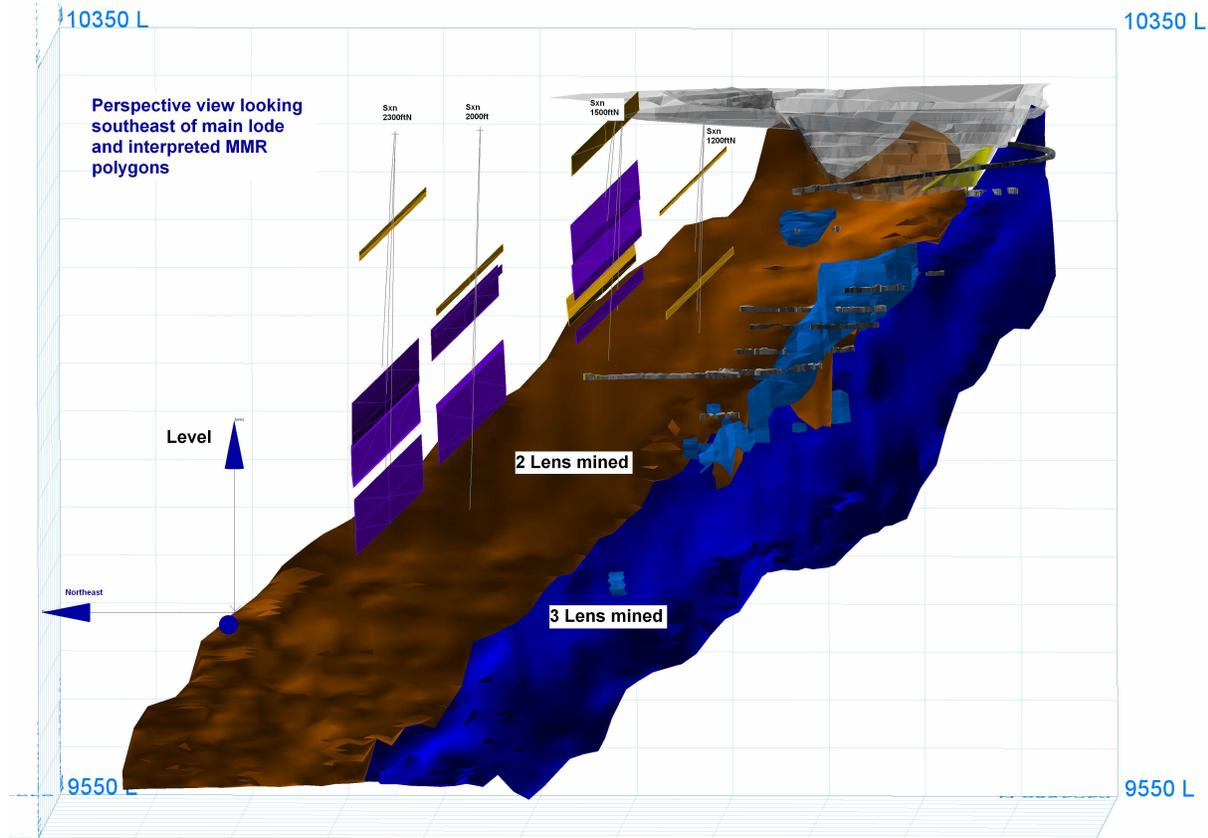
**Figure 5:** Perspective view looking south east of 3D DHMMR polygons and drill hole traces with 3-Lens and 2-Lens orebodies.
