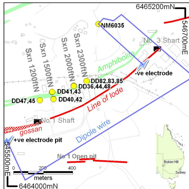
Figure 1: Location and survey setup for the North Mine DHMMR program.
