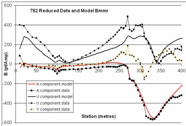
**Figure 4:** Hole 782 data and model Bmmr for A+U components, and Bmmr for V-component.
