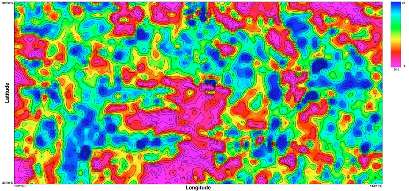
Figure 4: Calculated depth to the magnetic interface of the study area.
