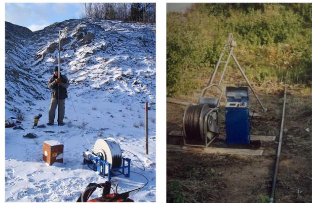
**Figure 3:** Photos of typical BHEM setups at the borehole collar. On the left is the setup of the Geonics BH-43-3 BHEM system with the assembled down-hole string held vertically out of the hole and winch. The receiver is in the foreground. On the right is shown the BHUTEM4 system comprising the winch system, receiver and the assembled probe string lying on the ground.
