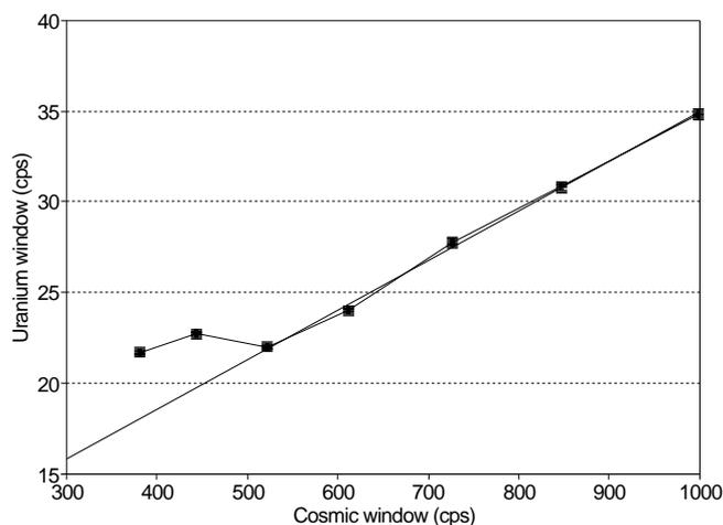
**Figure 1:** The variation of the uranium and cosmic windows showing the effects of radon at the lower elevations.
