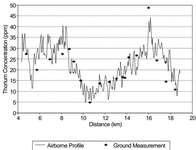
**Figure 4:** The relationship between the thorium ground concentration and the calibrated airborne measurements in Malaysia.
