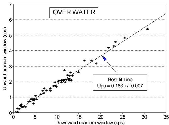
**Figure 2:** Calibration of the upward detector from flights over water.
