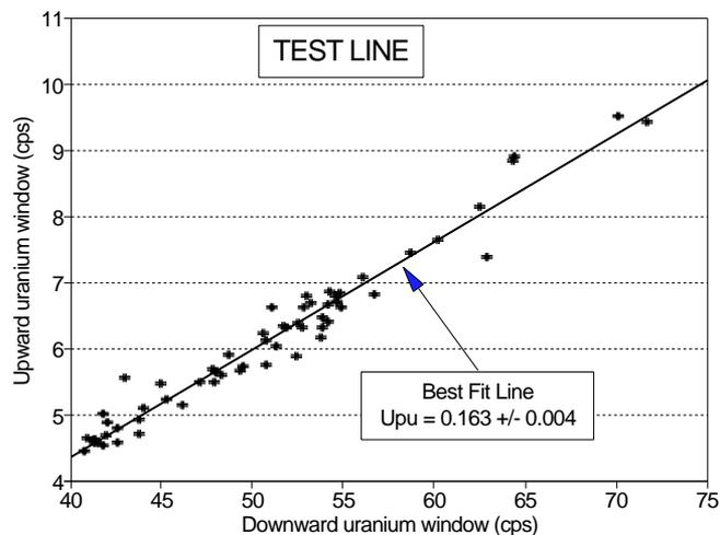
**Figure 3:** Calibration of the upward detector from flights over a test line.
