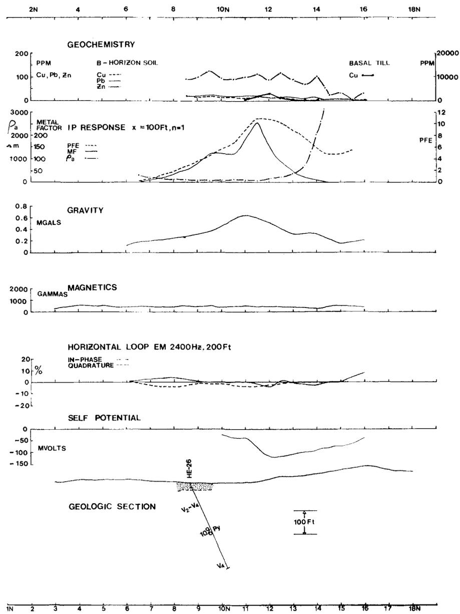
Figure 27.34. Geochemical and geophysical profiles and section, Line 4+00E, New Inasco Orebody.
