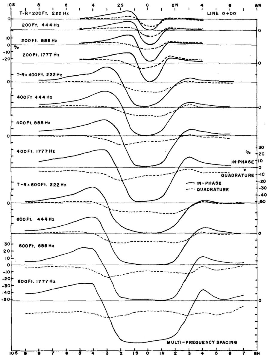
Figure 27.24. Horizontal-loop EM profiles, multifrequency-spacing, Line 0+00, Iso Orebody.
