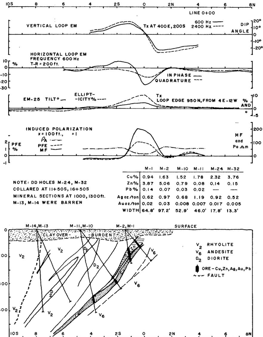
Figure 27.20. Geophysical profiles and section, Line 0+00, Iso Orebody.
