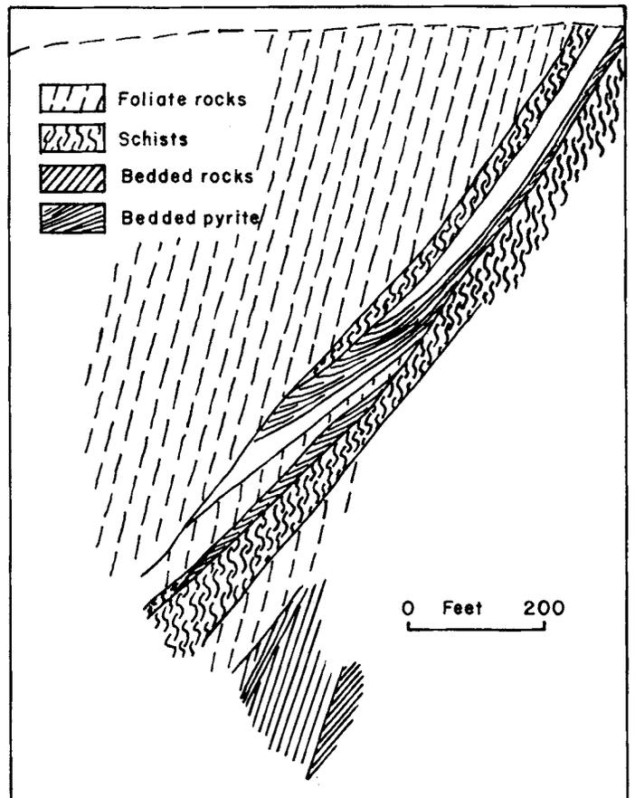
Figure 27.8. Fine layer and structure section, Line 2+00E, Iso Orebody.
