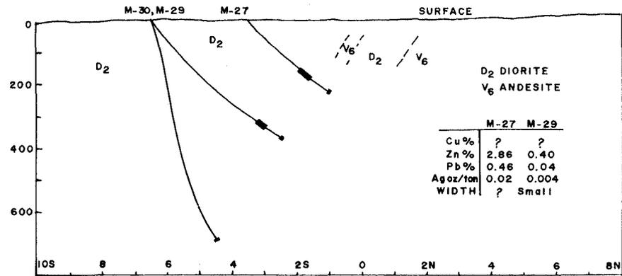
Figure 27.23. Geophysical profiles and section, Line 8+00E, Iso Orebody.
