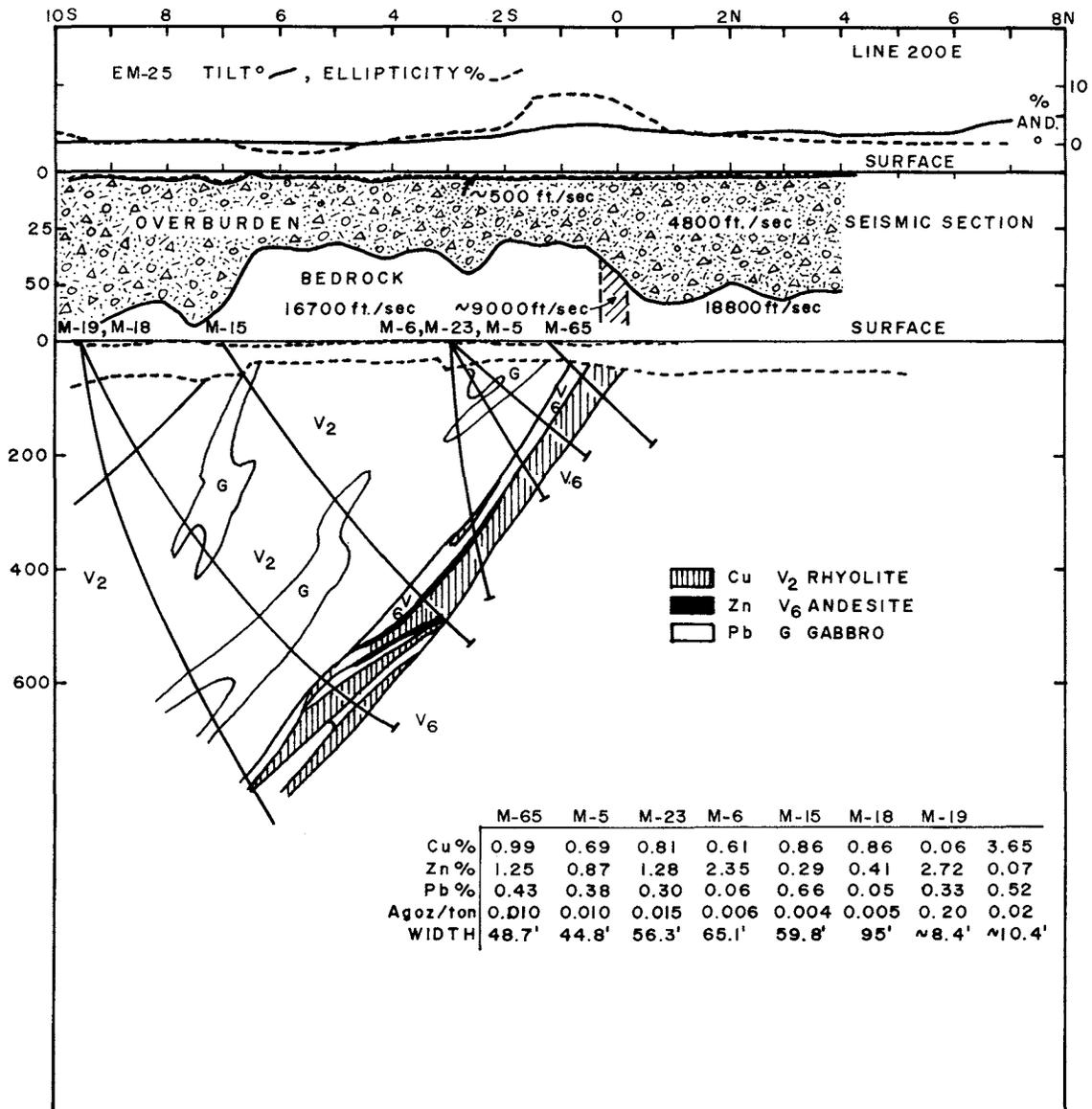
Figure 27.21. EM-25, seismic data and section, Line 2+00E, Iso Orebody.
