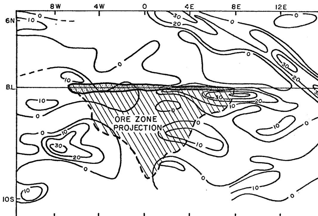
Figure 27.12. VLF-EM contours; contours in degrees tilt angle, Iso Orebody.
