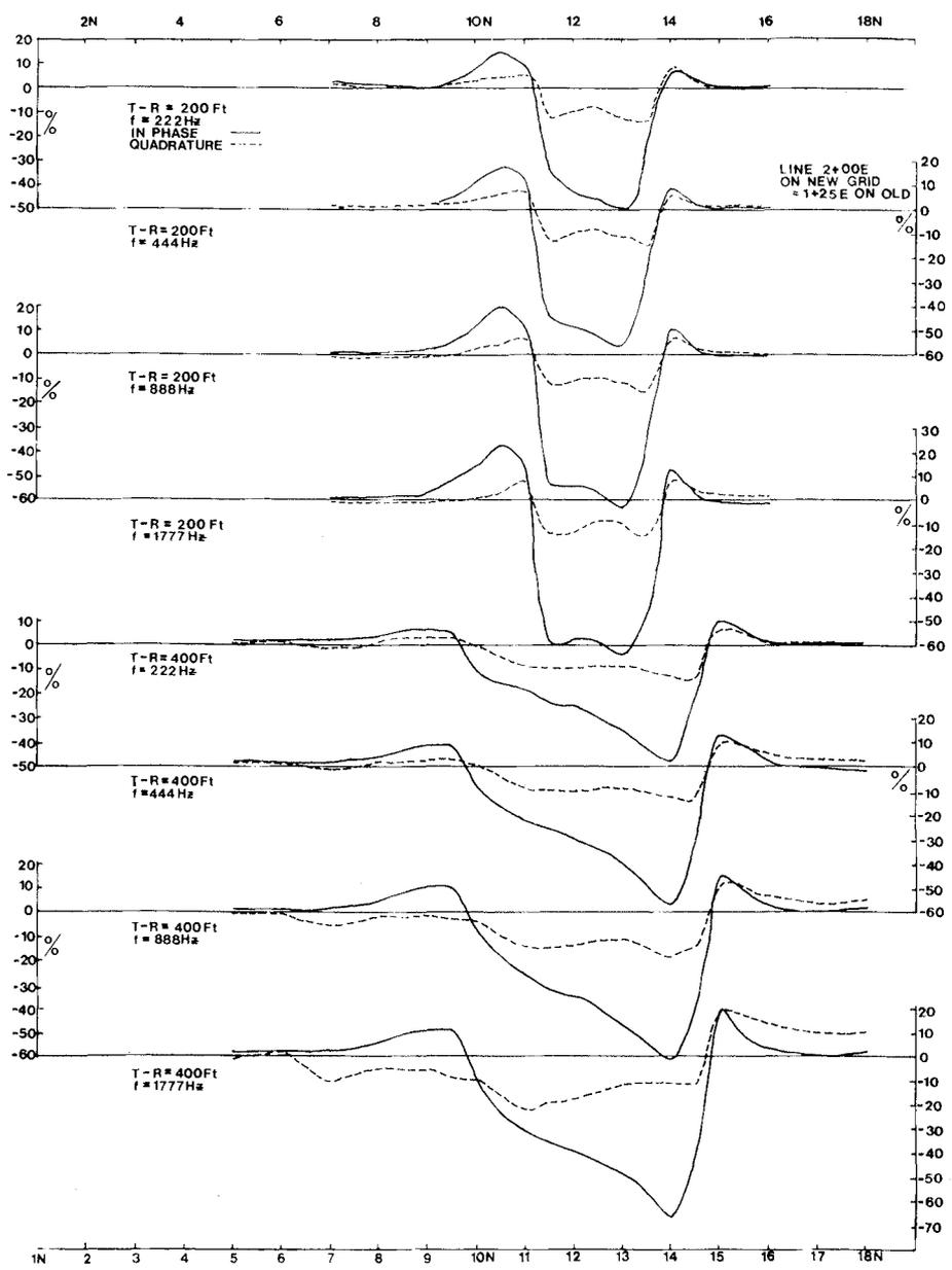
Figure 27.35. Horizontal-loop EM profiles, multifrequency-spacing, Line 1+25E, New InSCO Orebody.
