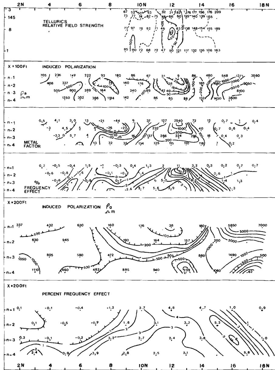
Figure 27.38. IP and telluric pseudo-depth sections, Line 2+00E, New InscO Orebody.
