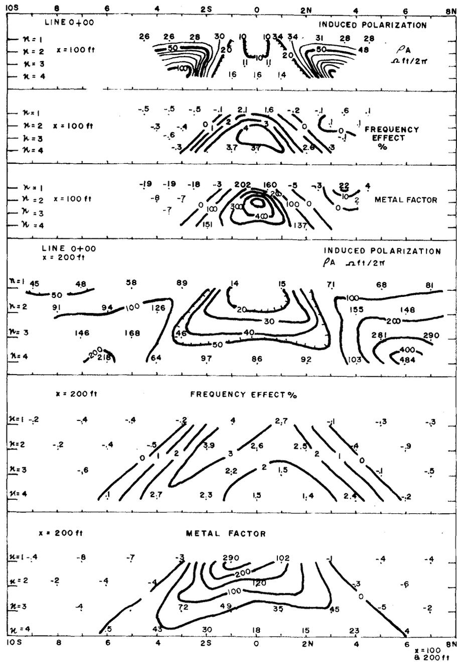
Figure 27.25. IP pseudo-depth plots, Line 0+00, double-dipole spread, Iso Orebody.
