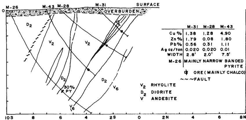
Figure 27.22. Geophysical profiles and section, Line 4+00E, Iso Orebody.
