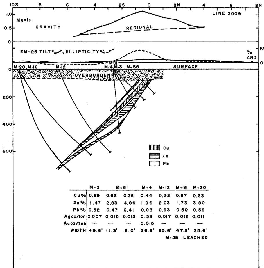
Figure 27.19. Gravity, EM-25 profiles and section, Line 2+00W, Iso Orebody.
