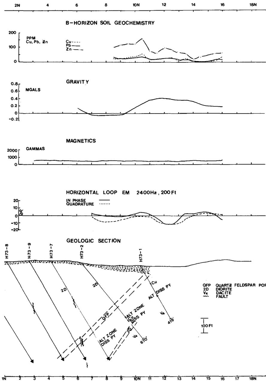
Figure 27.29. Various geochemical and geophysical profiles and section, Line 0+00, New InscO Orebody.
