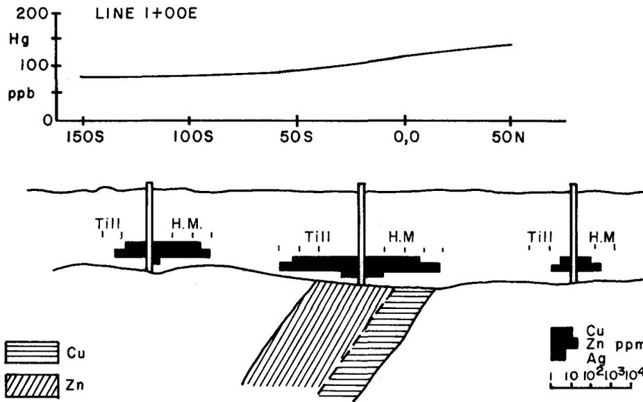
Figure 27.9. Soil and basal-till geochemistry, line 1+00E, Iso Orebody.
