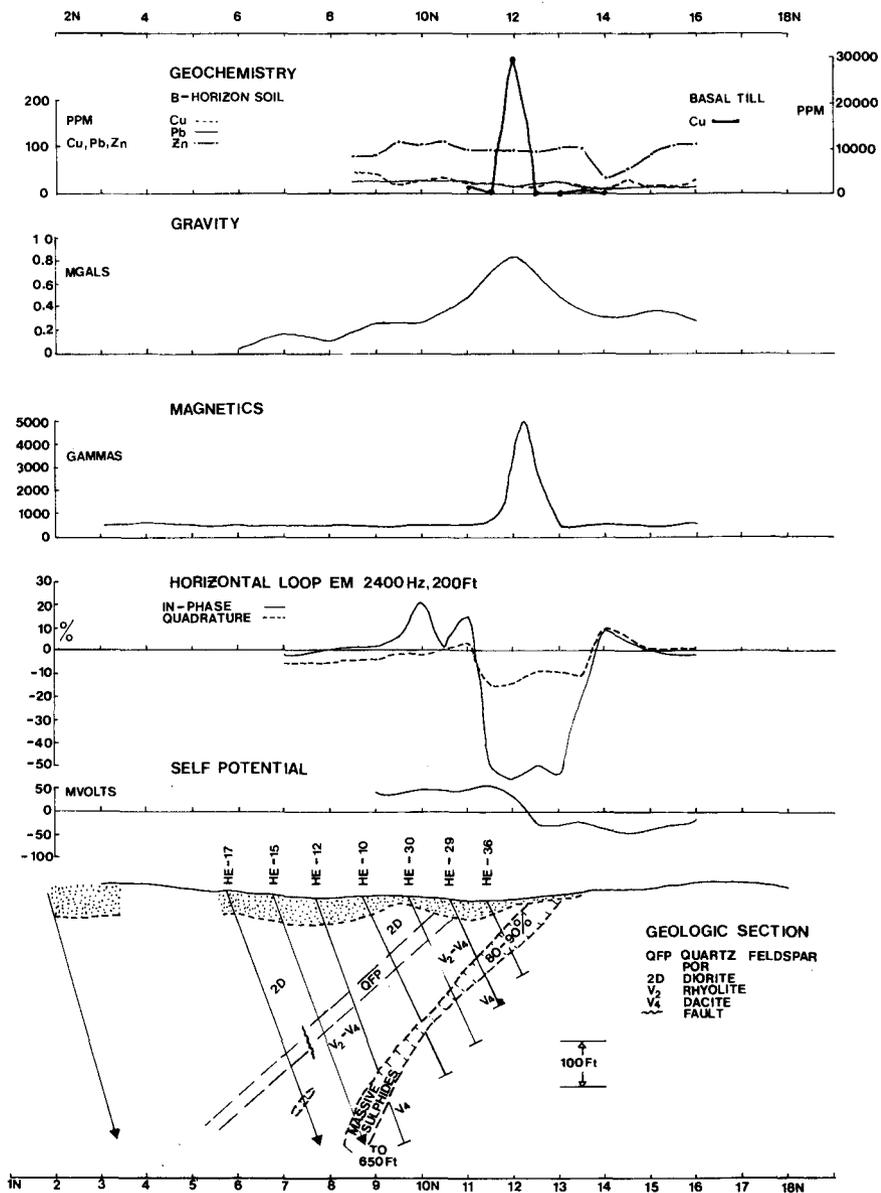
Figure 27.30. Various geochemical and geophysical profiles and section, Line 1+00E, New InscO Orebody.
