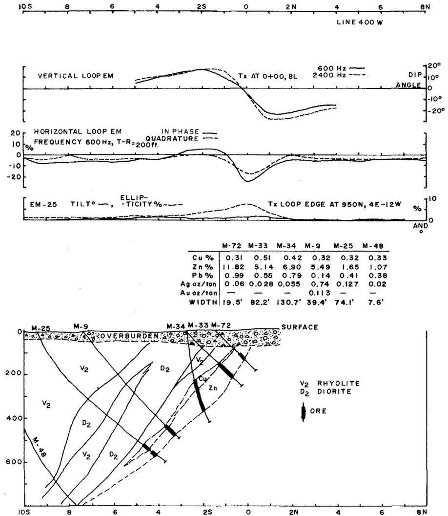
Figure 27.18. Geophysical profiles and section, Line 4+00W, Iso Orebody.
