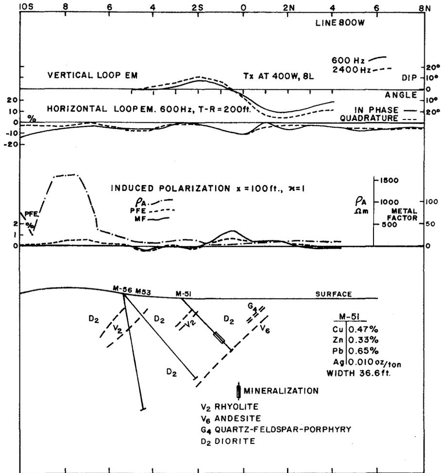
Figure 27.17. Various geophysical profiles and section, Line 8+00W, Iso Orebody.
