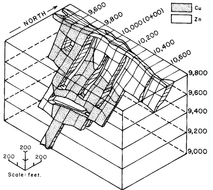
Figure 27.7. Isometric view of Iso Orebody.
