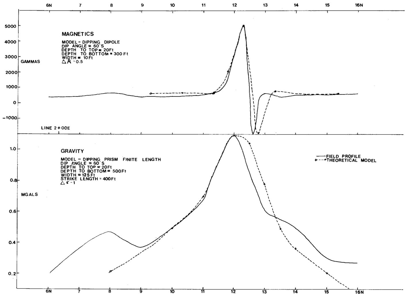
Figure 27.32. Matching of magnetic and gravity profiles by model shapes, Line 2+00E, New InscO Orebody.
