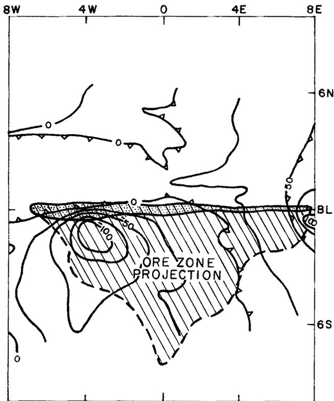
Figure 27.14. Self potential contours; contour interval 25 mV, Iso Orebody.
