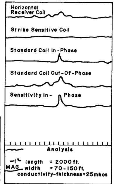
Figure 27.11. Dighem data, flight record profile, Iso Orebody.
