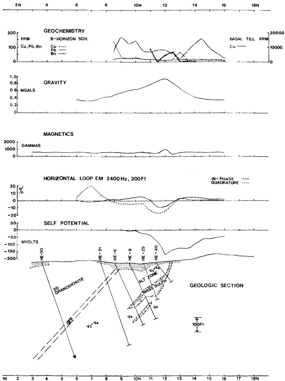
Figure 27.33. Geochemical and geophysical profiles and section, Line 3+00E, New Inasco Orebody.
