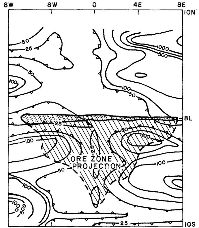
Figure 27.15. EM16R contours; contours of  $\rho_a \Omega m$ .  $f = 18.6$  kHz, Iso Orebody.
