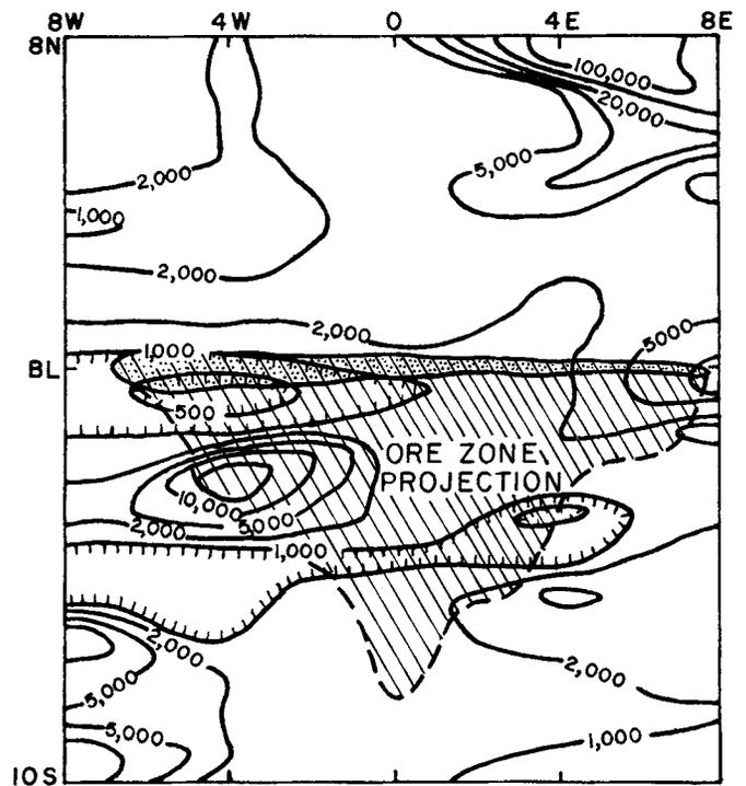
Figure 27.16. Magnetotelluric contours; contours of  $\rho_a \Omega m$ .  $f = 250$  Hz, Iso Orebody.
