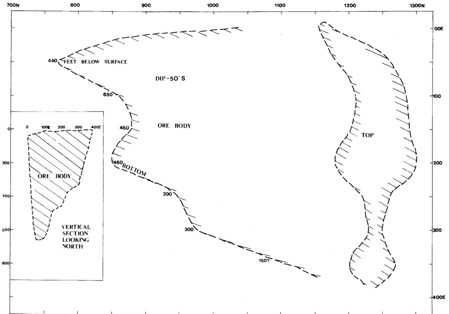
Figure 27.28. Surface projection and vertical section, New Insko Orebody.
