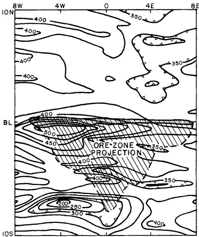
Figure 27.13. Vertical field magnetic contours; contour interval 25 gammas, Iso Orebody.
