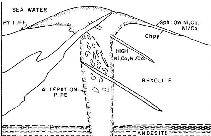
Figure 27.6. Idealized section of Noranda-type deposit (Vauze, Norbec, etc.).
