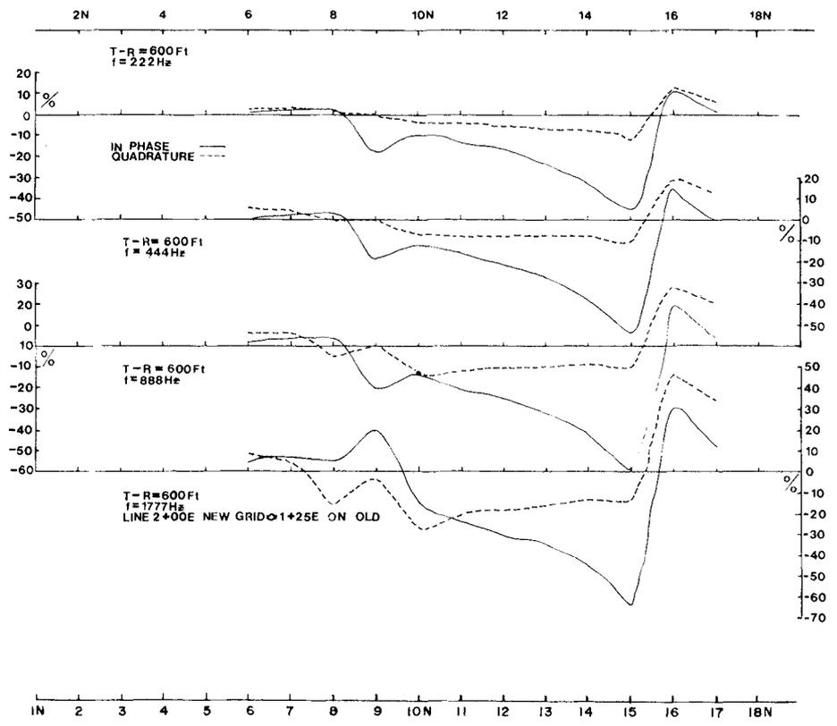
Figure 27.36. Horizontal-loop EM profiles, multifrequency-spacing, Line 1+25E, New InSCO Orebody.
