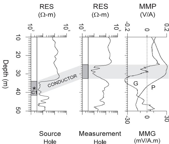
Figure 2: Field example showing the use of mise-à-la-masse potential (MMP) and potential (MMG) gradient measurements to establish continuity of conductive zones between boreholes. RES = resistivity, P = potential; G = gradient.
