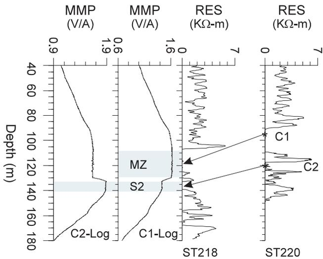
**Figure 13:** *Mise-à-la-masse* measurements acquired in ST218 with current sources in ST220. The C1- and C2-Logs represent potential-depth profiles with electrodes at C1 and C2, respectively.
