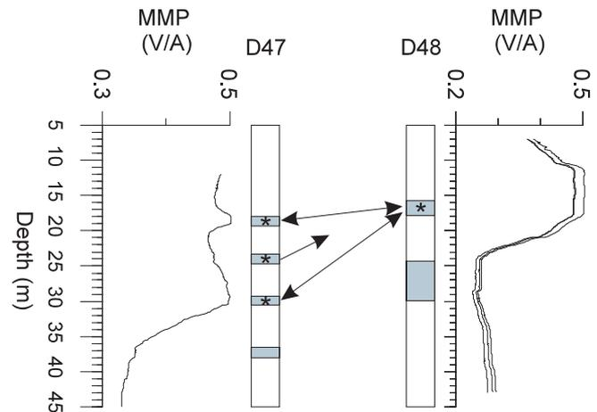
**Figure 5:** *Mise-à-la-masse* data acquired between D47 and D48, illustrating a more complex problem. The potential responses in D48 for current sources at three graphite intersections in D47, are virtually the same. Reciprocal measurements show that, of the three energised graphite intersections, two of them are in electrical continuity with the upper zone in D48.
