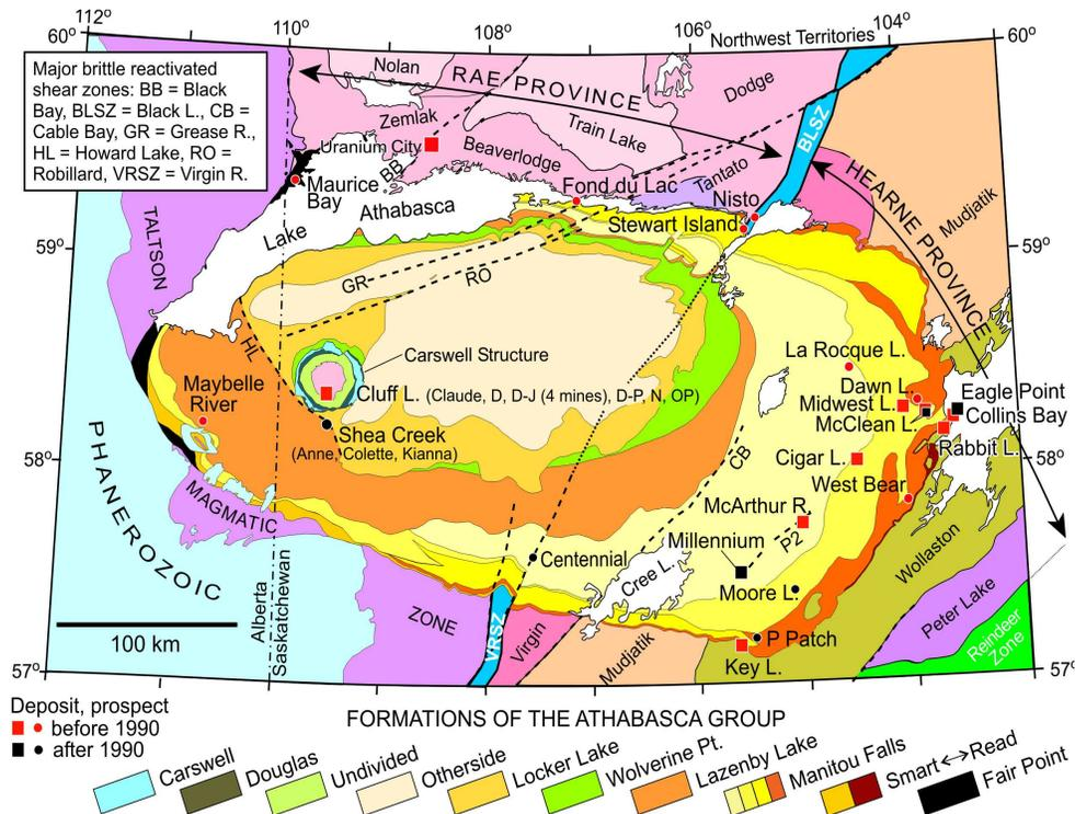
**Figure 2:** Geological setting and unconformity-associated U occurrences of the Athabasca Basin region of northwestern Canada (Figure 1). Heavy dashed lines are selected major reactivated fault zones. Basement geology is after Portella and Annesley (2000a), Thomas et al. (2002), Card (2006), and Card et al. (2003, 2007a, b). Athabasca Basin geology is after Ramaekers et al. (2007).
