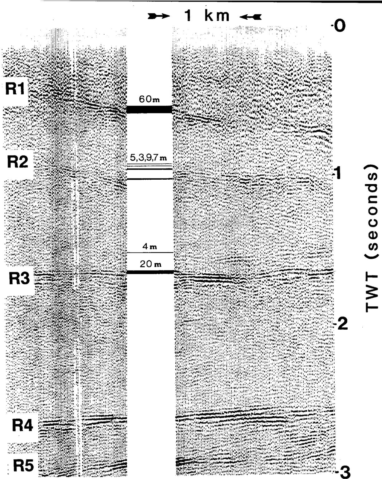
**Figure 2:** Part of the stacked section from lines 5 and 7 (Juhlin, 1990) over the Gravberg-1 borehole in the Siljan impact structure. Dolerite sills with their respective thickness (greater than 3 m thick) are marked on the section.
