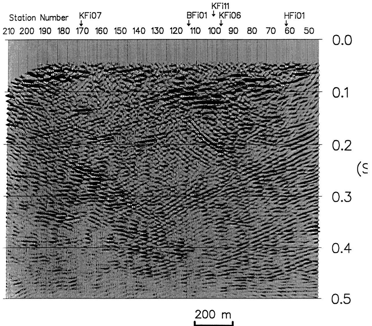
**Figure 3:** Migrated section from the Finnsjön area. The subhorizontal event at about 0.1 s is an hydraulically conductive fracture zone as determined from surface boreholes (locations marked with arrows).
