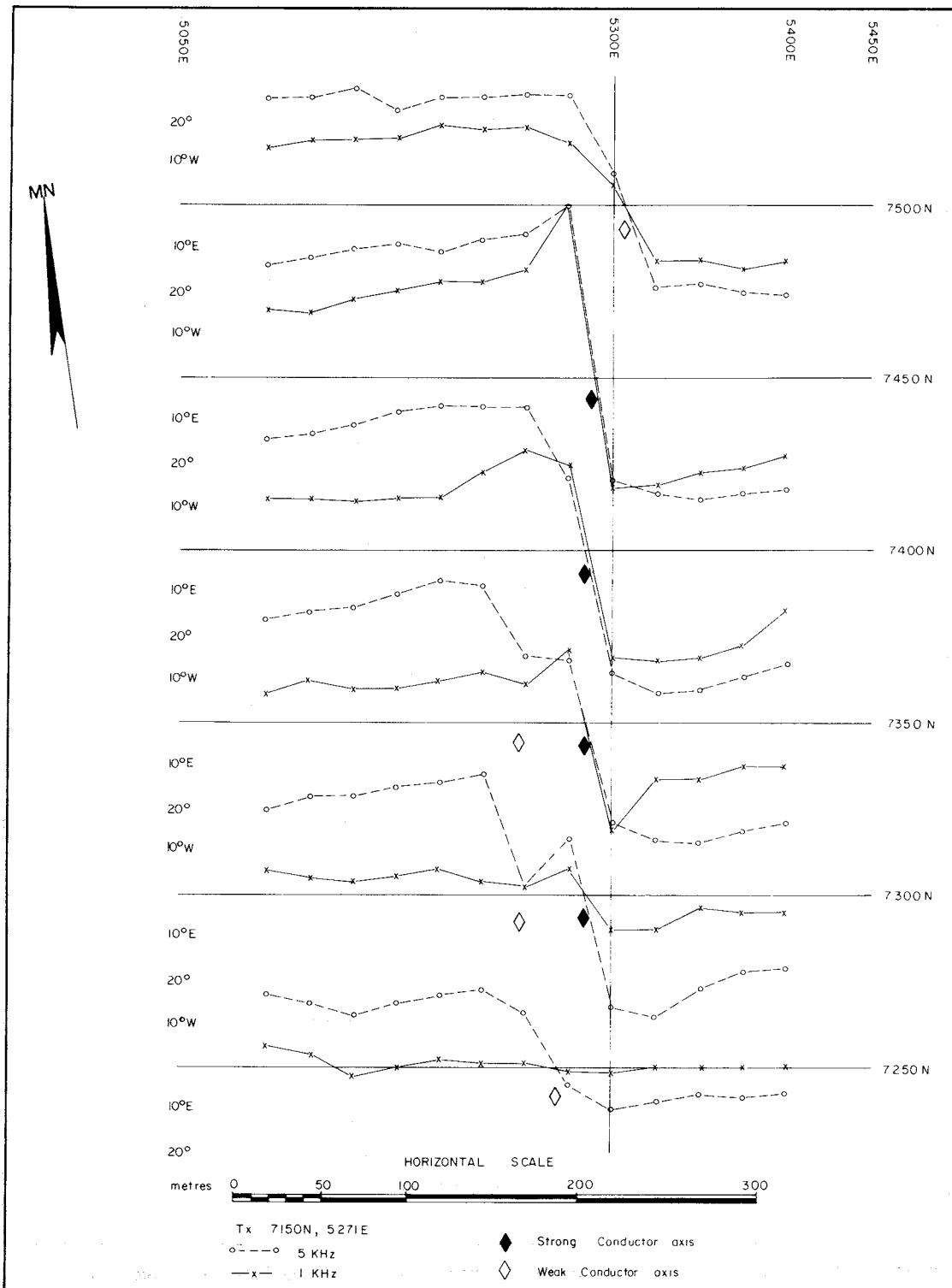
**Figure 33.19.** Vertical-loop electromagnetic profiles obtained using the McPhar SS15 system. Transmitter located at 7150N, 5270E. Que River Prospect, Tasmania.
