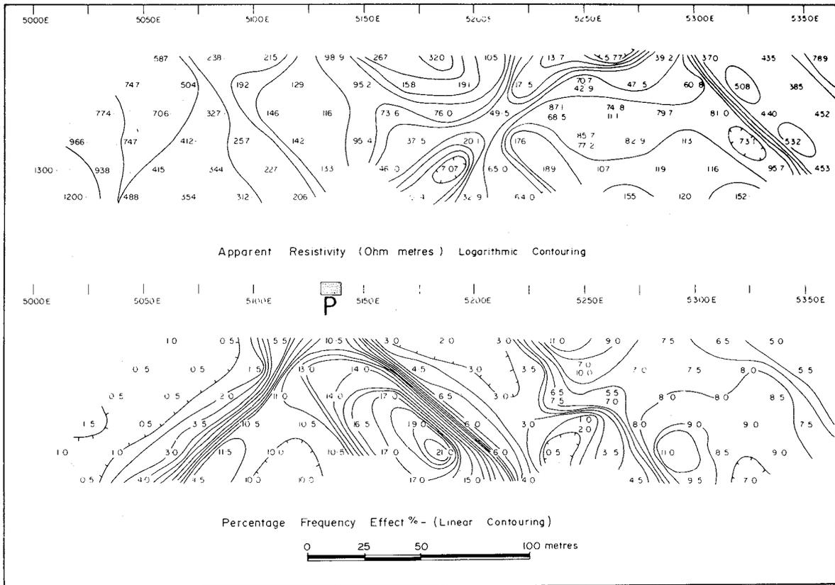
Figure 33.22a. Resistivity and frequency domain IP results along Line 7250N using a dipole-dipole array. Frequencies used ranged from 0.3 to 2.5 Hz. Que River Prospect, Tasmania.
