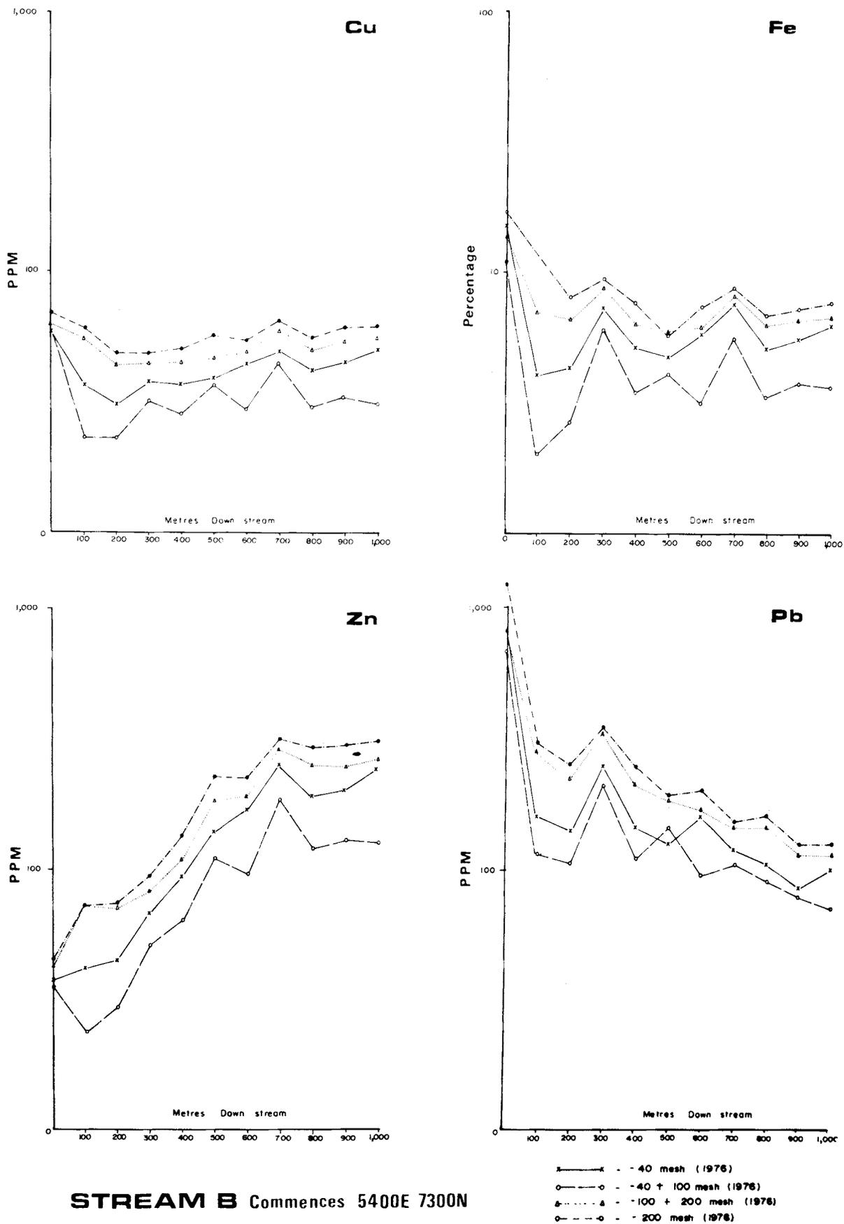
Figure 33.7. Stream sediment geochemical results for Cu, Fe, Zn, and Pb from Stream B. Que River Prospect, Tasmania.
