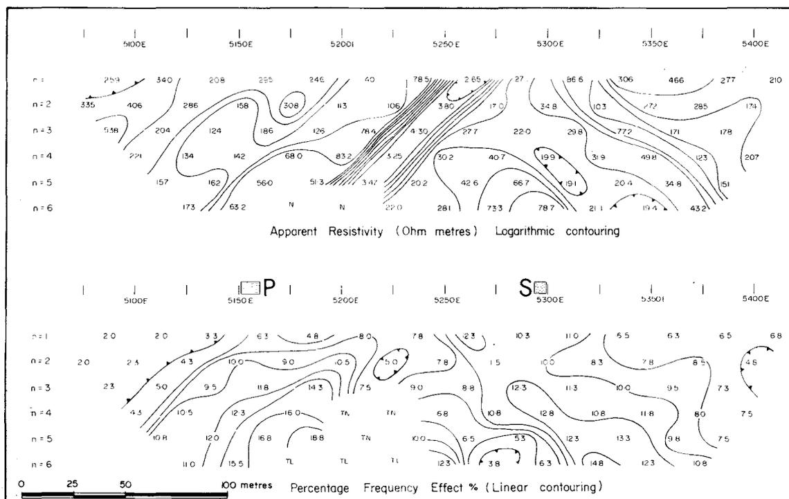
Figure 33.23. Resistivity and frequency-domain IP results along Line 7350N obtained using a 25 m dipole-dipole array. Frequencies used ranged from 0.3 to 2.5 Hz. TN and TL indicates that readings were either too noisy or the voltage was too low for measurement. Que River Prospect, Tasmania.
