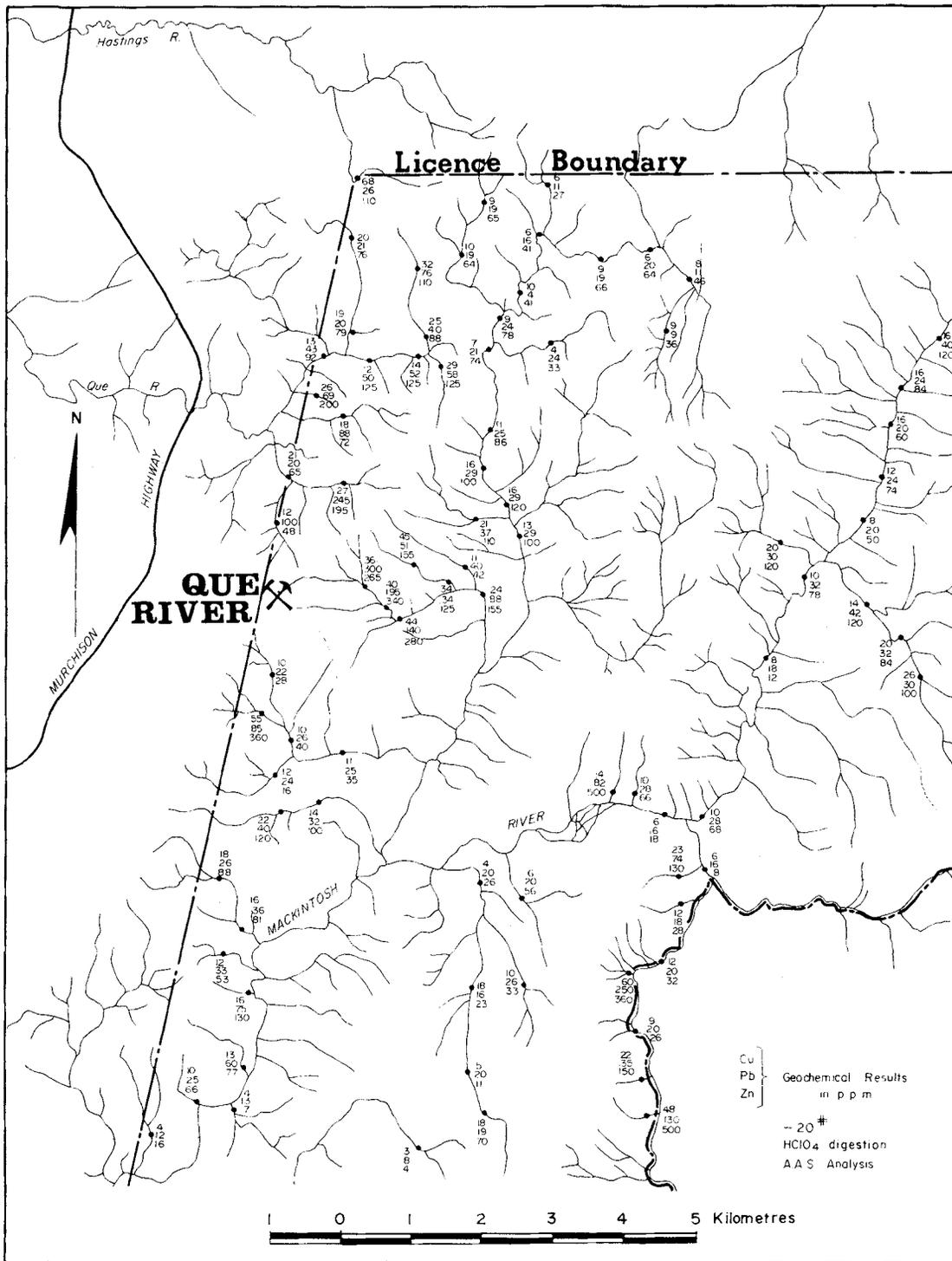
Figure 33.5. Geochemical results for the 1970-71 stream sediment survey, Que River Prospect, Tasmania.
