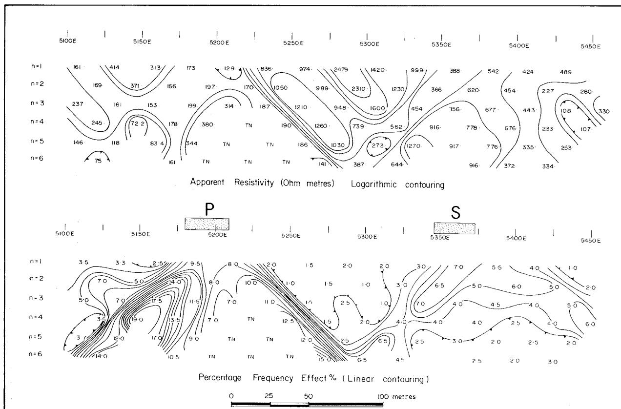
**Figure 33.22b.** Resistivity and frequency-domain IP results along Line 7800N. Frequencies used range from 0.3 to 2.5 Hz. Que River Prospect, Tasmania.
