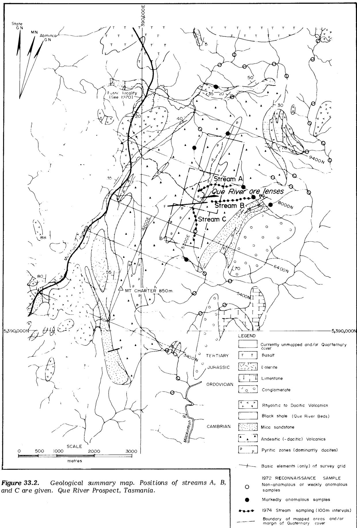
Figure 33.2. Geological summary map. Positions of streams A, B, and C are given. Que River Prospect, Tasmania.
