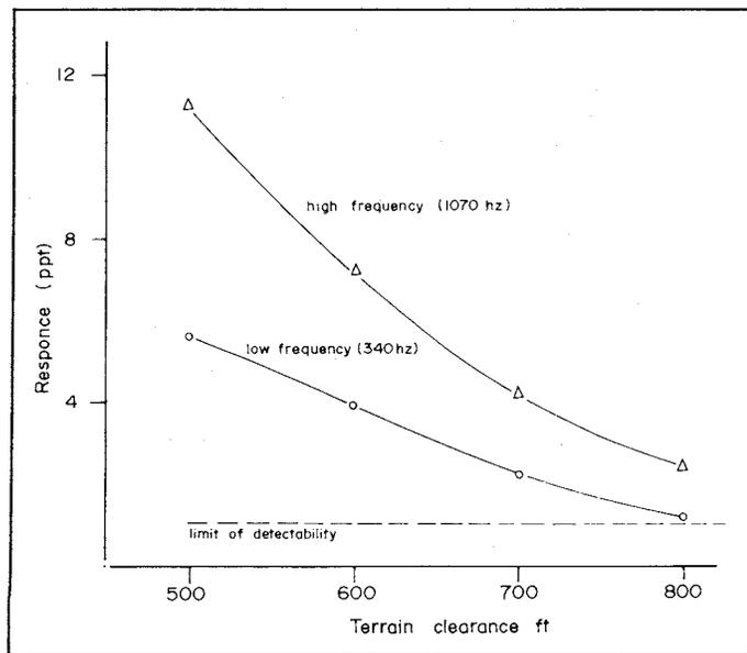
Figure 33.16. Attenuation tests over the Que River anomaly using the McPhar H-400 airborne EM system flown by Geox Pty Ltd. in 1975.
