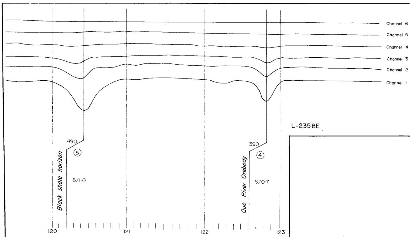
**Figure 33.17.** INPUT airborne EM profiles across the Que River Prospect, Tasmania.
