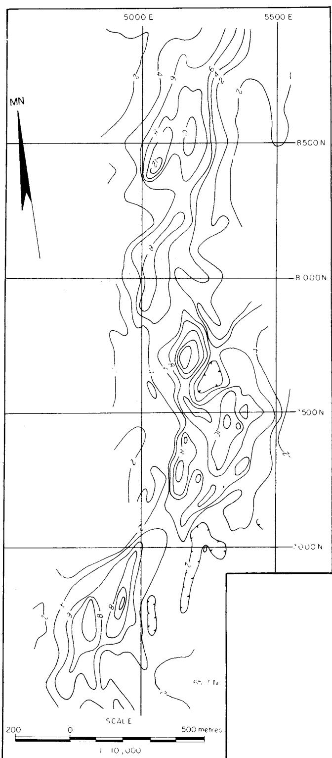
**Figure 33.26.** Average percentage frequency effect (PFE) map. Contour interval 2%. Que River Prospect, Tasmania.
