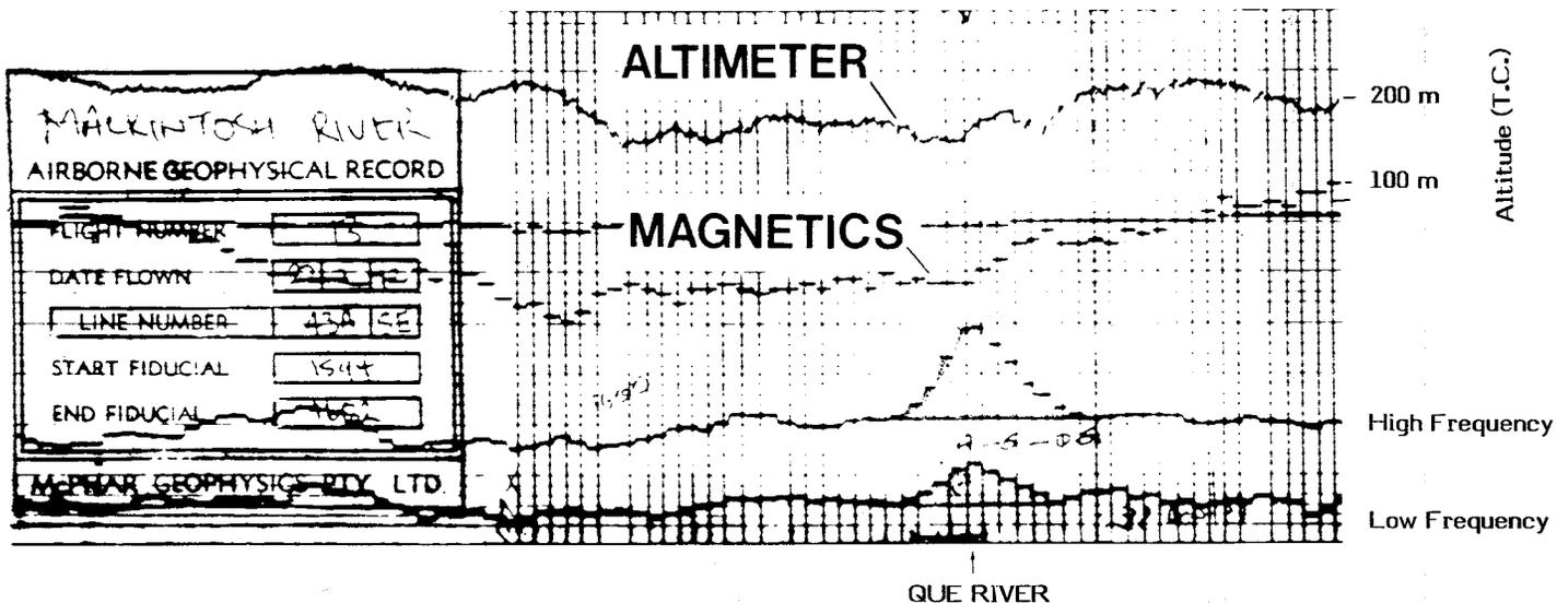
Figure 33.14. Airborne electromagnetic discovery profile across the Que River Prospect using the McPhar H400 two-frequency quadrature system (1972).
