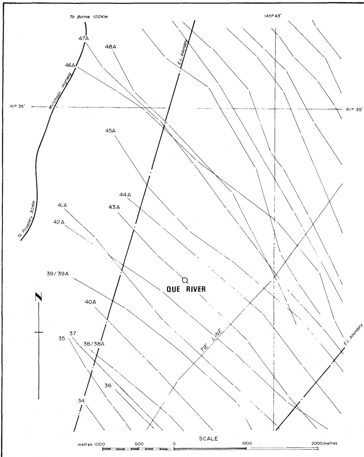
**Figure 33.15.** Flight path map for the 1972 airborne EM survey by McPhar Geophysics Pty. Ltd. Que River Prospect, Tasmania.
