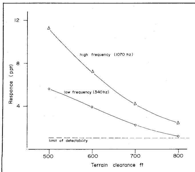
**Figure 33.16.** Attenuation tests over the Que River anomaly using the McPhar H-400 airborne EM system flown by Geoex Pty Ltd. in 1975.
