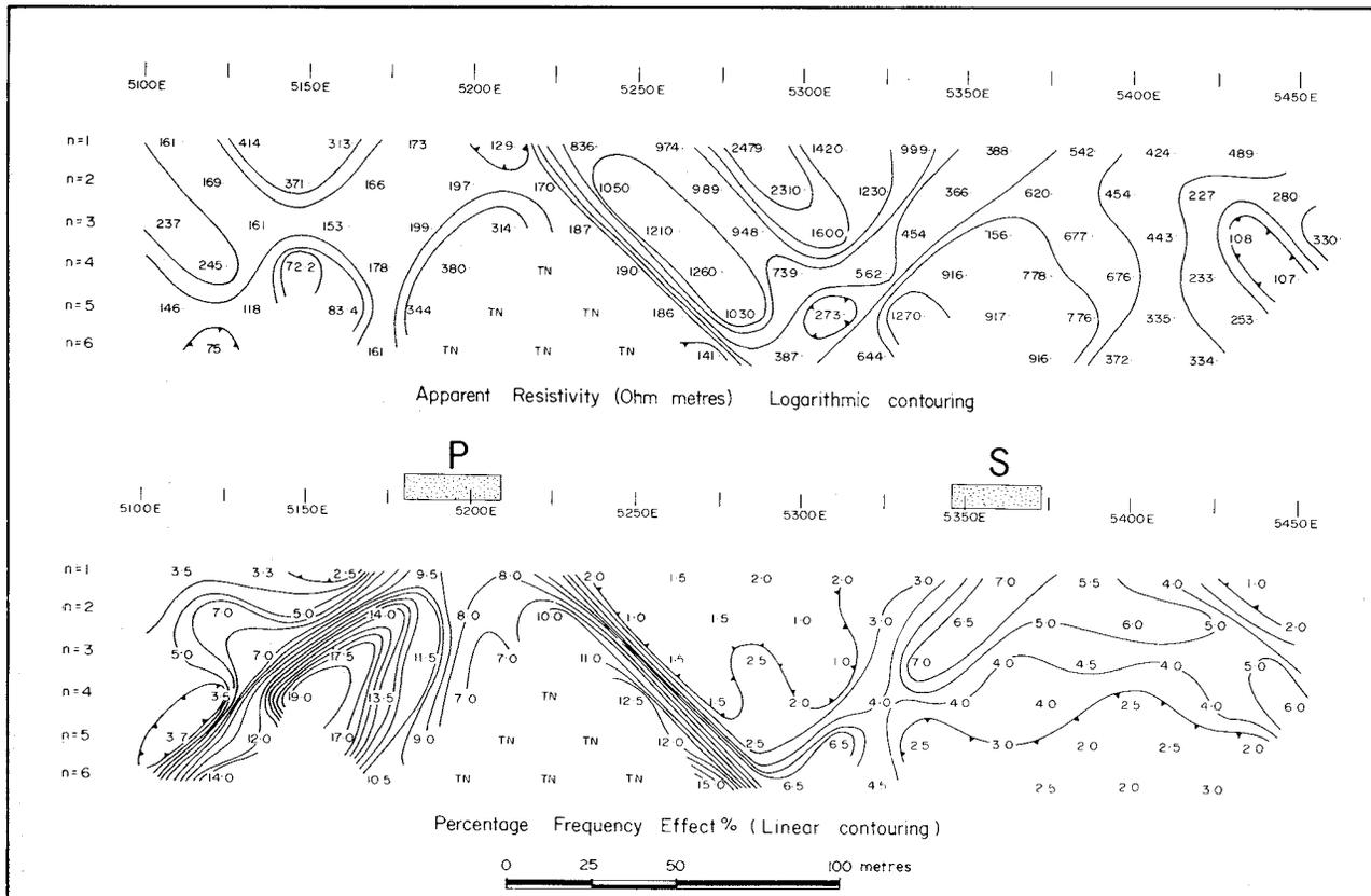
Figure 33.22b. Resistivity and frequency-domain IP results along Line 7800N. Frequencies used range from 0.3 to 2.5 Hz. Que River Prospect, Tasmania.
