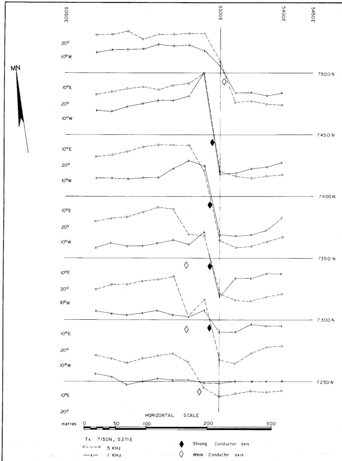
Figure 33.19. Vertical-loop electromagnetic profiles obtained using the McPhar SS15 system. Transmitter located at 7150N, 5271E. Que River Prospect, Tasmania.
