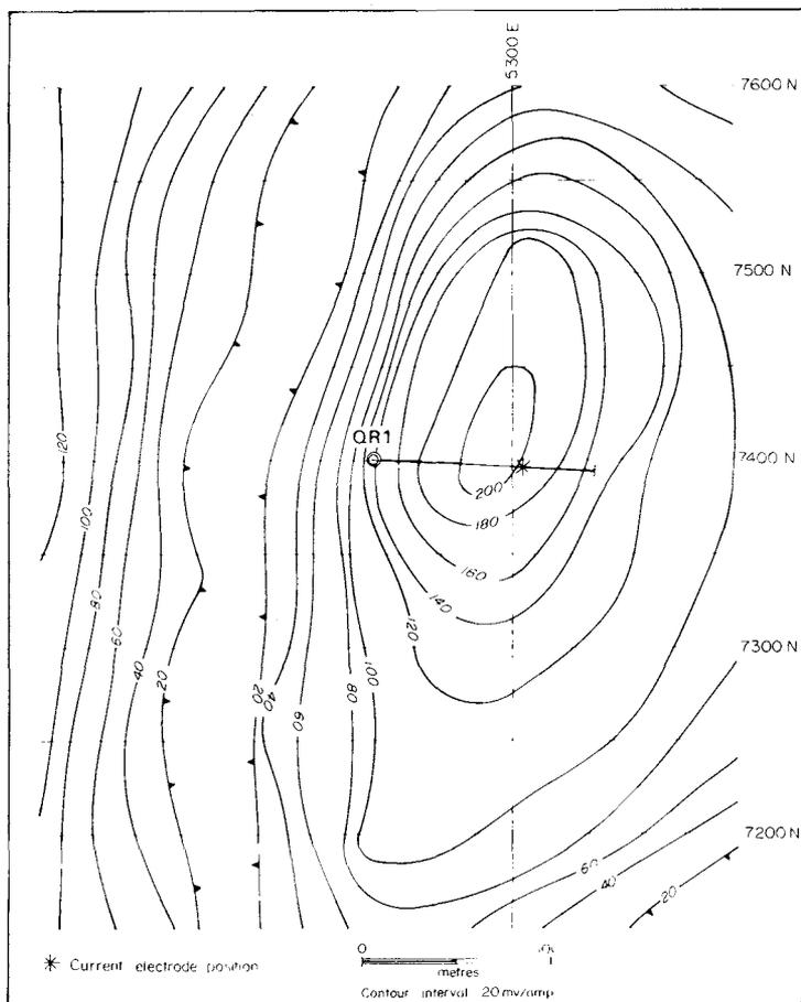
Figure 33.24. Mise-à-la-masse map survey results using a current electrode located in the eastern mineralization in drillhole QR1. Que River Prospect, Tasmania.
