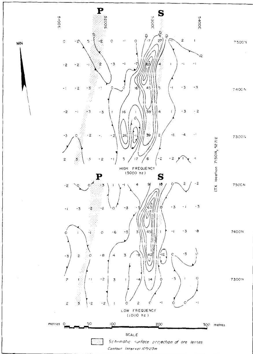
Figure 33.20. First horizontal derivative map of vertical-loop EM data obtained using Fraser (1969) procedure. Contour interval 10<sup>0</sup>/25 m. Que River Prospect, Tasmania.
