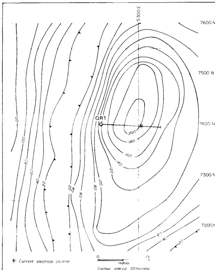
**Figure 33.24.** Mise-à-la-masse map survey results using a current electrode located in the eastern mineralization in drillhole QR1. Que River Prospect, Tasmania.
