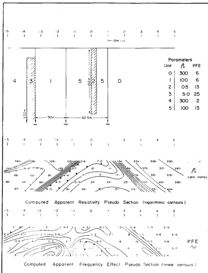
Figure 33.25. Model results derived from the dipole-dipole array IP results along Line 7350N.
