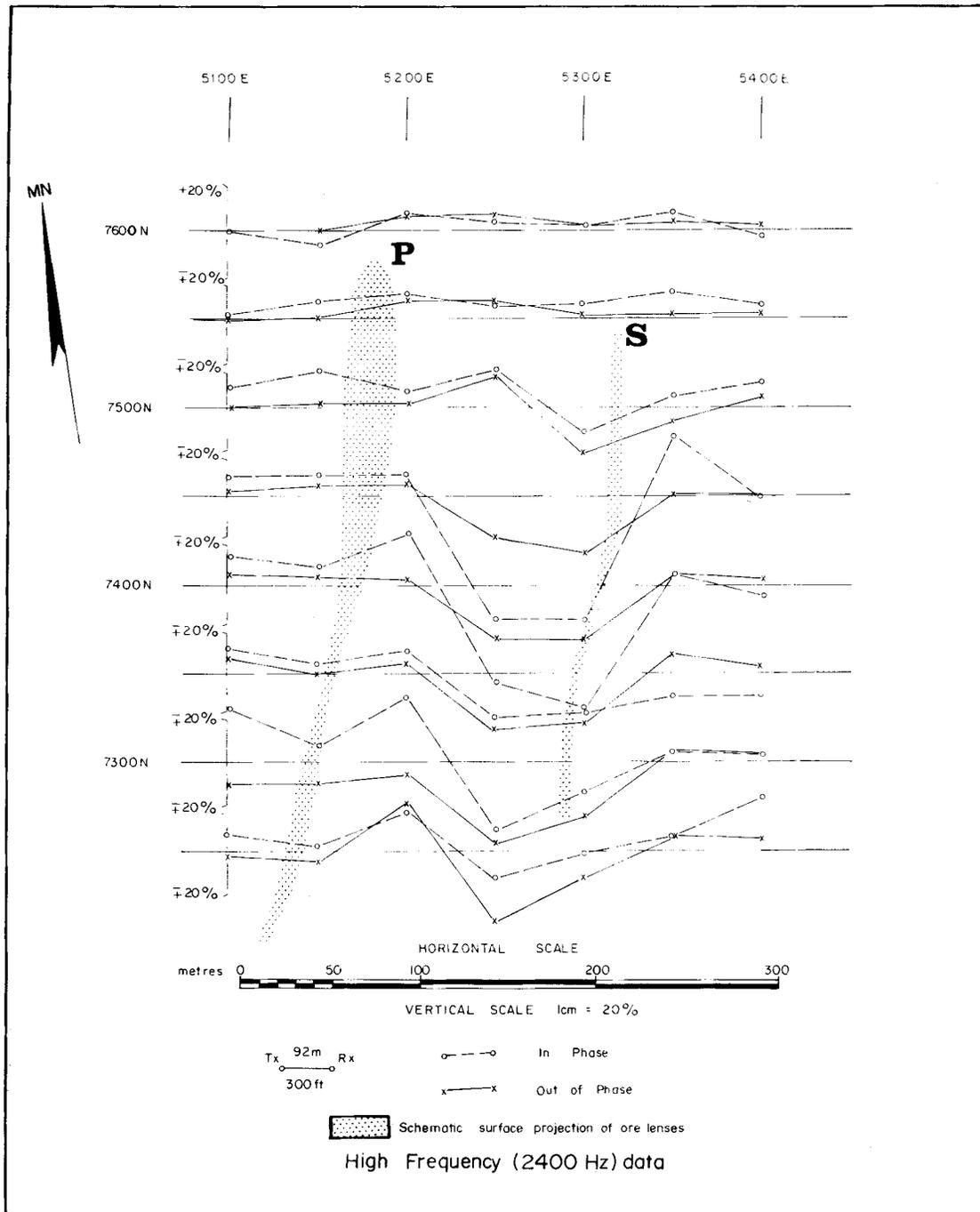
**Figure 33.18.** Horizontal-loop electromagnetic profiles using McPhar VHEM equipment operating at 2400 Hz. Separation of transmitter/receiver was 92 metres. Que River Prospect, Tasmania.
