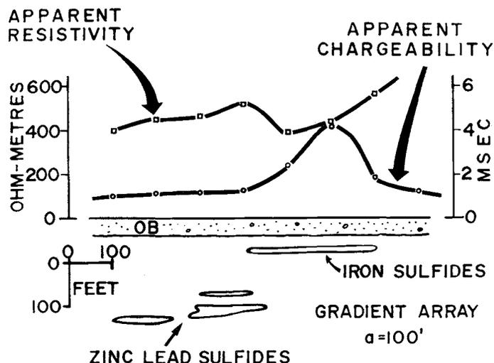
Figure 30.11. Example of an indirect discovery using time-domain IP on line M (Huntec MK-1) showing apparent resistivity and chargeability profiles. OB is overburden.
