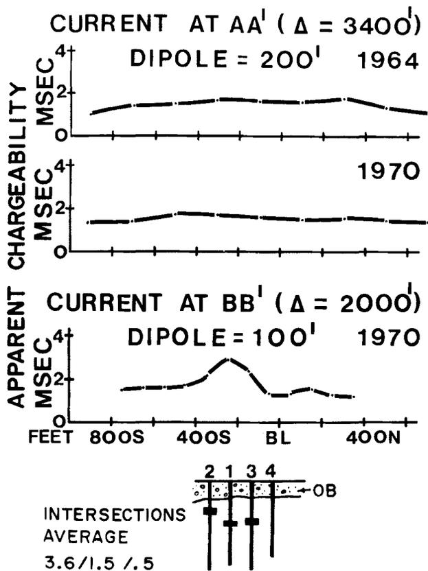
**Figure 30.9.** Gradient-array IP profiles obtained in 1964 and 1970 on line P (Huntec MK 1).  $\Delta$  is the current electrode separation. Grade is in per cent Pb, Zn, and Fe.
