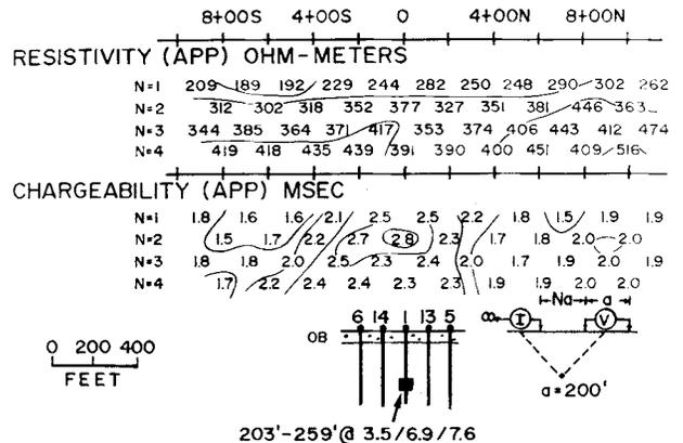
Figure 30.21. Time-domain IP-resistivity data on line L over deep and localized mineralized intersection (Huntec MK 3). Grade is in per cent Pb, Zn, and Fe.
