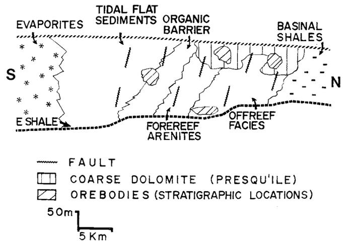
**Figure 30.3.** Simplified geological cross-section of barrier complex. Note the exaggerated vertical scale.
