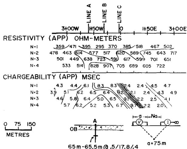
Figure 30.13. IP-resistivity data obtained on baseline of orebody R using pole-dipole array (Huntec MK 3). Grade is in per cent Pb, Zn, and Fe.
