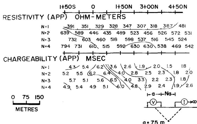
Figure 30.14. IP-resistivity data obtained on line A of orebody R (Huntec MK 3).
