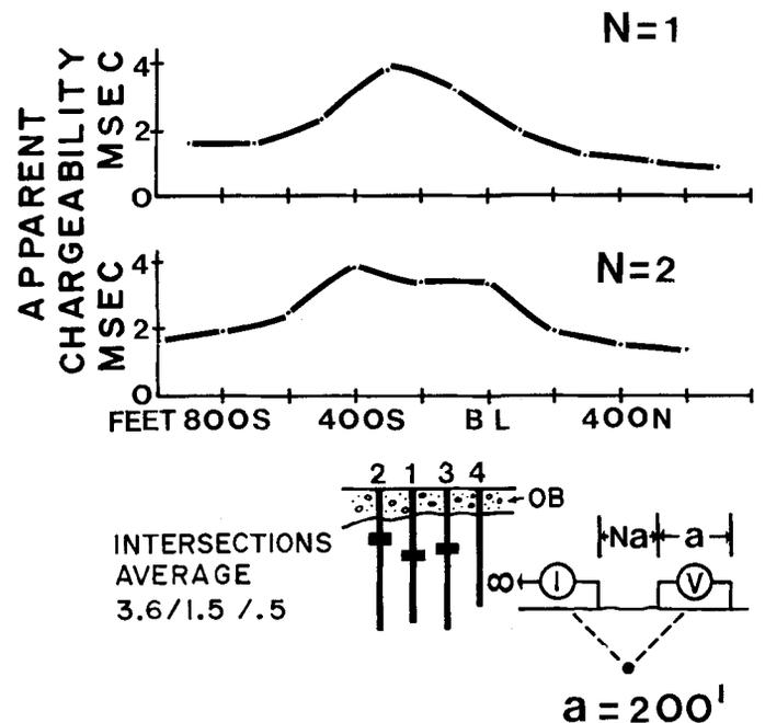
**Figure 30.10.** Pole-dipole array IP profiles on line P (Huntec MK 1). Grade is in per cent Pb, Zn, and Fe.
