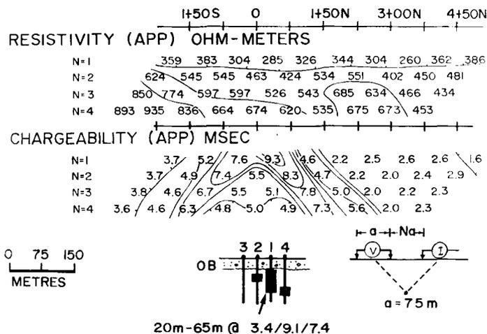
Figure 30.16. IP-resistivity data obtained on line B of orebody R (Huntec MK 3). Grade is in per cent Pb, Zn, and Fe.
