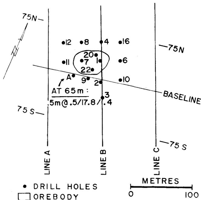
Figure 30.12. Plan of orebody R, drillholes, and IP lines.
