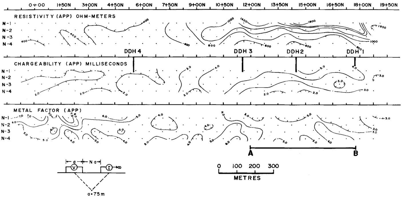
Figure 30.17. IP-resistivity data obtained on line N (Huntec MK 3).
