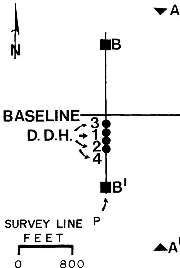
**Figure 30.8.** Plan of mineralized holes on line P and positions of current electrodes (AA' and BB') for gradient-array survey on line P.
