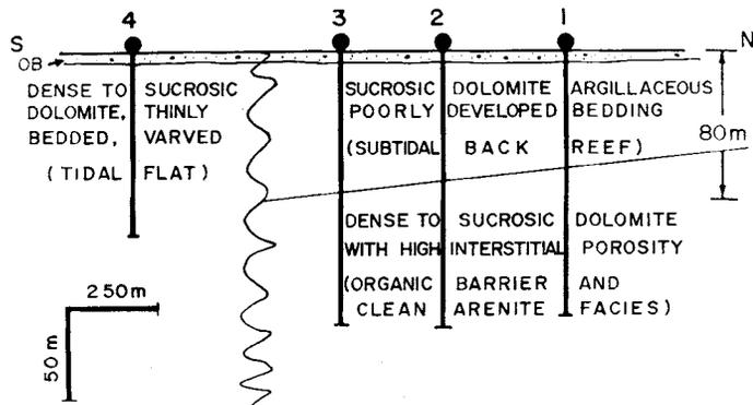
Figure 30.19. Geological cross-section of line N.
