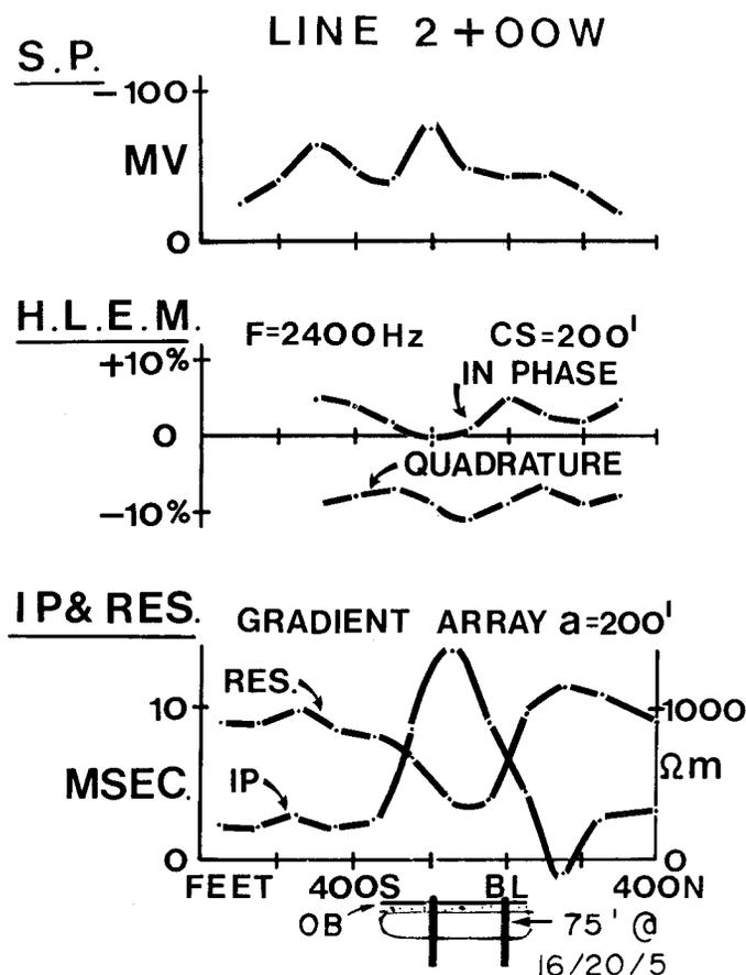
**Figure 30.5.** Geophysical test profiles over orebody N-42, line 2+00W, 1963 (Huntec MK 1). Ore grade is in per cent Pb, Zn, and Fe.
