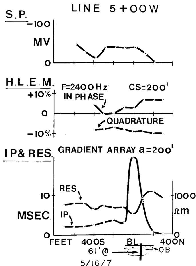
**Figure 30.6.** Geophysical test profiles over orebody N-42, line 5+00W, 1963 (Huntec MK 1). Ore grade is in per cent Pb, Zn, and Fe.
