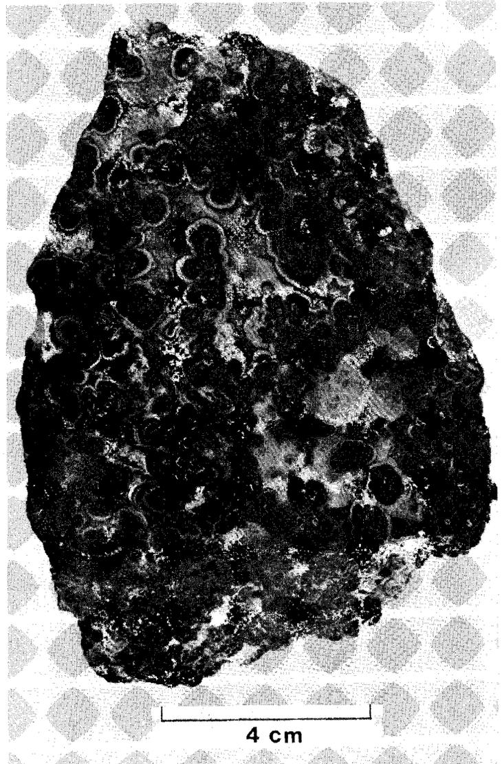
**Figure 30.4.** Sample of sphalerite and galena mineralization in a dolomite gangue. (GSC 203492-1)
