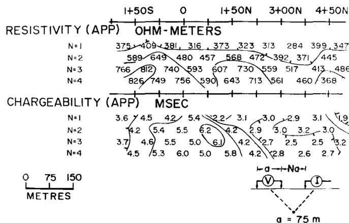
Figure 30.15. IP-resistivity data obtained on line C of orebody R (Huntec MK 3).
