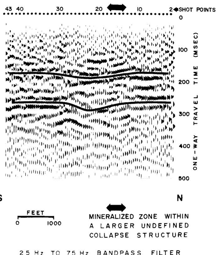
**Figure 30.27.** Reflection seismic data over orebody A. Shot spacing = 110 feet (34 m). Group offset = 1320 feet (402 m).
