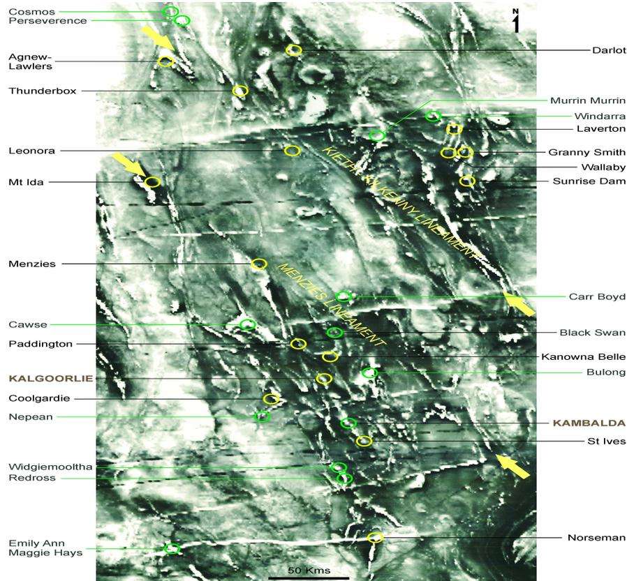
**Figure 6:** Lawlers-Kalgoorlie-Norseman BMR (now Geoscience Australia) 1960's vintage '1-mile-spaced' aeromagnetics illustrating regional scale features and the major nickel and gold districts. TMI image after Isles et al, (1989).
