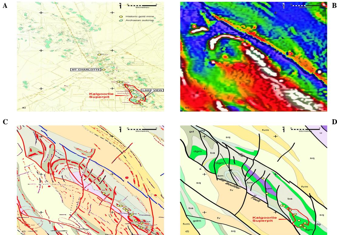
**Figure 3:** Kalgoorlie 'Golden Mile' district – detailed magnetic interpretation study. a- Distribution of outcrop (after Keats, 1987), b- Image of merged TMI and 1<sup>st</sup> vertical derivative (after Isles, 1989), c- Interpreter's 'structural skeleton' (Stage 1) with Stage 2 'solid geology', d- Completed geological interpretation
