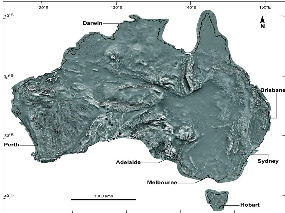
**Figure 2:** Aeromagnetic image of Australia comprising data entirely sourced from Geoscience Australia. The enhancement is a merge of TMI and 1<sup>st</sup> Vertical derivative grids.
