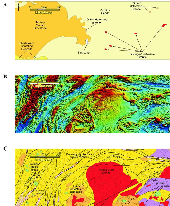
**Figure 4:** a) Surface geology from the ‘Fowler’ 1:250,000 sheet area, South Australia (PIRSA,2006). b) 400m-spaced ‘SAEI’ magnetic data (PIRSA,1992) covering the area in fig 4a. The image is a merge of shaded TMI with 1<sup>st</sup> Vertical Derivative. c) Interpretation map based on extrapolation from surrounding areas (after Fairclough et al 2002)
