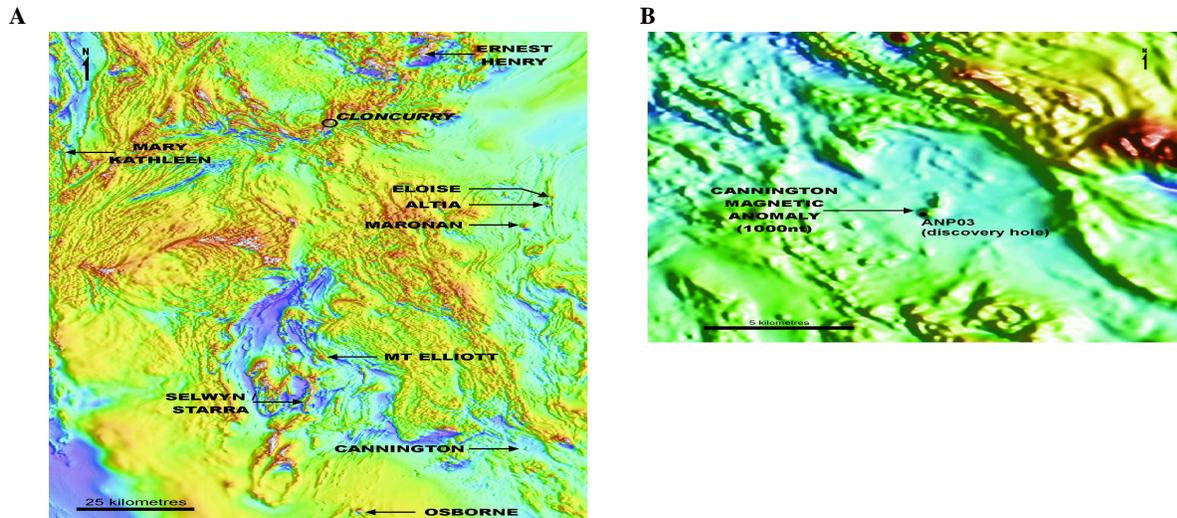
**Figure 7:** a) Regional 200m-spaced aeromagnetics over the Cloncurry Region, NW Queensland. Shaded TMI image, data courtesy Geoscience Australia. b) Section of the above data showing the Cannington magnetic anomaly.
