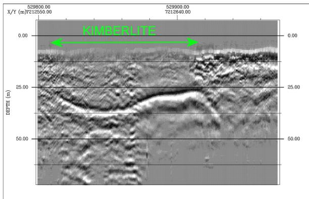
**Figure 7:** GPR responses showing the strong, smooth reflectivity of bedded crater facies kimberlite.
