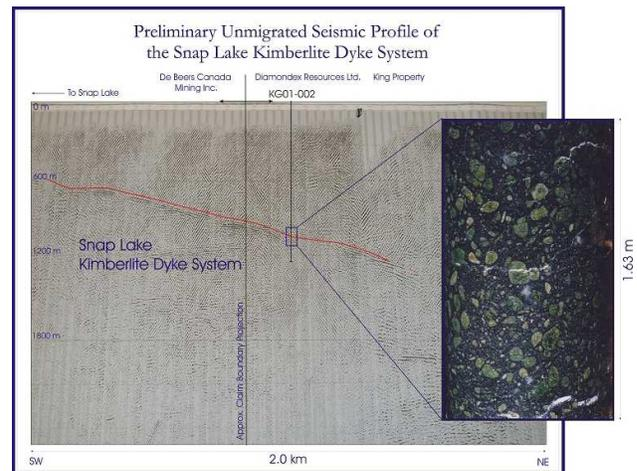
**Figure 9:** Seismic reflection section showing the response of the Snap Lake hypabyssal dyke.
