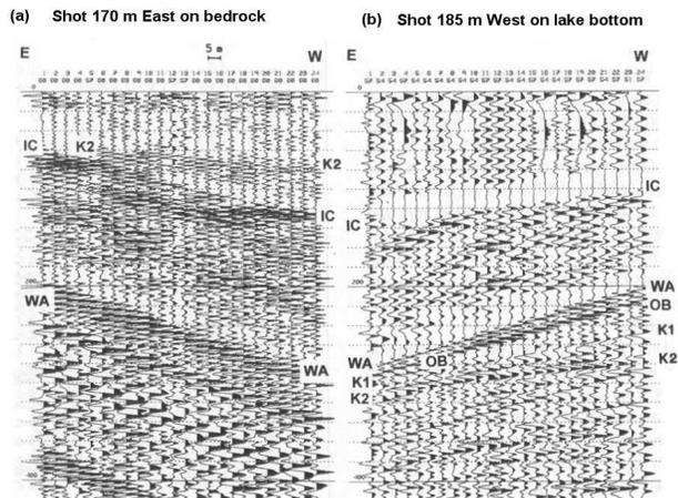
**Figure 6:** Seismic refraction survey over a kimberlite pipe showing water (WA), ice (IC), overburden (OB), weathered kimberlite (K1) and fresh kimberlite (K2) arrivals.
