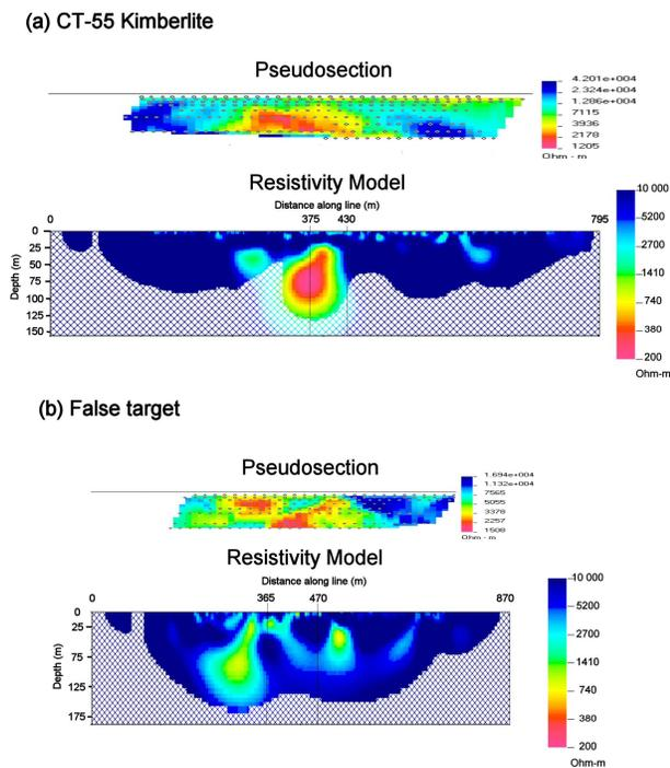
**Figure 5:** CCR surveys over a land-based kimberlite and over a drill tested barren target.
