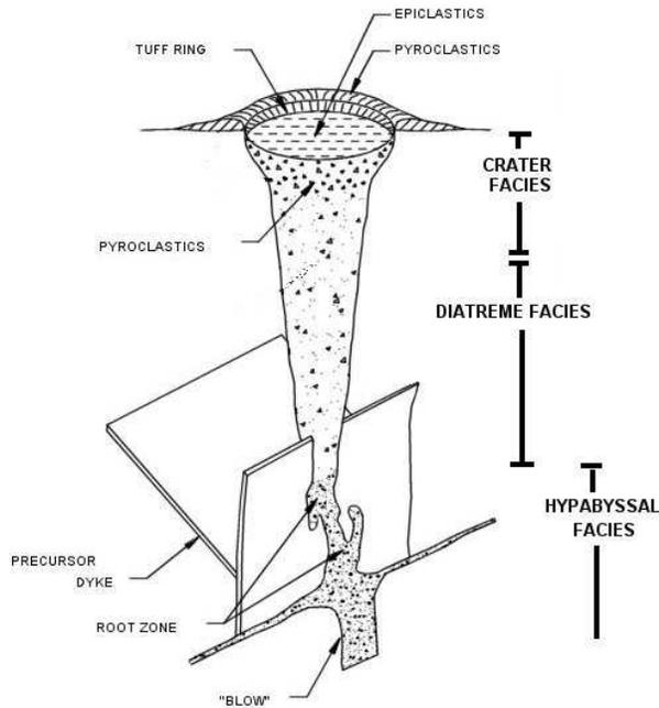
**Figure 1:** Facies and components of a typical kimberlite pipe with no erosion (modified after Mitchell (1986)).
