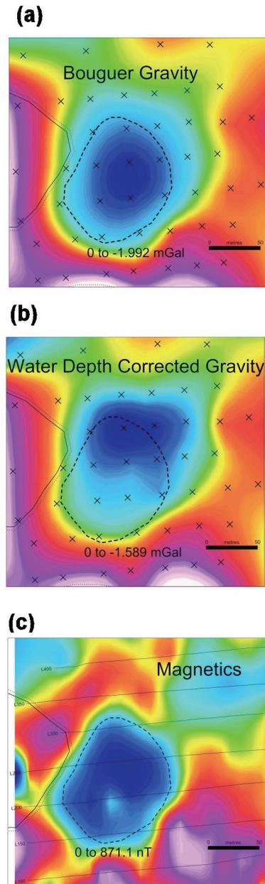
**Figure 4:** Crater facies kimberlite gravity and magnetic response of the Torrie Pipe showing the effect of a large granitic xenolith in the southern end of the pipe. Panel (a), with no bathymetric correction, does not correctly image the xenolith.
