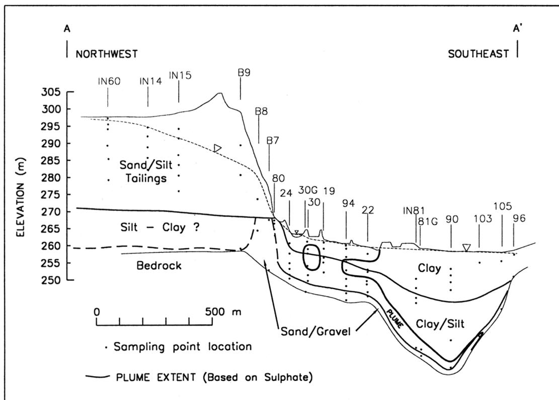
Figure 2: Cross-section A-A' from Figure 1, showing stratigraphic units and plume boundaries as of September, 1994.
