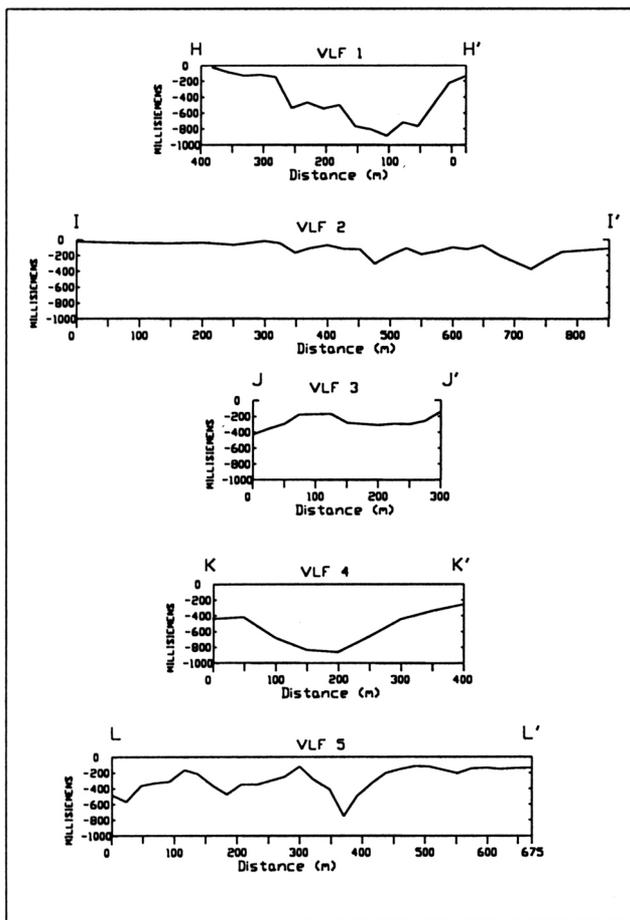
**Figure 4:** Cross-sections based on VLF resistivity showing resistivity plotted in negative (for relative comparison purposes).
