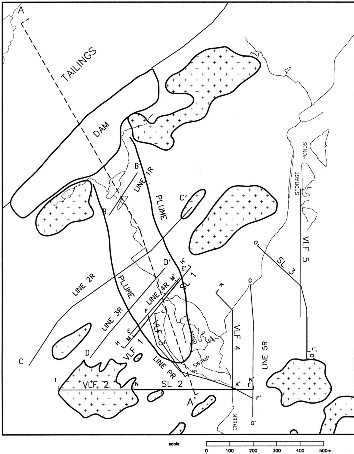
**Figure 1:** *The study area, showing locations of geophysical cross sections and plume extent.*
