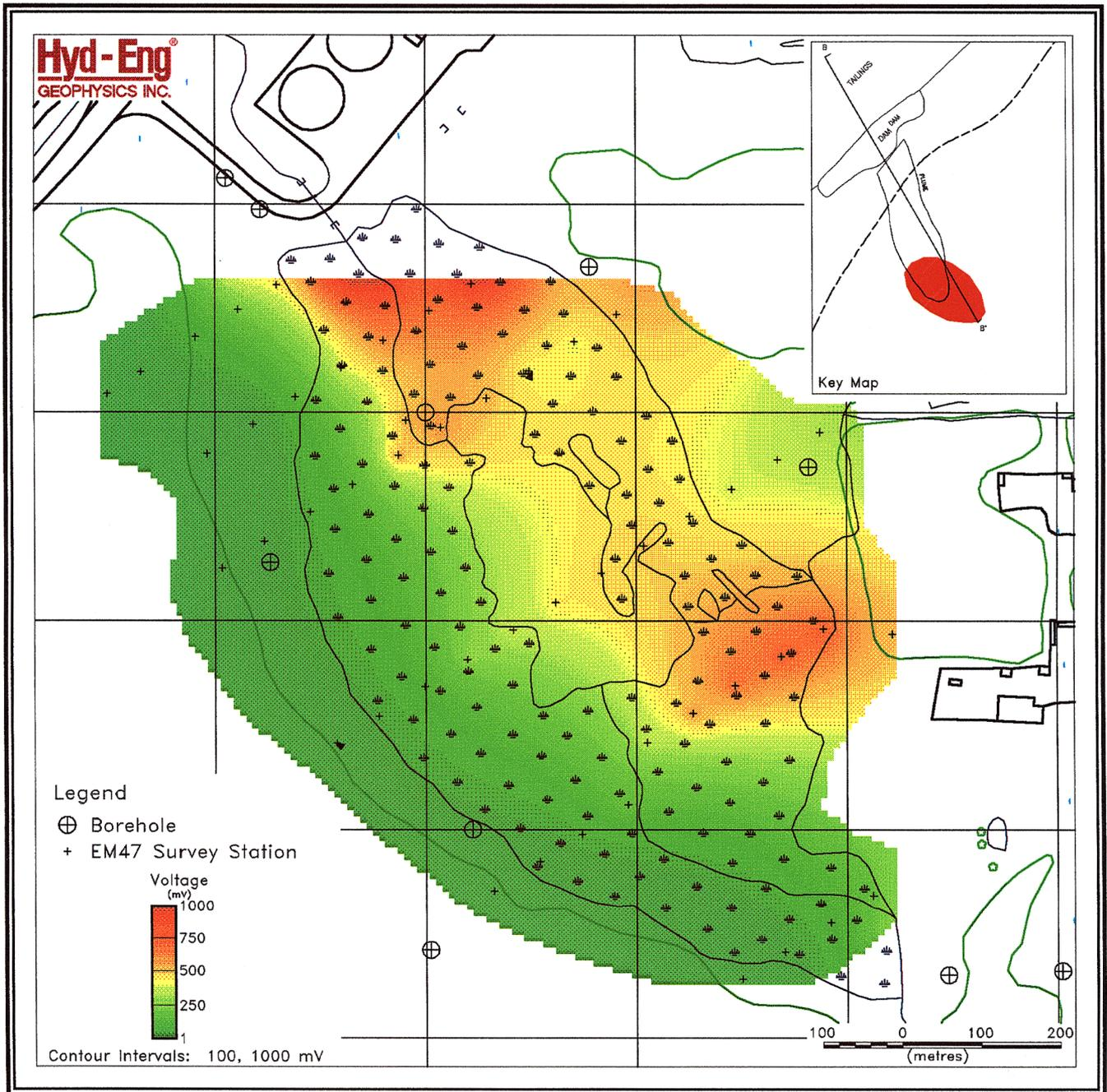
Figure 6: Time domain EM data, Pistol Dam Project (Channel 8, data in millivolts).
