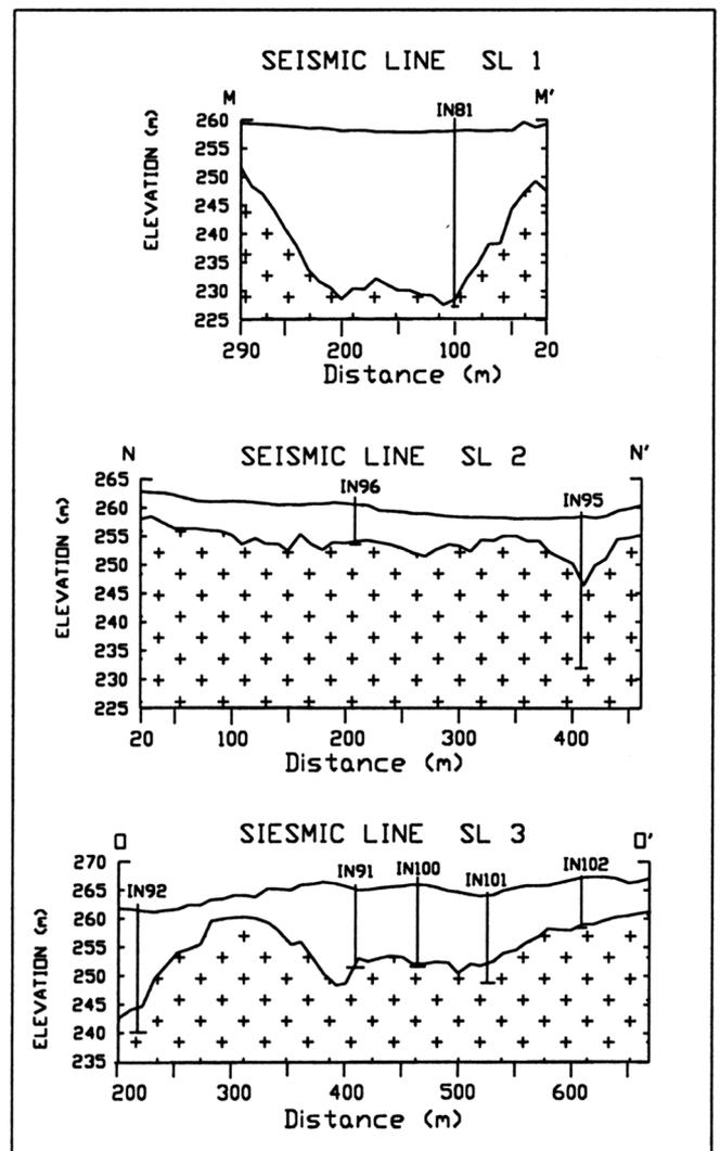
**Figure 5:** Cross-sections based on seismic refraction data showing interpreted depth to bedrock.
