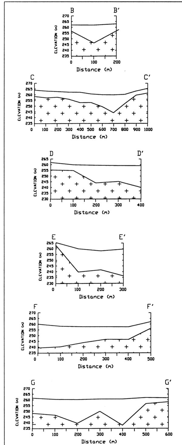
**Figure 3:** Cross-sections based on galvanic resistivity soundings showing interpreted depth to bedrock.
