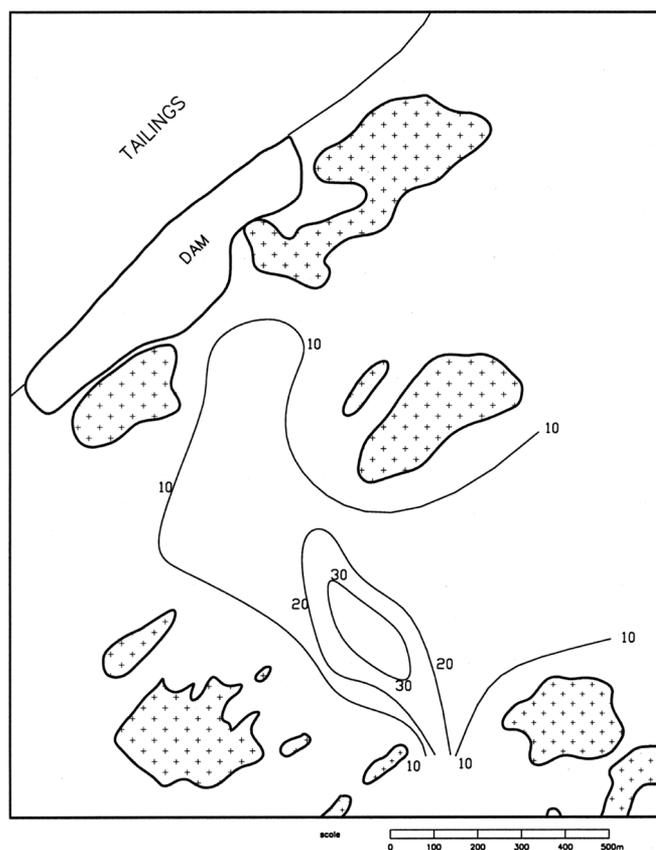
**Figure 7:** Map of estimated depth to bedrock (m) in the study area based on geophysical, borehole and piezometer data.
