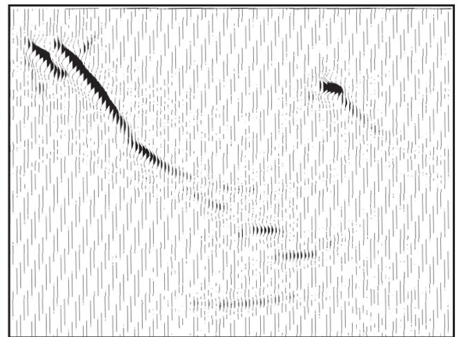
**Figure 3d:** Vertical incidence response of the structure in (a) after migration of the seismic data. The Pipe formation is represented by the pelitic schist unit.
