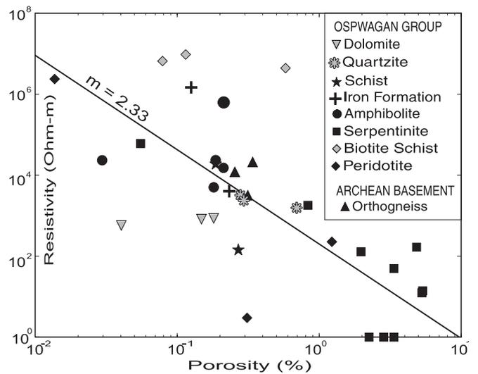
**Figure 6:** Rock property results from a suite of samples provided by Inco Limited, Exploration. Plotted is the log of resistivity versus of the log of porosity to facilitate the interpretation of conductivity in terms of ionic transport (fluids) versus electronic transport (metals and semiconductors).
