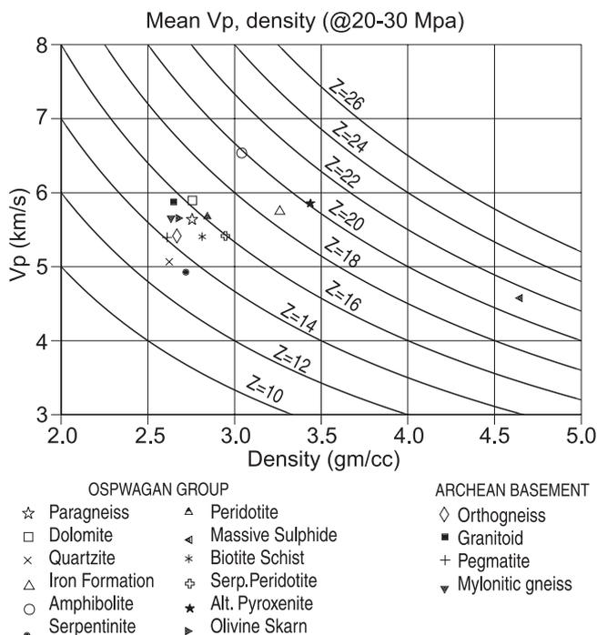
**Figure 4:** Mean  $V_p$  and densities measured for a suite of rock samples from Thompson. Measurements were made on dry samples under hydrostatic pressure (30 MPa), or under an applied uniaxial stress (17–25 MPa). Note that in the absence of measurements on massive sulphides from Thompson, the  $V_p$  and density values for massive sulphide are for a pyrrhotite-rich sample from Sudbury measured at a confining pressure of 200 Mpa.
