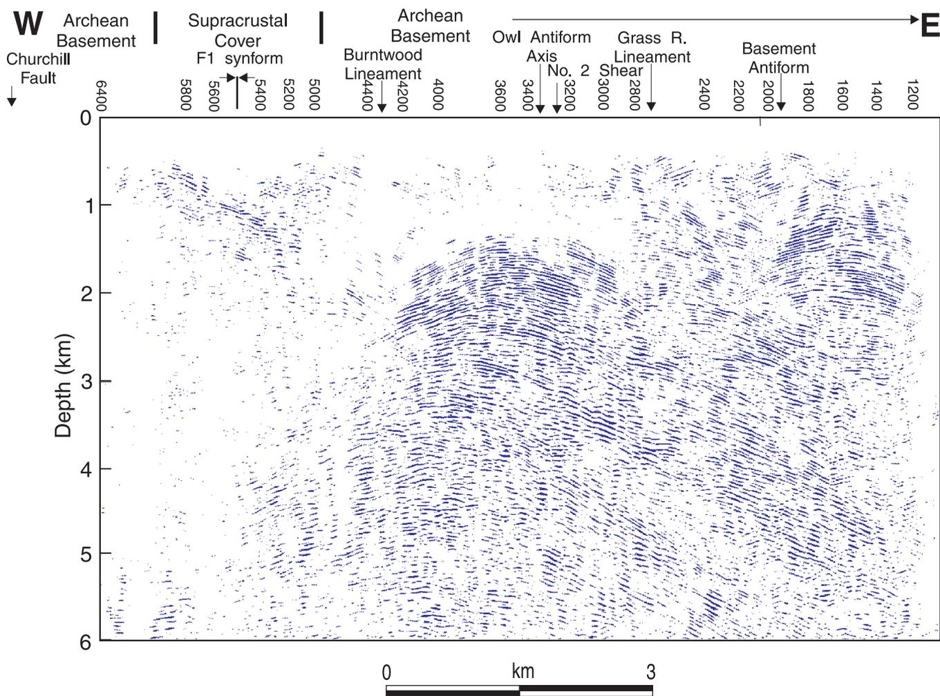
**Figure 8:** Unmigrated seismic data for Line 1A. This stack was obtained by using low stacking velocities (6000 m/s).
