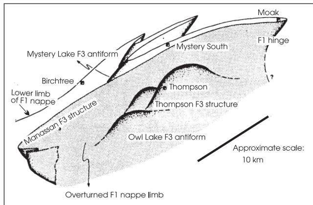
**Figure 2a:** 3-D sketch of the refolded Thompson nappe structure as seen from the southeast (from Bleeker 1990a). The location of the mines in the Thompson vicinity are indicated by the half-shaded boxes.
