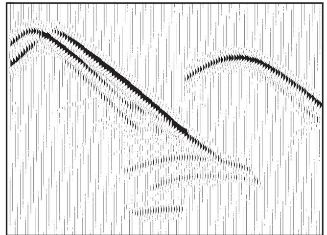
**Figure 3c:** Simulated seismic vertical incidence response of the structure in (a) (unmigrated).
