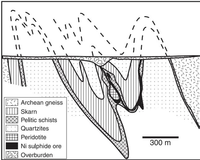
**Figure 3a:** Profile through the Thompson structure, Thompson Mine, 24400 N section, looking towards the northeast (from Bleeker 1990a).
