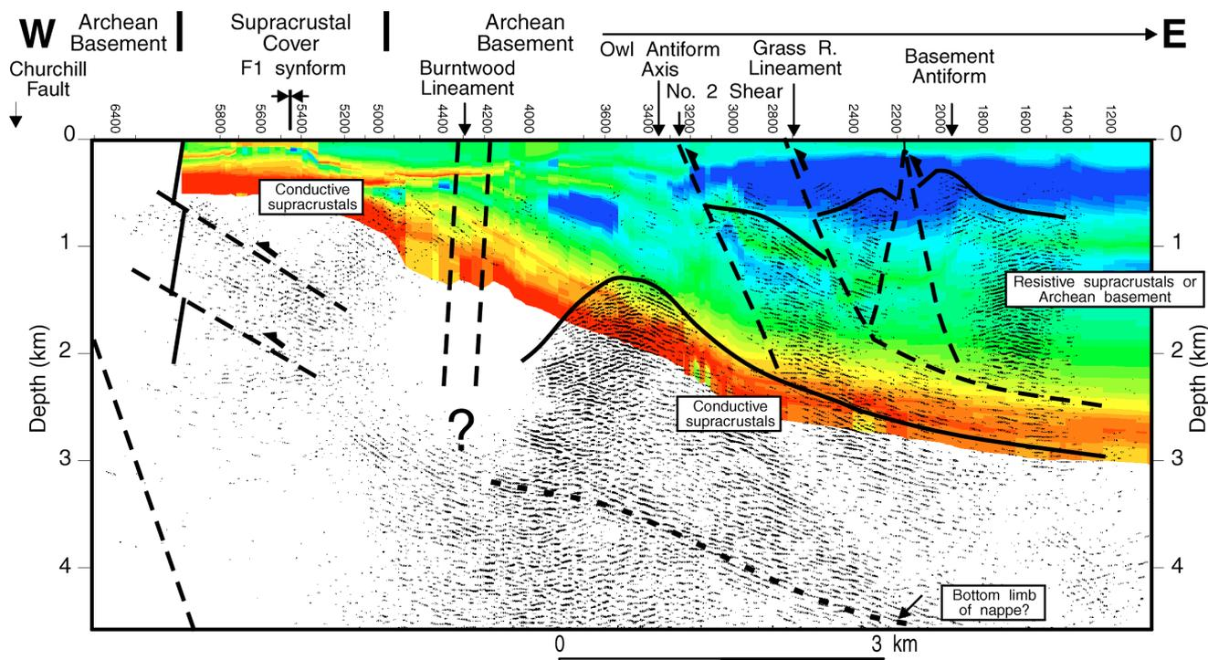
Figure 9: Hybrid migrated seismic data for Line 1A with the resistivity versus depth image for the coincident EM profile overlain in colour.
