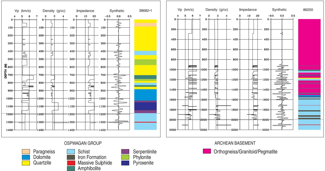
**Figure 5:** Synthetic  $V_p$ , density, seismic impedance and seismic response determined for the geologic log from (a) borehole 38682-1 and (b) borehole 86250, using the rock property measurements. The seismic response is determined for the frequency range of 35–130 Hz typically used in high frequency seismic surveys. The log response for a 10 m thick massive sulphide layer embedded within a schist host rock has been added to the logs (below the dashed line) for comparison.
