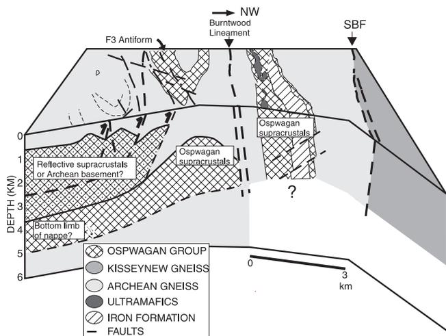
**Figure 10:** Perspective view (looking from the northeast) of the combined seismic/EM interpretation.
