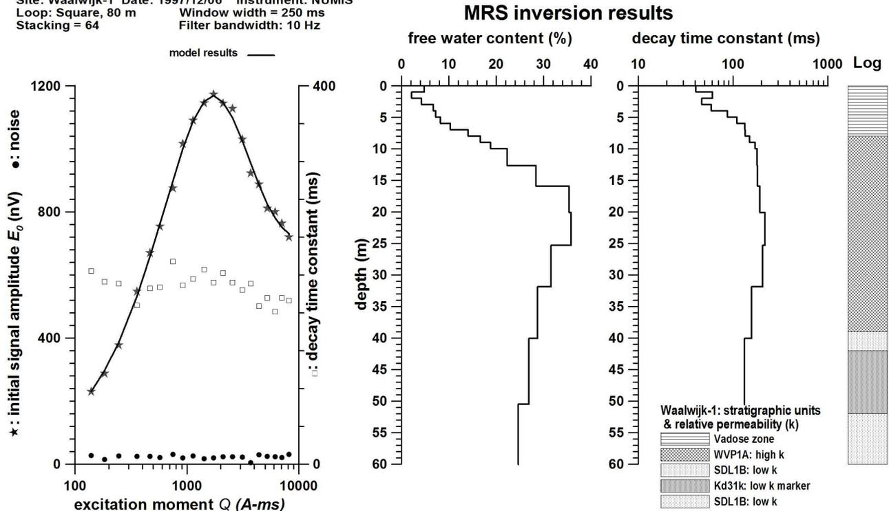
**Figure 2:** MRS data set & inversion; Waalwijk-1, Netherlands: from left to right (1) MRS data summary, field [ $*$  -  $E_0$ , -  $T_2^*$ , • - noise] & model [—] vs.  $Q$ , (2 & 3) MRS inversion results: water content & decay time constant vs. depth, (4) Lithological log inferred from three nearest boreholes; in this model, the WVP1A unit has a higher permeability than the SDL1B and Kd31k units. (Item 4, TNO, 1998).
