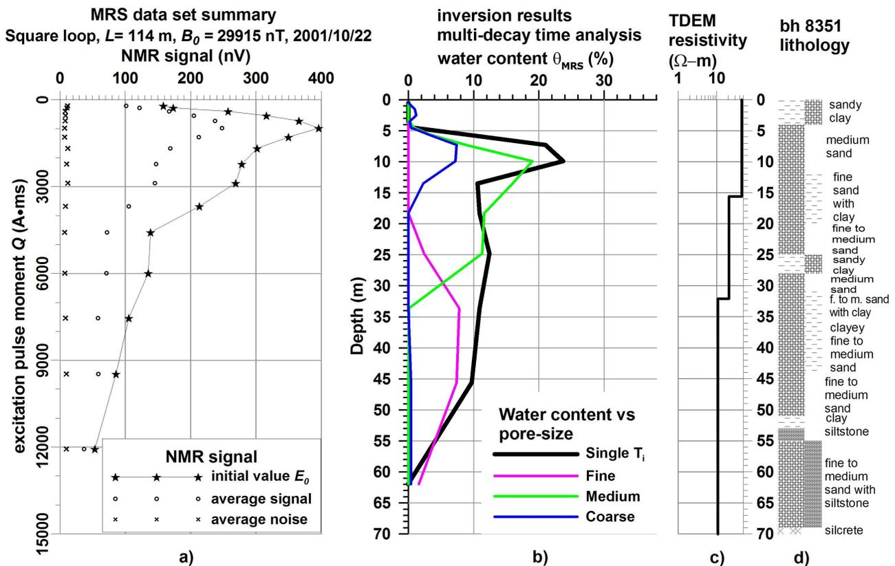
**Figure 3:** MRS investigation on a paleo-channel near Maun, Botswana, site BH8351; a) data set summary, b) MRS inversion results with multi-decay time analysis, c) TDEM resistivity, d) BH 8351 lithology (after Mangisi, 2004; Roy and Lubczynski, 2005).
