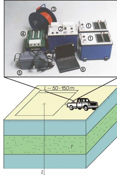
**Figure 1:** MRS set-up: - bottom: typical MRS field layout using a square loop; top inset: NUMIS<sup>PLUS</sup> system - IRIS Instruments (2001): (1): DC/DC converter, (2) main unit, (3) wire loop, (4) tuning box, (5) rechargeable battery, (6) control & data acquisition PC.
