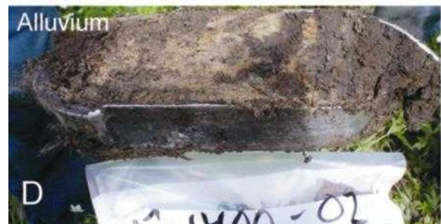
**Figure 14:** Soils likely to be encountered during geochemical surveys in northern Ontario. (A) Shows a typical dry podzol soil with a well developed Ae-horizon (whitish) and an underlying B-horizon. (B) Shows a typical B-horizon in a clay substrate. (C) Shows a well humified peat. (D) Shows alluvium (note mottling and organic-rich laminations).
