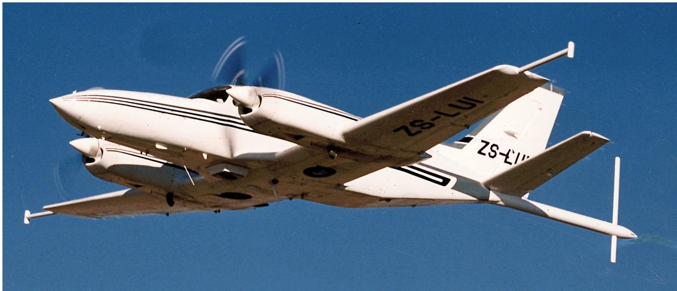
**Figure 1:** Cessna 404 Titan aircraft with triaxial aeromagnetic gradiometer installation. The separation between the wingtip sensors ( $\Delta H_x$ ) is 16.46 m, the wingtip and tail sensors ( $\Delta H_y$ ) is 8.68 m, and the tail sensors ( $\Delta H_z$ ) is 1.92 m.
