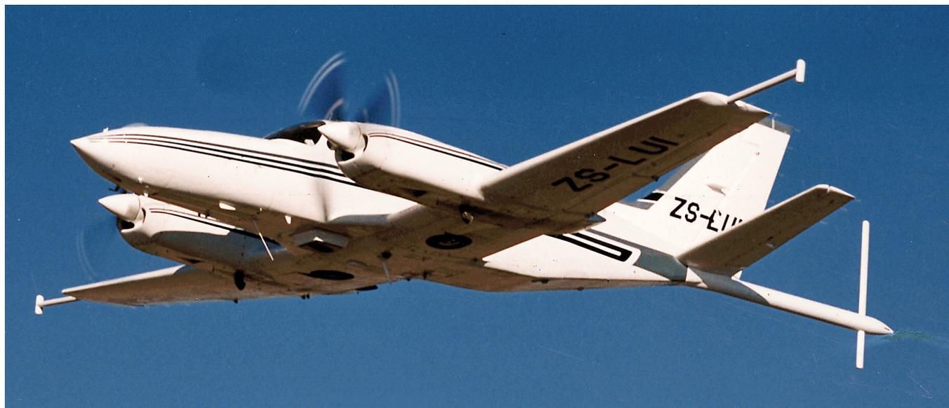
**Figure 1:** Cessna 404 Titan aircraft with triaxial aeromagnetic gradiometer installation. The separation between the wingtip sensors ( $DH_x$ ) is 16.46 m, the wingtip and tail sensors ( $DH_y$ ) is 8.68 m, and the tail sensors ( $DH_z$ ) is 1.92 m.
