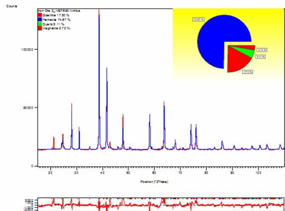
**Figure 2:** Rietveld analysis of NIST SRM 693 iron ore from Labrador.
