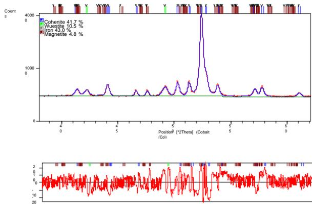
Figure 3: A portion of the Rietveld simulation overlaid with the measured data.
