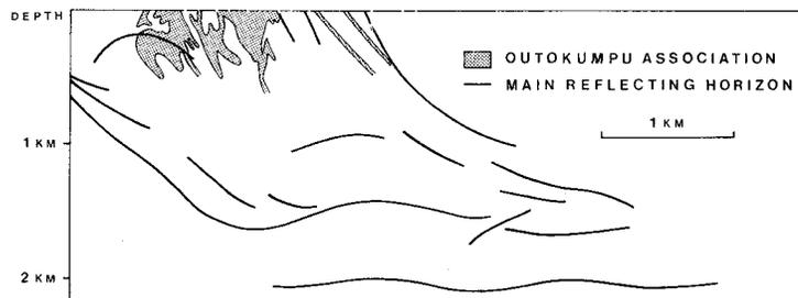
**Figure 31.13.** Reflection seismic cross-section through the Outokumpu area.
