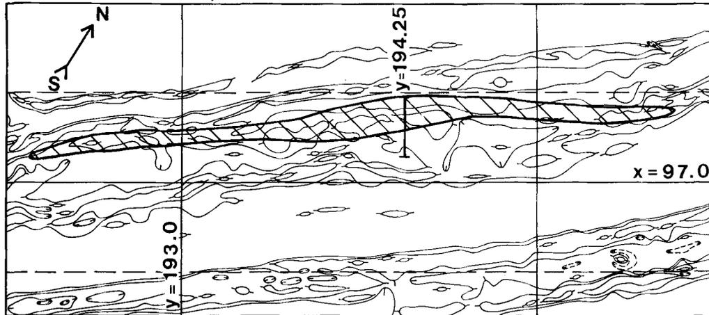
**SLINGRAM MAP (REAL COMPONENT)**CONTOURS:  $\pm 4, 8, 16$  % etc.  $f=1775$  cps  $a=40$  m
