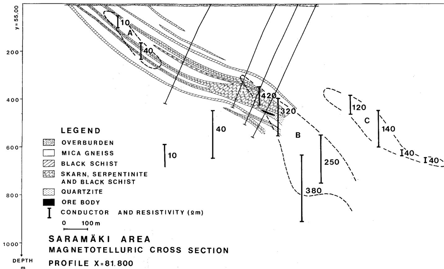
Figure 31.14. Magnetotelluric cross-section in the Saramäki area.
