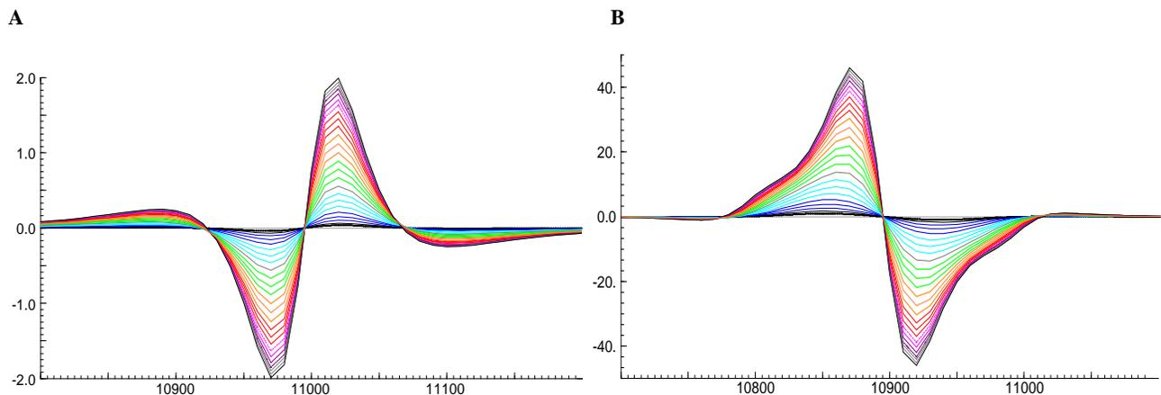
**Figure5:** Off-time typical anomaly shape detected by an in-loop system over a) a vertical 200m x 200 m thin plate conductor located at 11000 b) an horizontal 200 m x 200 m thin plate located between 10800 and 11000.
