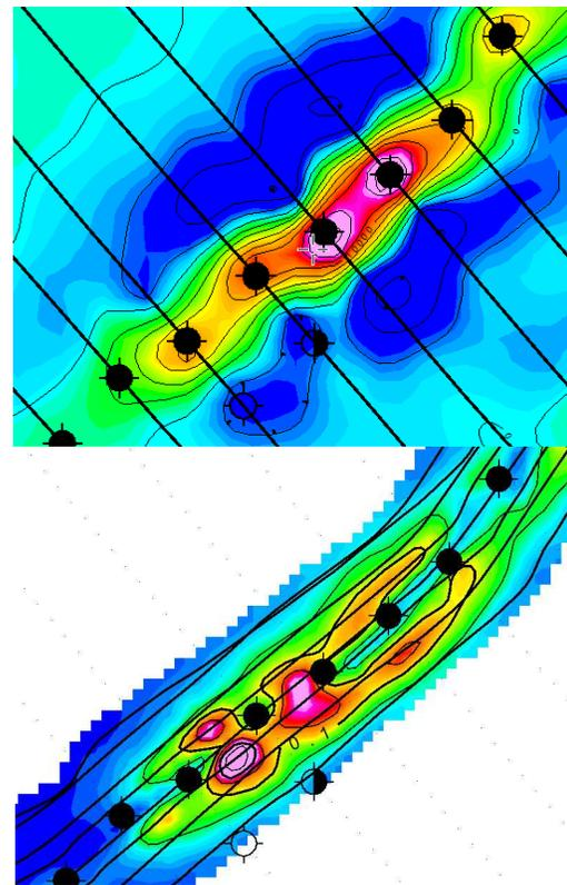
**Figure 17:** a) Plot the MEGATEM II flight path superimposed on a color map of X component mid off-time channel amplitude. Black dots are the anomaly pick locations b) Plot of a VTEM flight path flown parallel to the same conductor on a colour map of an equivalent off-time window amplitude.
