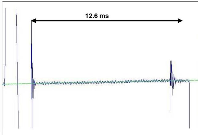
**Figure 9:** Example of a spheric burst that was detected at the end of an off-time period. On average a spheric lasts less than 1 ms
