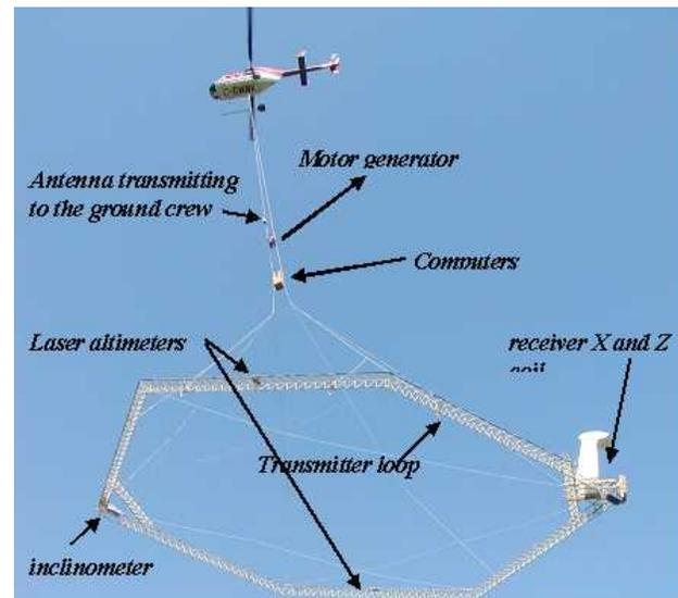
Figure A6: Details of the SKYTEM system components (courtesy of SkyTEM ApS)
