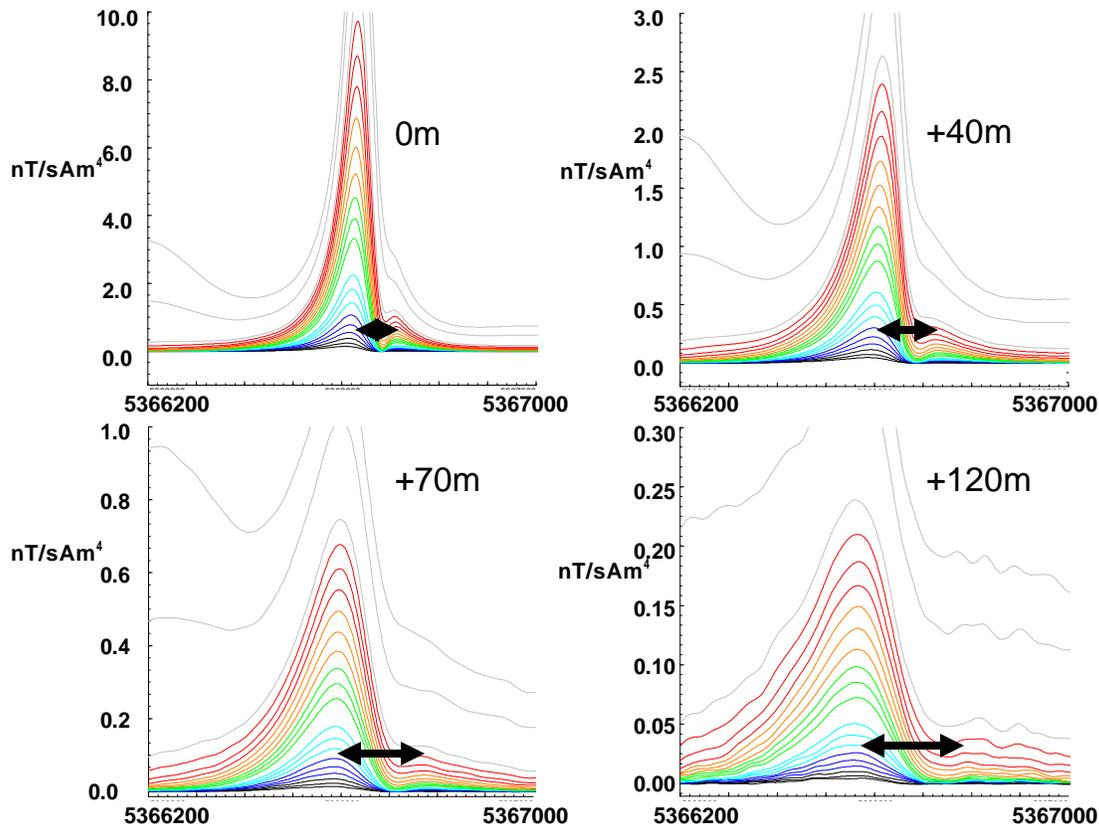
**Figure 13:** VTEM profiles over the Iso-Magusi deposit at different altitudes relative to the nominal flying height. The distance between the two anomalous peaks increases with flying height.
