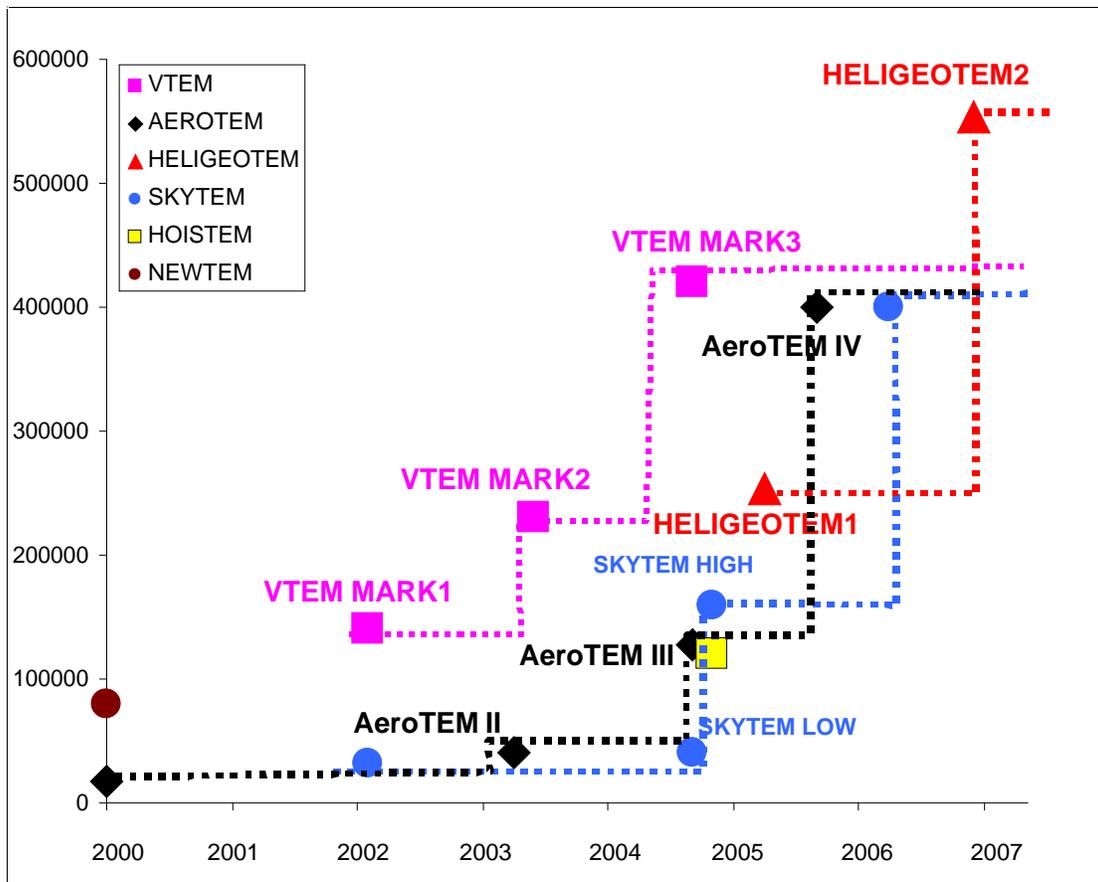
Figure 7: Graph showing the steady increase in dipole moment (Am<sup>2</sup>) for all HTEM systems during the last 5 years
