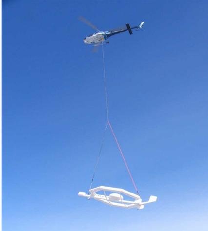
**Figure A1:** The AeroTEM II in flight (courtesy of Aeroquest Ltd).
