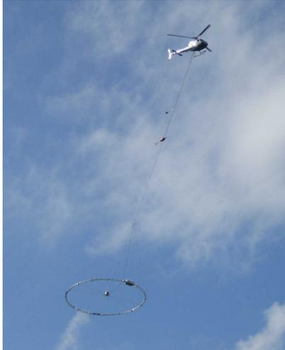
**Figure A3:** The HeliGEOTEM II in flight (courtesy of Fugro Airborne Surveys).
