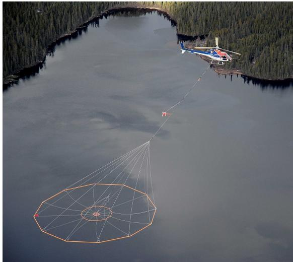
Figure A5: The VTEM system in flight (courtesy of Geotech)
