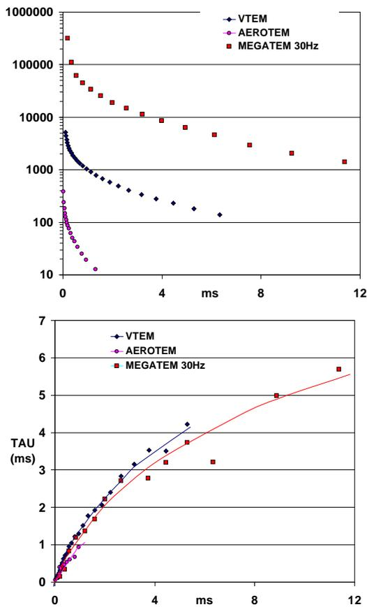
**Figure 16:** a) Decay curves of the VTEM, AEROTEM and MEGATEM anomalous responses over the Montcalm deposit b) Variation of the time constant with time : running Tau
