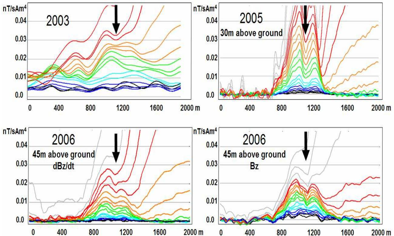
**Figure 10:** VTEM stacked profiles from surveys flown in 2003, 2005 and 2006 over the Caber deposit which is located by the arrow. The red profiles are early off-time and the blacks are the late off-time. Significant improvement in the noise level can be observed between 2003 and 2006
