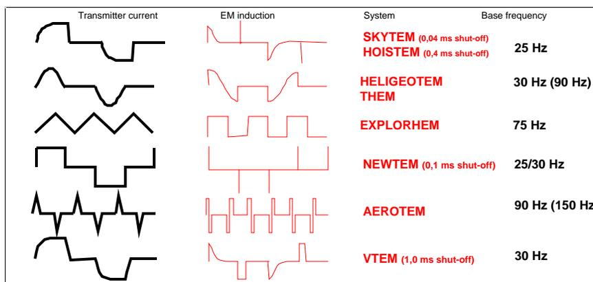
**Figure 6:** Schematic representation of the various current waveforms used by the HTEM systems. The primary EM field detected by the receiver coil is proportional to the time derivative of current waveform.
