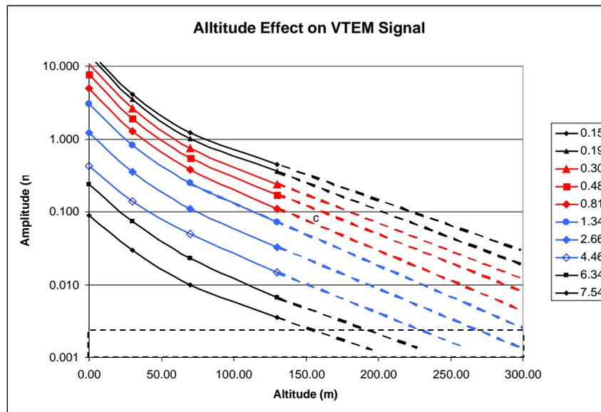
**Figure 14:** Graph of the amplitude of the VTEM anomaly over the Magusi River deposit decreasing with flying height. The grey area corresponds to the noise level
