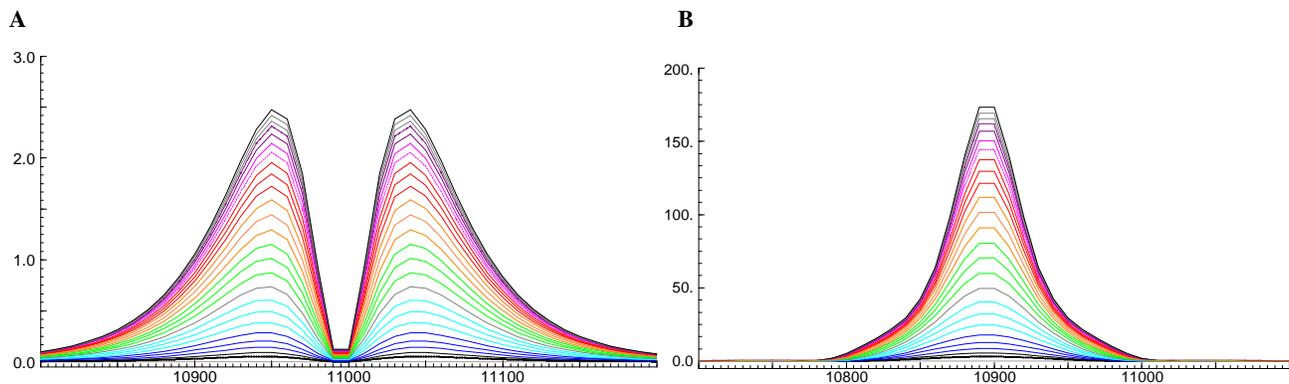
**Figure 4:** dBz/dt off-time typical anomaly shape detected by an in-loop system over a) a vertical 200 m x 200 m thin plate conductor located at 11000 b) a horizontal 200m x 200 m thin plate located between 10800 and 11000. Note that the difference in the vertical scale between the two plots.
