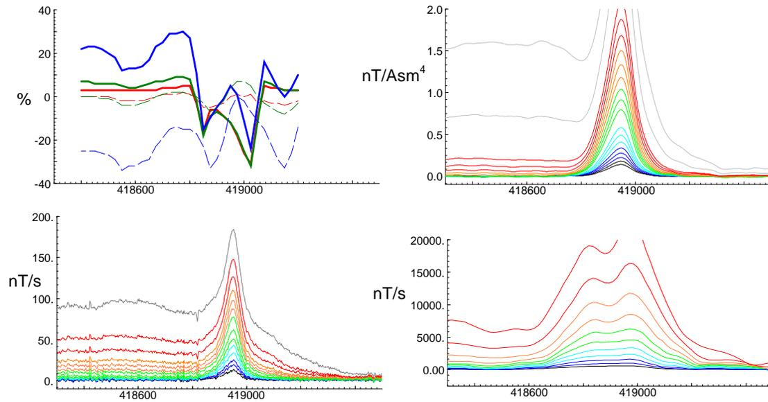
**Figure 15:** Stacked profiles over the Montcalm deposit, Ontario of a) ground HLEM at 222, 444 and 1777 Hz (200 m coil spacing). Continuous lines are in-phase profiles and dashed lines are quadrature b) VTEM c) AeroTEM II d) MEGATEM II  $dBz/dt$  at 30Hz.
