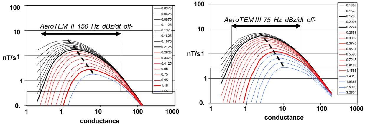
**Figure 12:** Off-time anomaly amplitude based on modelling of 200 m x200 m vertical plates at 10m below surface as a function of their conductance for the AeroTEM II and III
