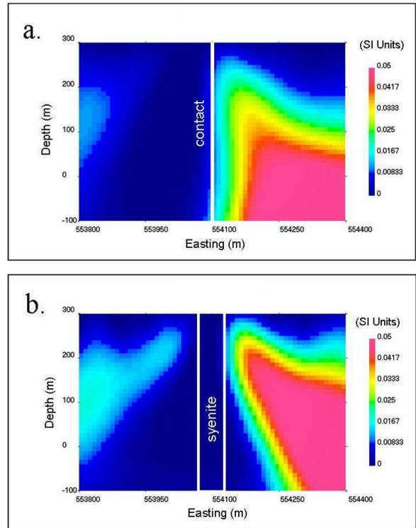
**Figure 3:** North-facing cross-section through the default 3D inversion results for a) the faulted contact model and b) the syenite intrusive model.
