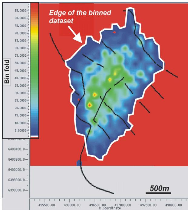
Figure 5: Fold coverage of the 3D data using 10x10 m bins.
