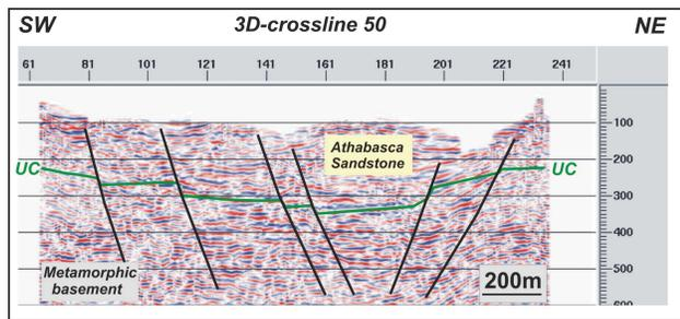
Figure 7: Preliminary interpretation of crossline 50 from the 3D survey. This line is parallel with the P2 trend.
