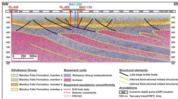
Figure 6: Interpreted 2D high-resolution line 12 running perpendicular to the P2 trend.
