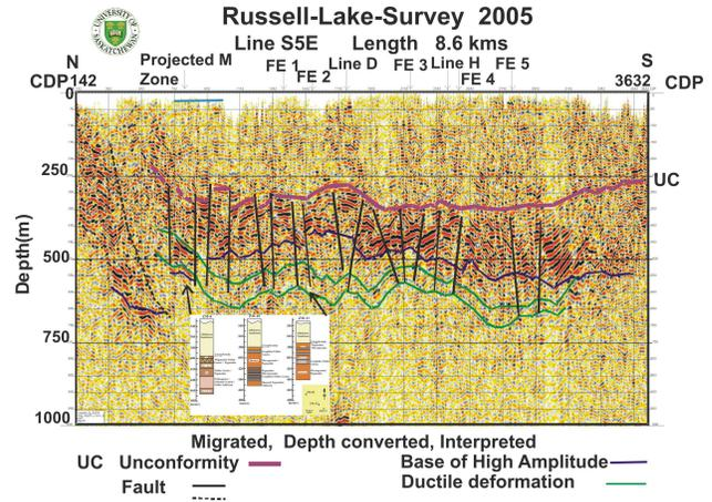
Figure 8: Seismic profile of line 5 from Russell Lake. Correlation to borehole geology illustrates the lithologic complexity in the vicinity of UC.
