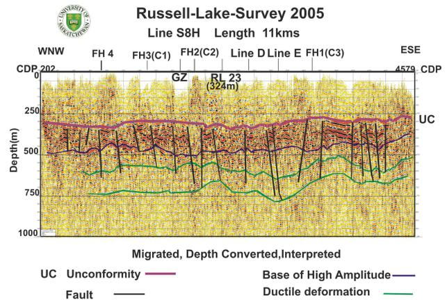
Figure 9: Seismic section of line 8 illustrates preservation of early ductile deformation in the basement.
