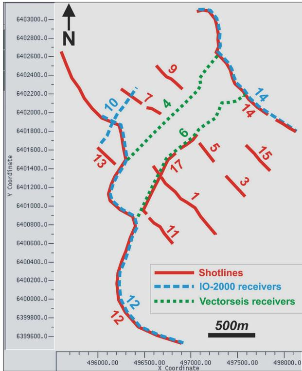
Figure 4: Acquisition geometry of the 3D survey and 2D profiles 12 and 14.
