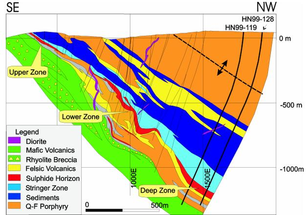
**Figure 2:** Composite geological cross-section through Halfmile Lake deposit based on projection of drilling results to a southeast-northwest section. Borehole HN99-128 was used for the VSP survey. See Figure 1 for surface location of the cross-section.
