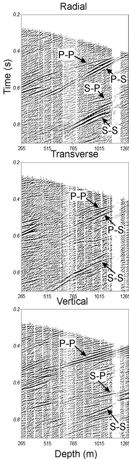
**Figure 3:** processed radial, transverse and vertical components from shot site B. Several events are annotated: P-P (incident P-wave, scattered P-wave), P-S (incident p-wave, scattered S-wave), S-P (incident S-wave, scattered P-wave), and S-S (incident S-wave, scattered S-wave).
