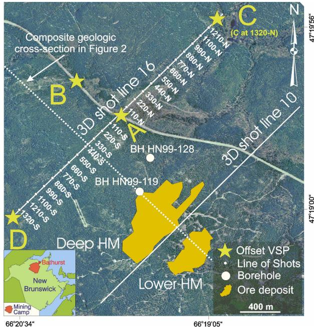
**Figure 1:** VSP acquisition geometry used at Halfmile Lake. The shots for the offset VSP are indicated by yellow stars. Recording depths in borehole HN99-128 ranged between 265m and 1300m. The location of the composite geological cross-section in Figure 2 is also shown.
