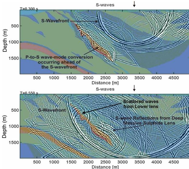
**Figure 4:** Simulation of shear wave propagation at Halfmile lake. The wavefields at 0.300s (top) and 0.550s (bottom) are shown. The arrow indicates the shot location. The snapshot at 0.3s shows P-S wave-mode conversion occurring ahead of the S-wavefront whereas the snapshot at 0.550s shows strong reflections from the deep zone. The three sulfide lenses are shown in red in the background.
