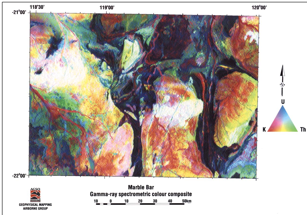
**Figure 4:** A three-color composite of airborne gamma ray spectrometry for the Marble Bar, 1:250 000 map sheet in Western Australia. This map was prepared and released by the “Geophysical Mapping Airborne Group” of the Australian Geological Survey Organization (AGSO).
