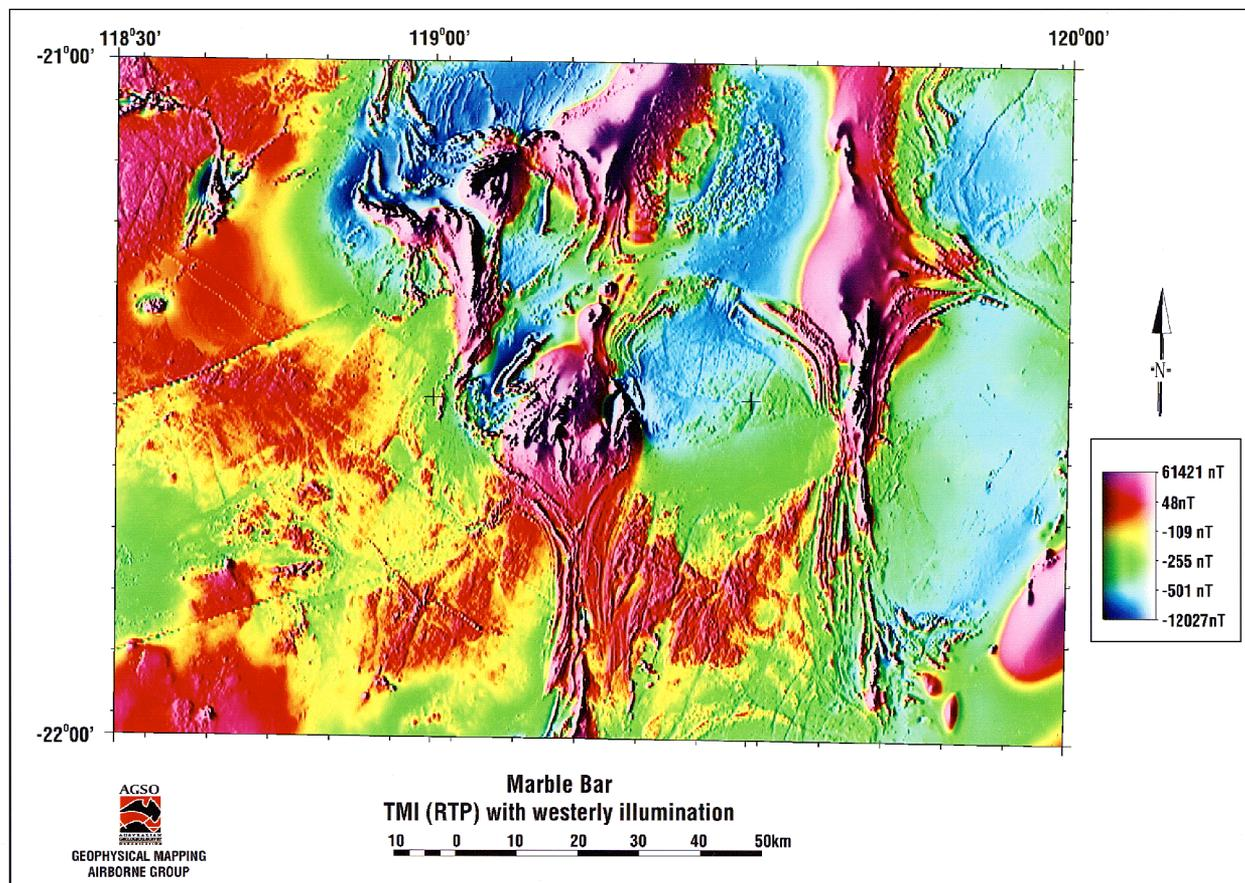
**Figure 3:** The total magnetic intensity, reduced to the pole, with a westerly “illumination” for the Marble Bar, 1:250 000 map sheet in Western Australia. This map was prepared and released by the “Geophysical Mapping Airborne Group” of the Australian Geological Survey Organization (AGSO). The data were collected by AGSO in 1996 on east-west lines flown 400 m apart and 80 m above terrain.
