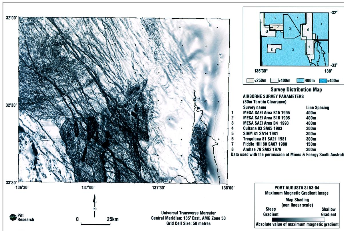
**Figure 7:** Aeromagnetic map of the Port Augusta 1:250 000 map sheet, South Australia, showing maximum magnetic gradient of the total magnetic intensity and representing a compilation of company and government surveys (image courtesy Pitt Research).
