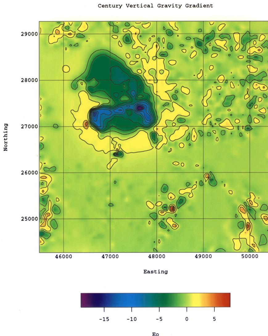
**Figure 5:** The terrain-corrected vertical gravity gradient calculated for a simulated airborne gravity gradient survey over a 3-D finite mesh model of the Century ore body and its surrounds in northwest Queensland, Australia.
