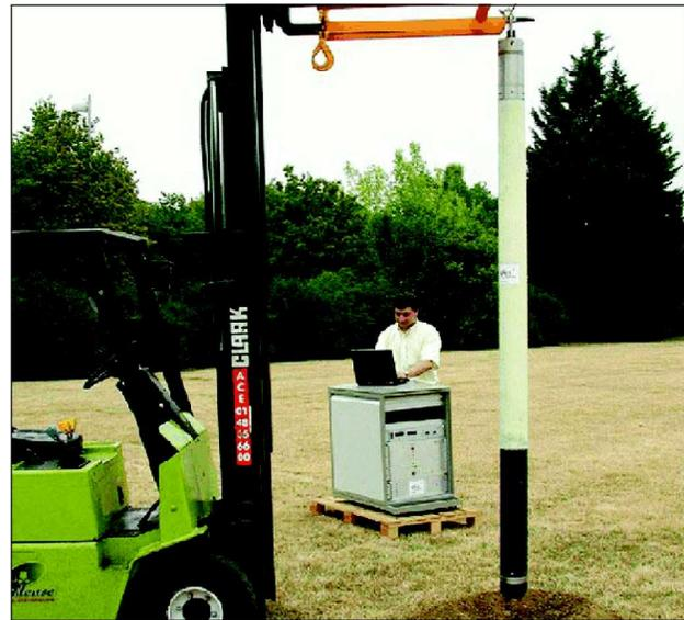
**Figure 8:** Neutron Activation Multi-element Borehole Assay system – In-situ assay for Ni, Cu, S, Fe, Si, Mg, Al, Mn, Cr etc.
