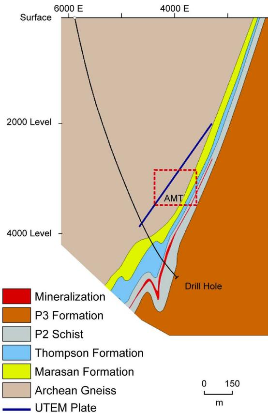
**Figure 11:** Drilling on a deep interpreted plate conductor which was targeted on a deep AMT target zone (red dashed line box). Depth levels are in feet.
