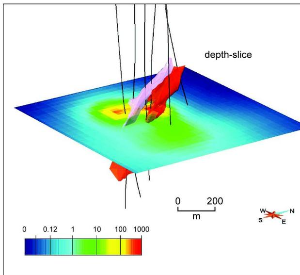
**Figure 32:** Xstrata Nickel's Nickel Rim South deposit - same conductivity inversion model showing mineralized zones (red and pink shapes) with depth slice through the inverted conductivity data cube (from Phillips 2006).
