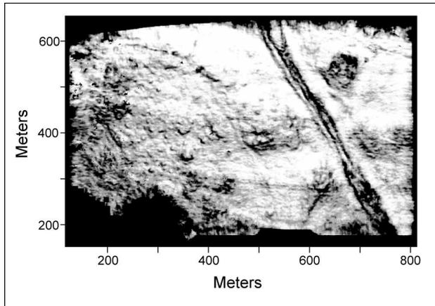
**Figure 41:** 3D Reflection Seismic Bushveld Complex – Plan view of Coherency Map along the UG2 horizon showing Potholes and Fault (from Laroque et al, 2002).
