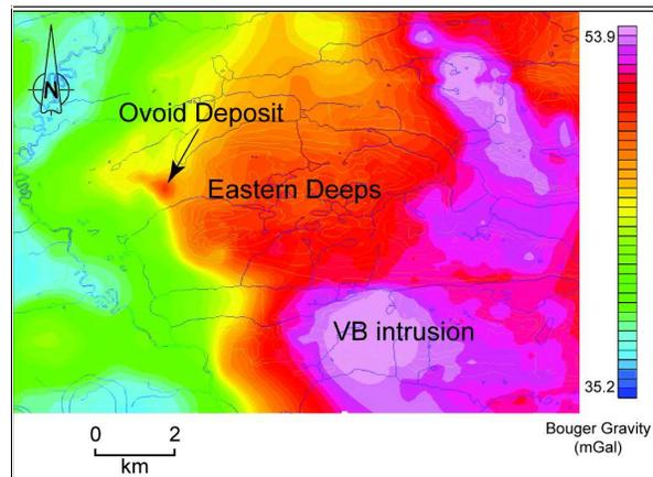
Figure 20: Ground Bouguer Gravity over the Ovoid Deposit, and Eastern Deeps, and Voisey's Bay (VB) mafic intrusives.
