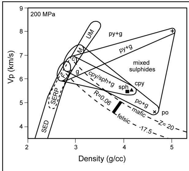
**Figure 7:** Seismic P wave Velocity versus Density for common rock types (Sed=Sedimentary, Serp=Serpentinized, F=Felsic, M=Mafic, UM=Ultramafic) and common sulphide minerals with lines of constant acoustic impedance Z and typical Reflectivity value R (After Milkereit et al., 2000).
