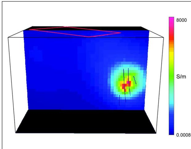
**Figure 31:** Xstrata Nickel's Nickel Rim South deposit : 3D voxel based inversion of borehole UTEM data for a high conductivity contrast body using new UBC TEM inversion software (from Phillips 2006).
