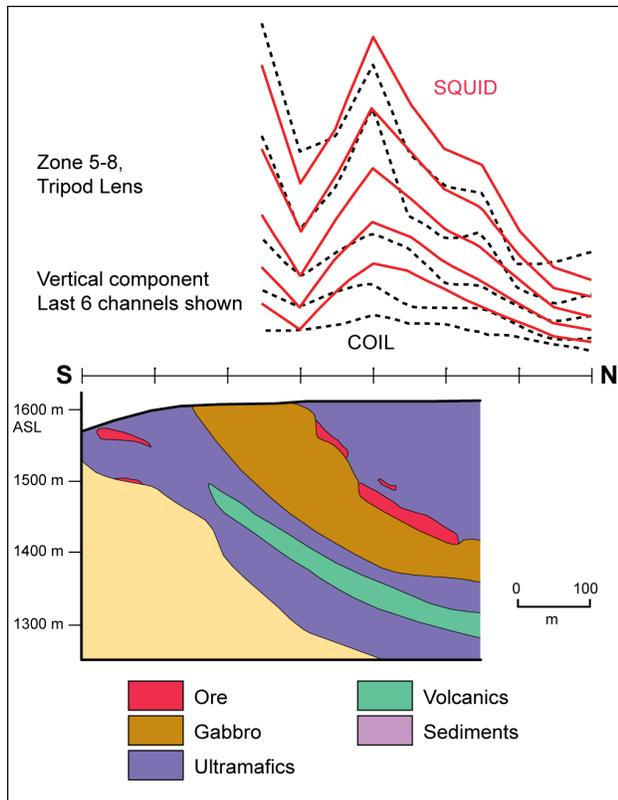
**Figure 37:** Ground Moving Loop 5 Hz TEM responses over small high conductance body at Raglan Quebec (Xtrata Nickel) - B field High Temperature SQUID receiver data vs Coil (dB/dT) Receiver data (from Osmond et al 2002).
