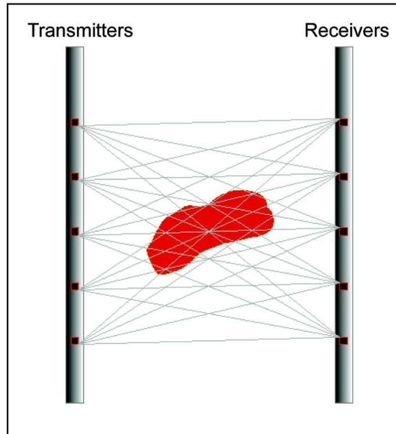
**Figure 12:** Seismic Crosshole Tomography – Schematic showing sample cross hole acoustic ray paths from transmitter locations in hole on the left to receivers in the hole on the right.
