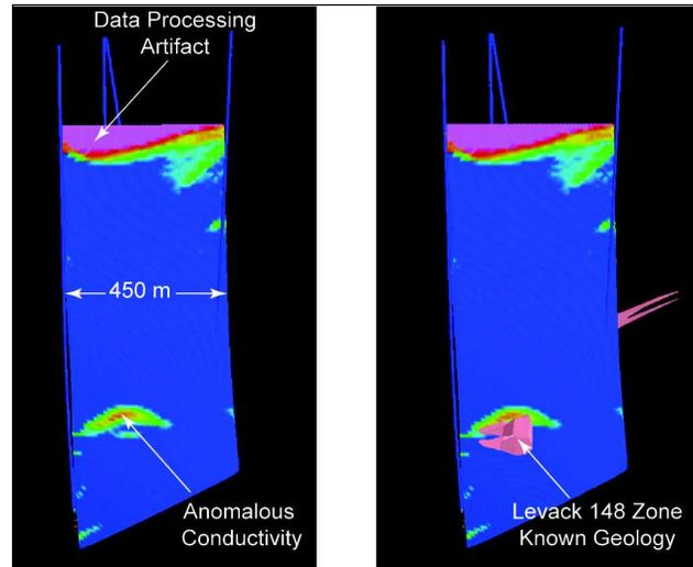
**Figure 33:** Levack 148 Zone - Left - Crosshole Radio Imaging (RIM) image – warm colours indicate higher radio wave attenuation and higher conductivity. Right – Known mineralization envelope (pink body) superimposed on RIM image.
