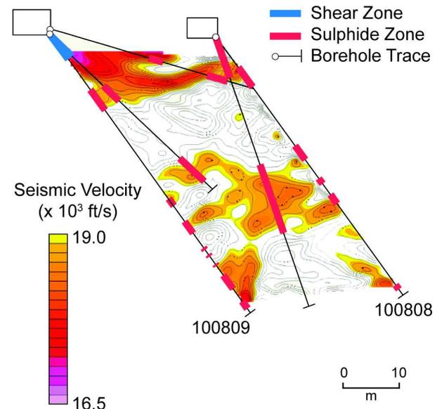
**Figure 13:** Seismic Tomography image - Thompson 1-D - low velocity zones shown in warm colours and sulphide intersections in drill holes shown as red bars.
