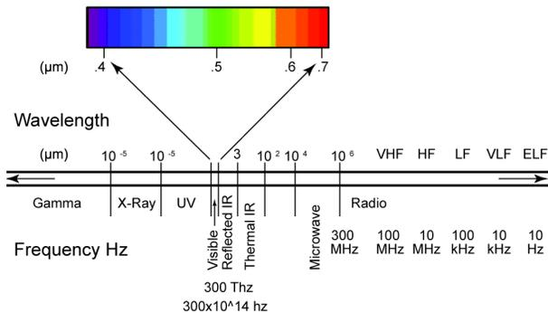
**Figure 3:** Electromagnetic Spectrum showing visible light range in relationship to more usual low frequency prospecting frequencies
