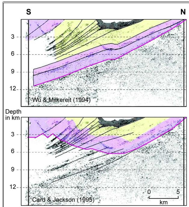
Figure 26: 2D Lithoprobe Seismic Reflection line across the Sudbury Basin showing two possible interpretations at depth.
