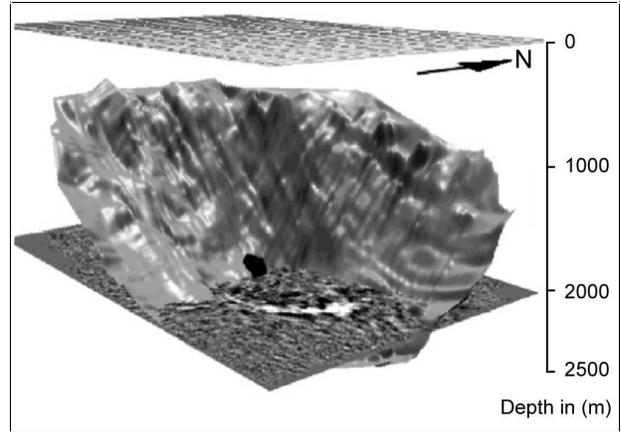
**Figure 29:** Trillabelle 3D Reflection Seismic survey highlights showing the base of the SIC as interpreted from the 3D survey, the known massive to semi massive mineralization (small black blob at 1800m depth) and a time slice through the data cube at 612 msec. showing the expanding reflection (white semicircle) from the mineralization (from Milkereit et al., 2000)
