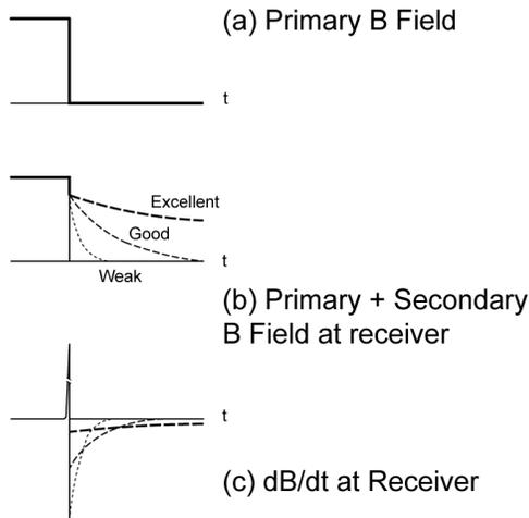
**Figure 34:** Schematic of an “off time” TEM system transmitted and received waveforms showing a) Primary B field from transmitter b) Primary plus secondary B field at receiver showing responses from weak, good, and excellent conductors c) dB/dt response at receiver for weak, good, and excellent conductors (after West et al 1991)
