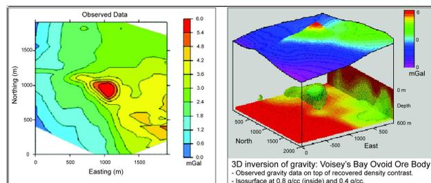
Figure 21: Local Bouguer ground gravity response of the Ovoid deposit (left) and constrained 3D gravity inversion using the UBC inversion codes (right) (from UBC-GIF website and Ash et al., 2006).
