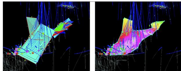
**Figure 30:** BHEM interpretation of multiple complex bodies: Left - current plate based iterative forward modeling and parametric inversion Right - new and future tools - automated iteration of surface facets on multiple curved sheets or solid bodies.
