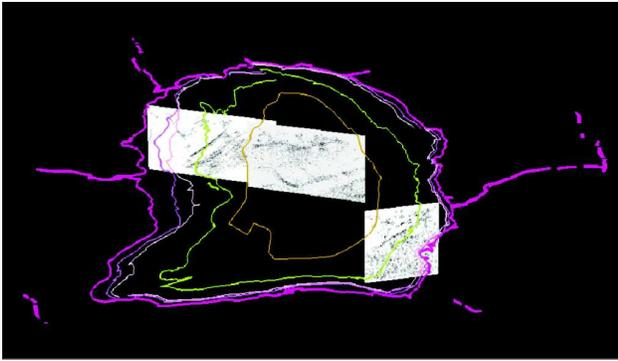
**Figure 27:** Simplified view of Sudbury 3D Model showing several of the Lithoprobe 2D seismic lines and surface traces of the main geological units.
