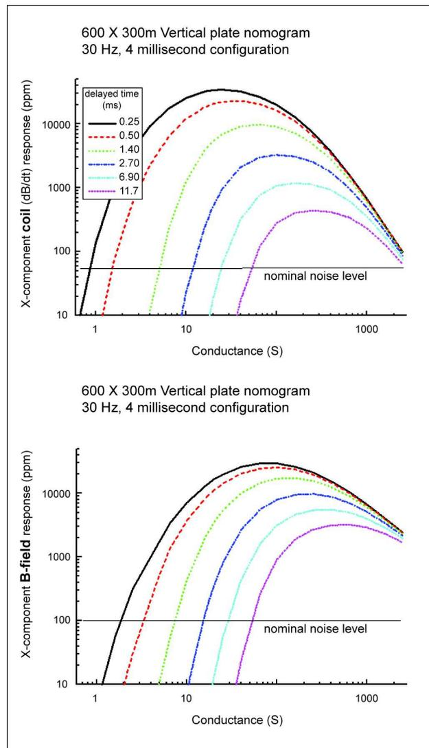
**Figure 36:** Left dB/dt versus Right B field calculated responses for a vertical 600m, by 300m plate for Fugro GEOTEM System (from Smith et al, 1998).
