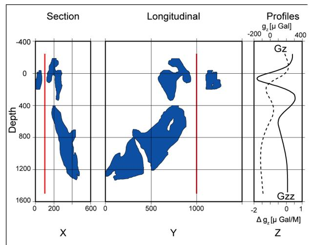
**Figure 39:** Borehole Gravity - Calculated responses  $G_z$  –dashed line and  $G_{zz}$  – solid line to known massive Ni-Cu-S orebodies (blue) at Kelly Lake, Sudbury from drillhole (red line) (After Nind et al., 2007)
