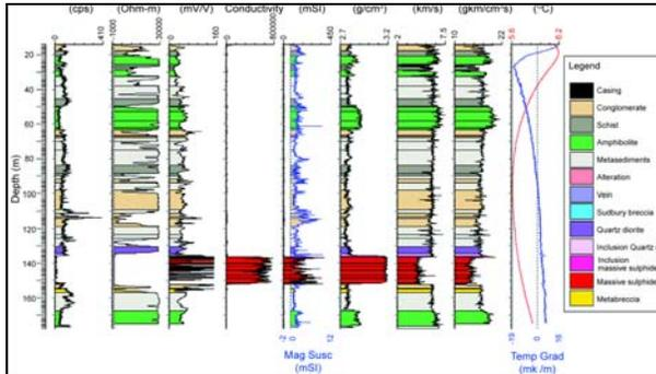
Figure 1: Physical Property Logs - McConnell Deposit BH 78930-0 (from Killeen et al., 1995)
