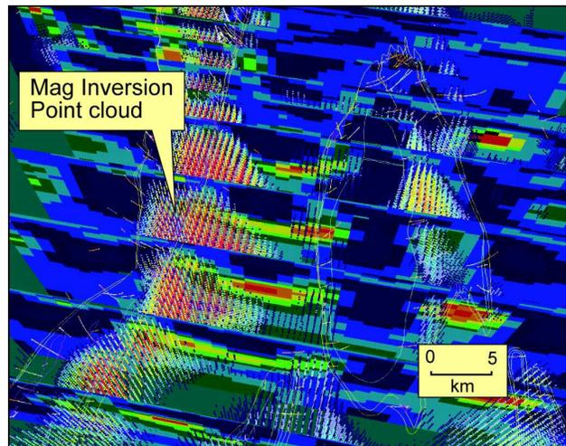
**Figure 10:** Thompson Nickel belt - AMT 2D stacked Vertical Sections and 3D magnetic inversions shown as point clouds (after Dowsett 1970).
