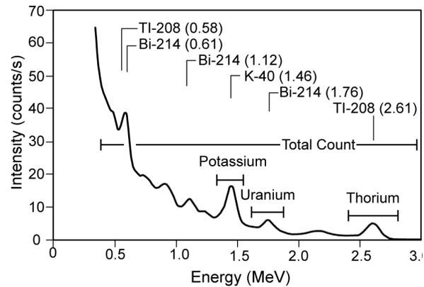
**Figure 6: Natural Gamma Spectrum**
