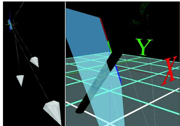
**Figure 5:** Oriented Virtual Core projected onto drill holewalls in 3D visualization software showing a fold in virtual core and interpreted fold axis surface.
