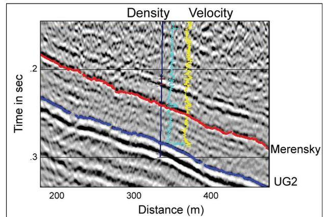
**Figure 40:** 3D Reflection Seismic Bushveld Complex – Vertical Section through 3D data volume showing reflections from the Merensky and UG2 horizons and Density and Velocity logs (from Larroque et al, 2002).
