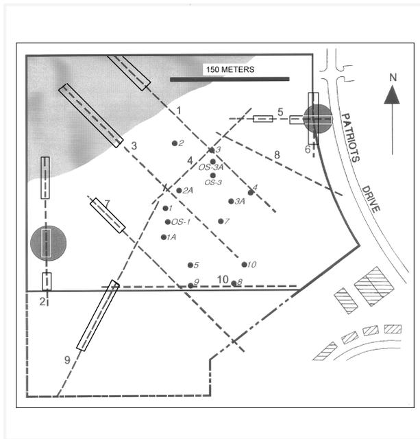
**Figure 1:** Map of the SAB study area (after Smith, 1958). Areas denoted on old (1958 vintage) regional mine location maps as mined-out have been highlighted. The locations of the reflection seismic lines, the test boreholes, areas of recent surface subsidence, and areas interpreted as mined-out are also shown.
