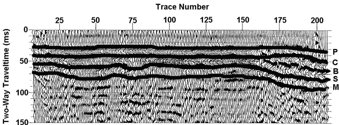
Figure 4: Interpreted version of reflection seismic line 1.
